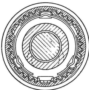
Cross section B-B Cone synchronizer
