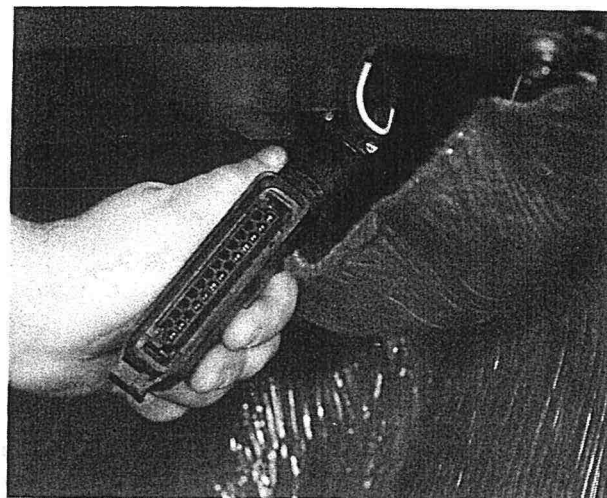
Multiple connector connecting injection system to control unit
