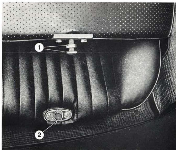
Fig. 511 - Detail showing seat squab adjusting device.
