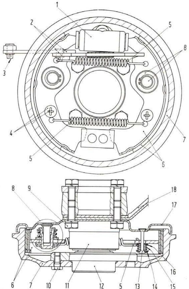
Fig. 294 - Right rear wheel sectional views (from car with No. for spare 802093).
