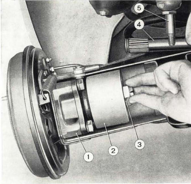
Fig. 258 - Loosening wheel shaft flexible joint mounting nut.
