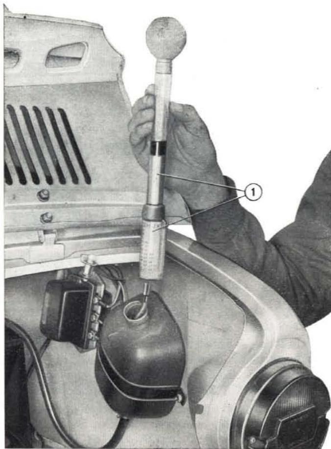
Fig. 131 - Checking rate of « Paraflu 11 » fluid in cooling system.
