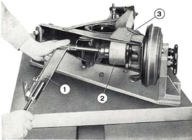
Fig. 254 - Installing wheel shaft flexible joint on work bench.
