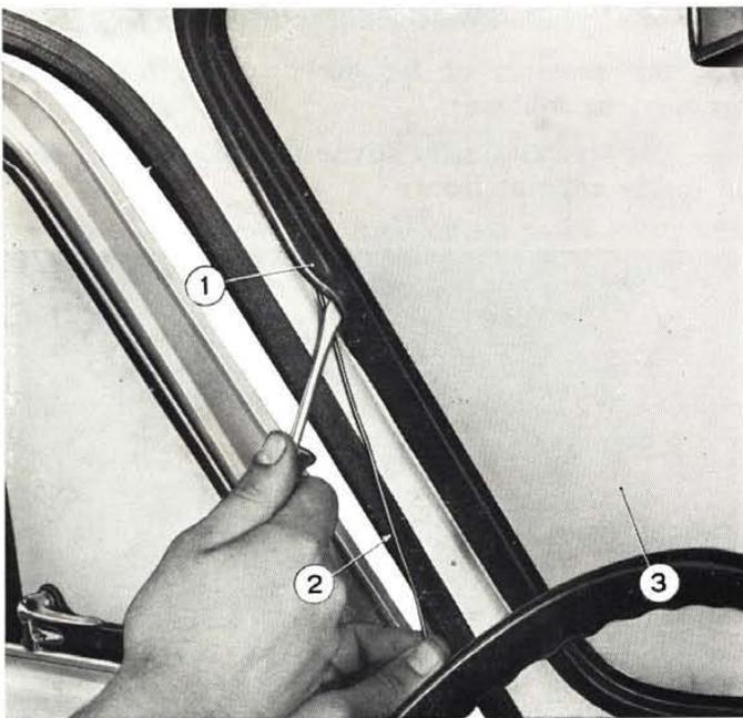
Fig. 404 - Installing windshield glass.
