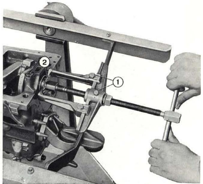
Fig. 14 - Pulling timing drive sprocket.
