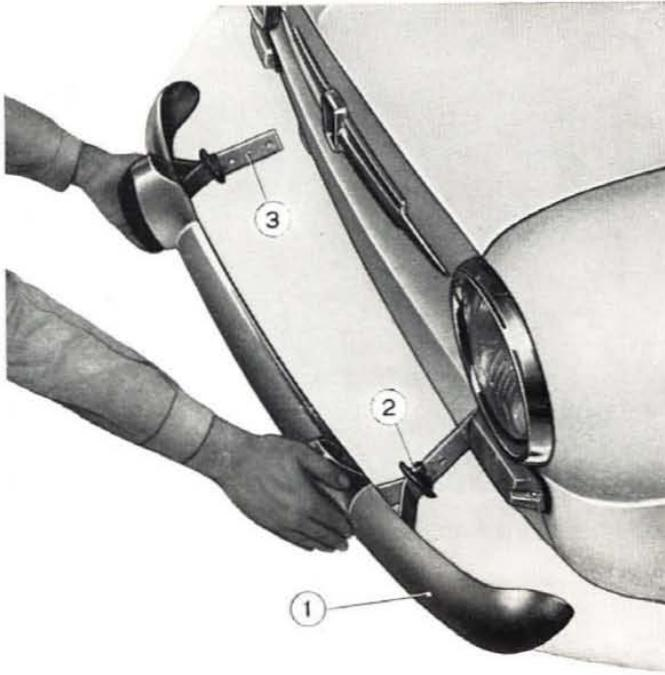
Fig. 407 - Removing front bumper.
