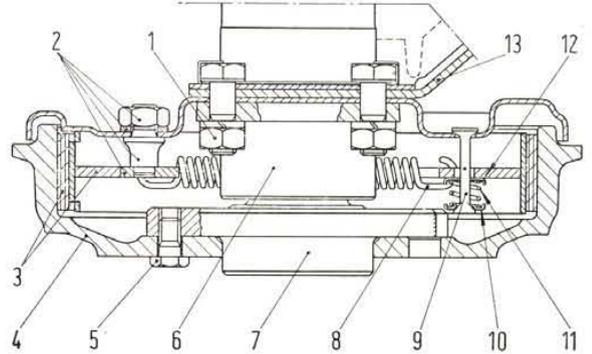
Fig. 291 - Sectional view of right side rear wheel. (Up to car with No. for spare 802091).
