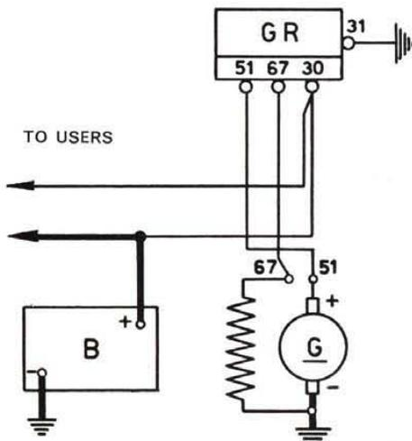
Fig. 333 - Wiring diagram of regulator assembly GN 2/12/16.
