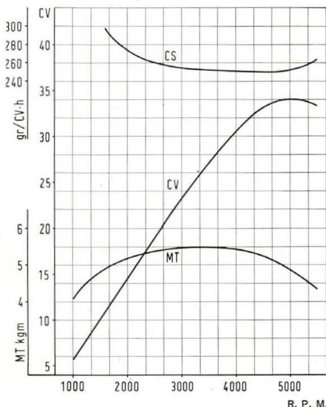
Fig. 122 - Horsepower, consumption and torque curves of 100G.000 engine.
