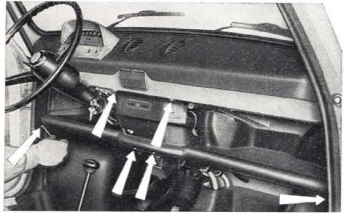
Fig. 305 - Removing utility shelf. Arrows point to shelf mounting screws.
