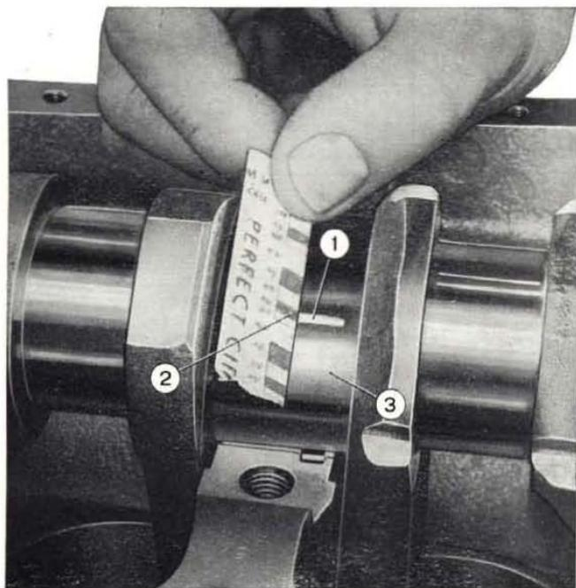
Fig. 77 - Comparing the width of flattened « Plastigage » with the graduations on the envelope.
