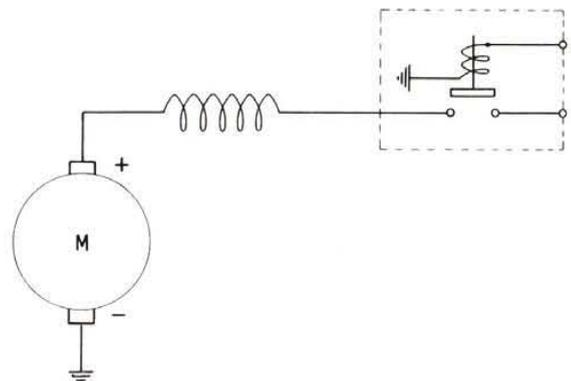
Fig. 346 - Starting motor wiring diagram.
