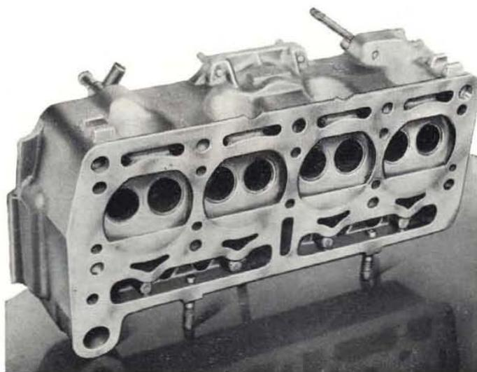
Fig. 88 - Checking cylinder head on surface plate.
