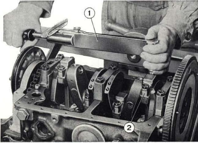
**Fig. 63 - Securing connecting rod bearing caps.**
