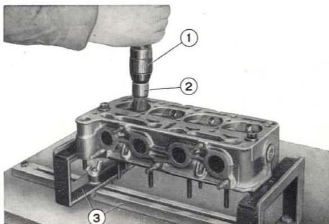
**Fig. 87 - Decoking and cleaning combustion chambers.**
