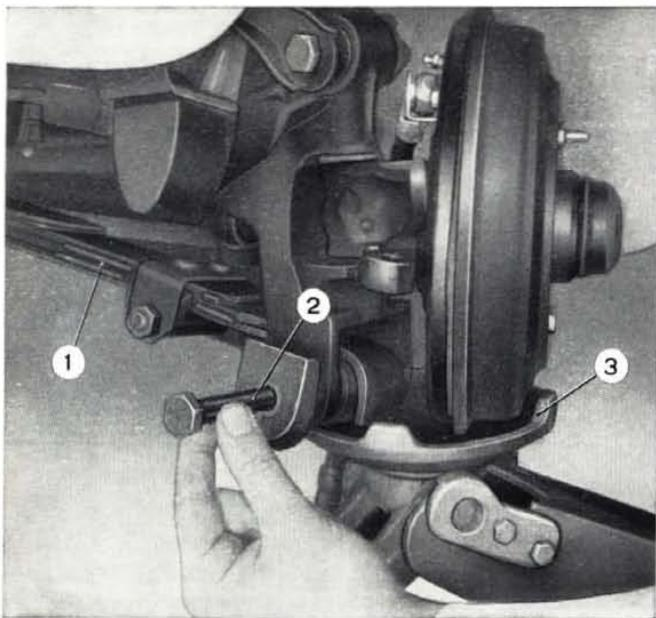
**Fig. 211 - Removing semi-elliptic spring pin.**
