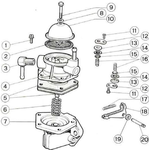
**Fig. 139 - Layout of fuel pump components.**
