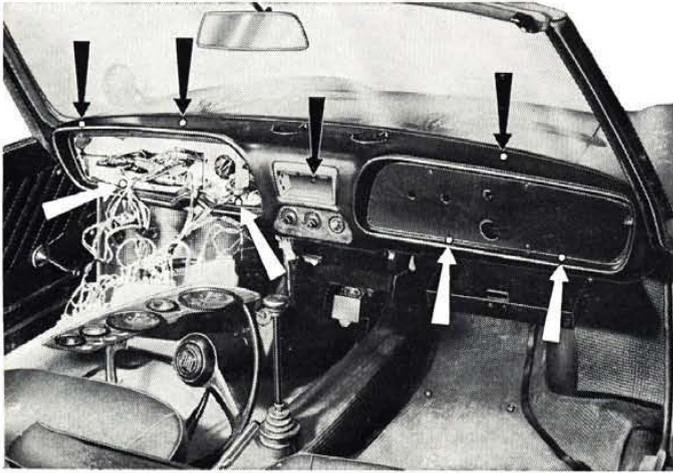
Fig. 512 - Layout of instrument panel lining holding points. Arrows evidence location of lining holding screws, nuts and lugs.
