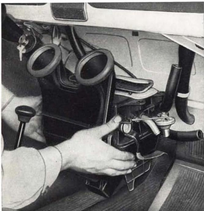
**Fig. 308 - Withdrawing air conditioner.**
