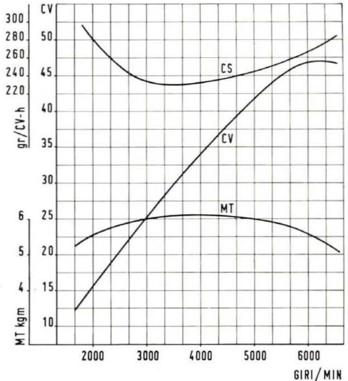
Fig. 438 - Horsepower, consumption and torque curves of 100 GC.000 engine.
