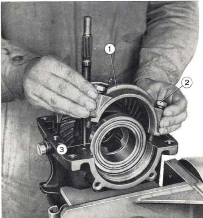
Fig. 188 - Removing differential carrier caps.
