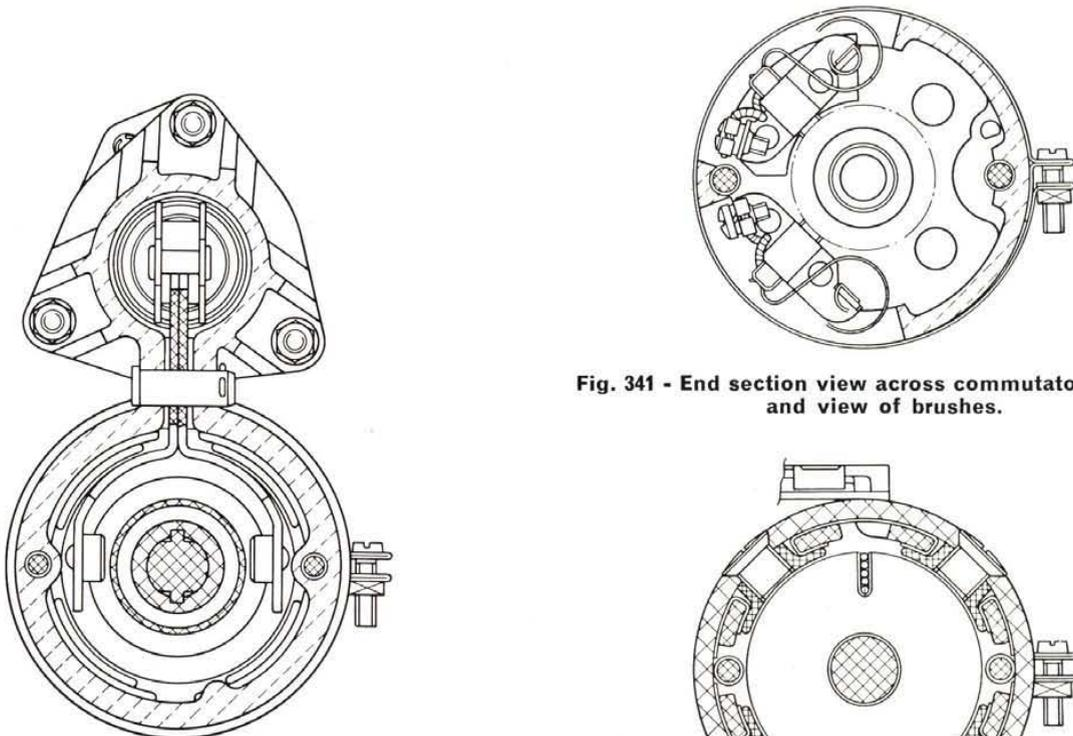
Fig. 340 - End section view of starting motor across pinion drive.
