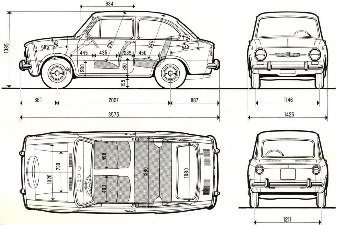
Fig. 2 - Leading dimensions of car (metric).
