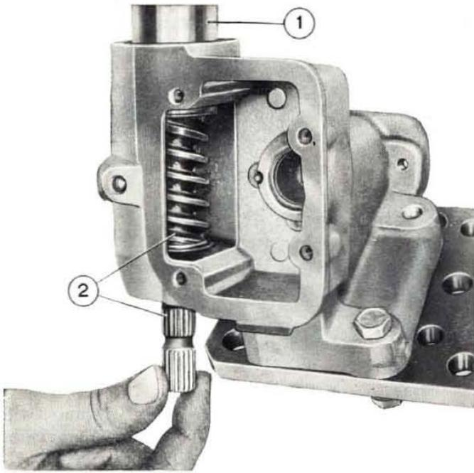
Fig. 277 - Adjusting worm bearings.
