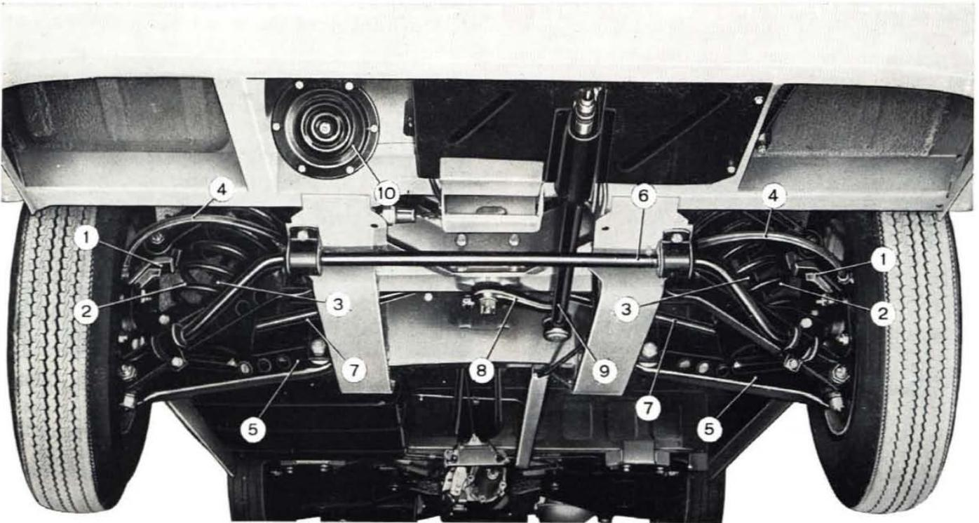
**Fig. 523 - Bottom view of front suspension in place on car.**
