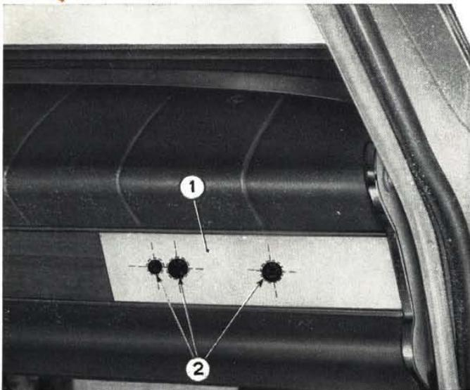
**Fig. 465 - Fitting templet to drill radio receiver mounting holes.**
