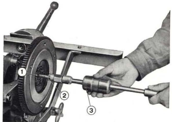
Fig. 82 - Pulling clutch shaft pilot bushing.
