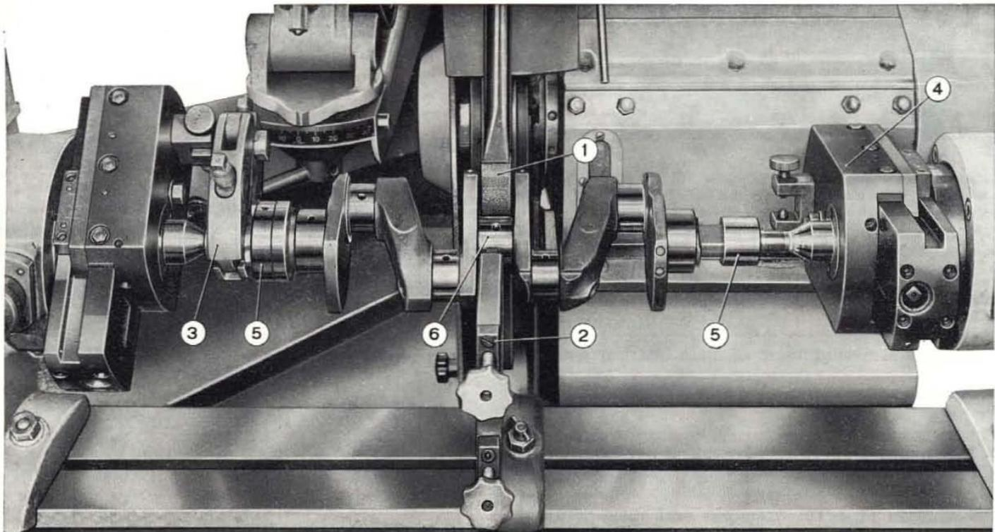
Fig. 65 - Grinding main bearing journals on grinding machine.
