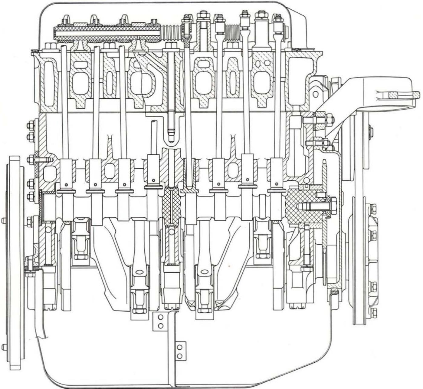
Fig. 83 - Side sectional view of engine across valve mechanism.
