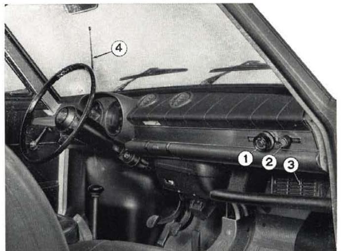
**Fig. 467 - Radio assembly installed on car.**
