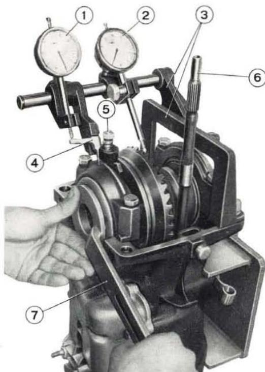
Fig. 197 - Setting differential cage bearing preload by means of fixture A. 95688.
