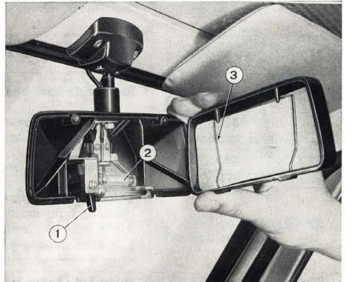
**Fig. 368 - Removing map light bulb.**
