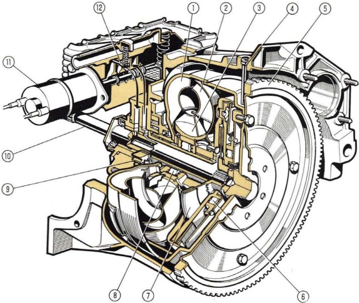
Fig. 560 - Sectional view of Idroconvert transmission.
