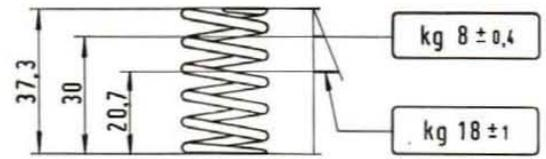
Fig. 427 - Inner valve spring specifications.
