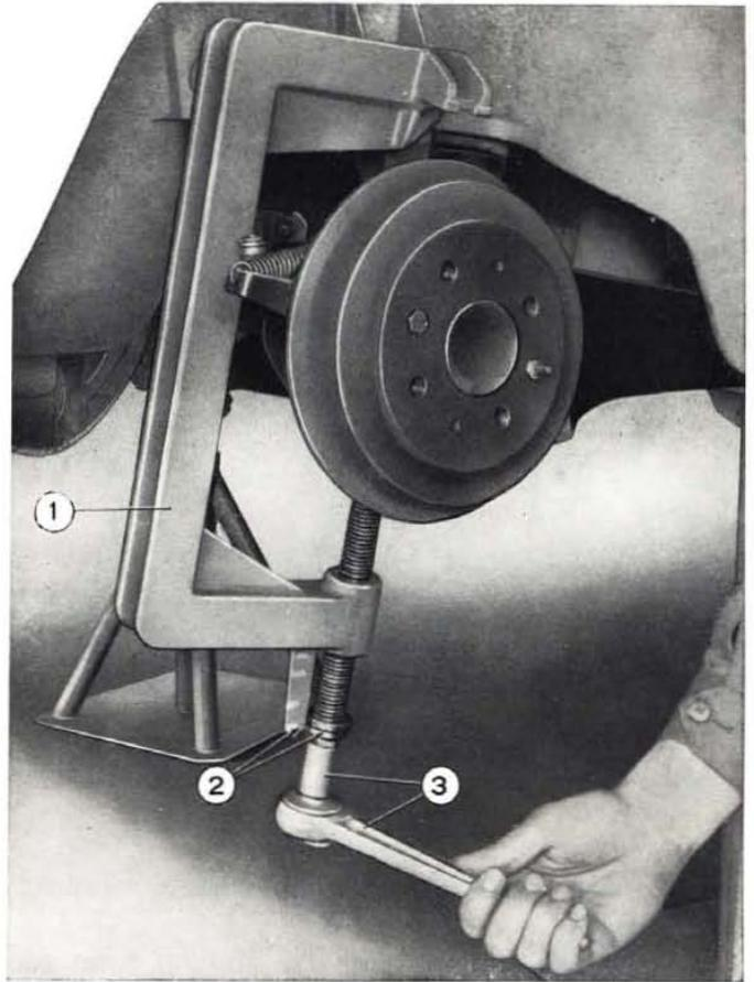
Fig. 264 - Installing coil spring compressor.
