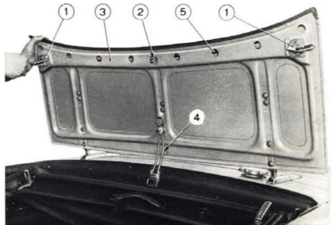
**Fig. 519 - Removing folded top recess lid latch link.**
