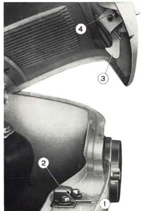
**Fig. 402 - Engine compartment lid catch.**
