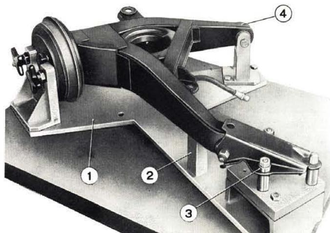
**Fig. 249 - Checking control arm and drum assembly.**
