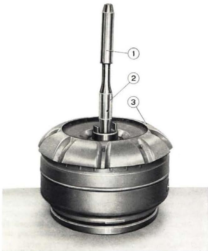
Fig. 590 - Torque converter assembly.
