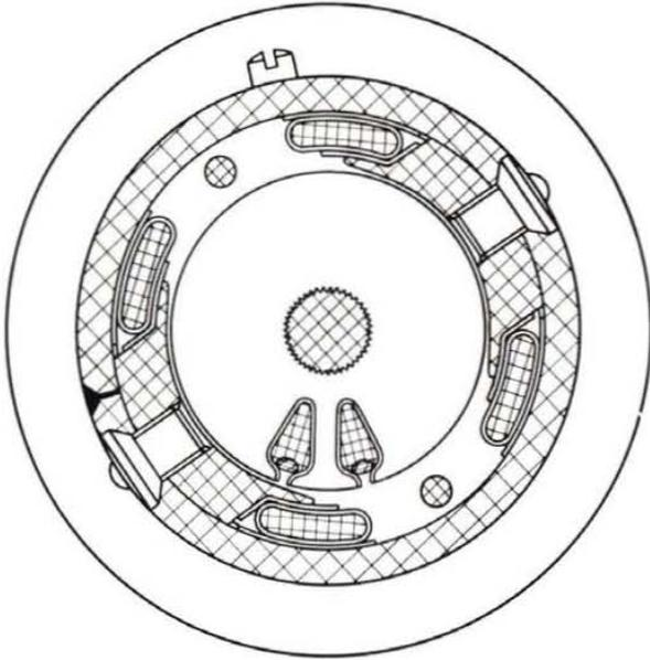
Fig. 316 - End sectional view of generator across field frame, pole shoes and windings.
