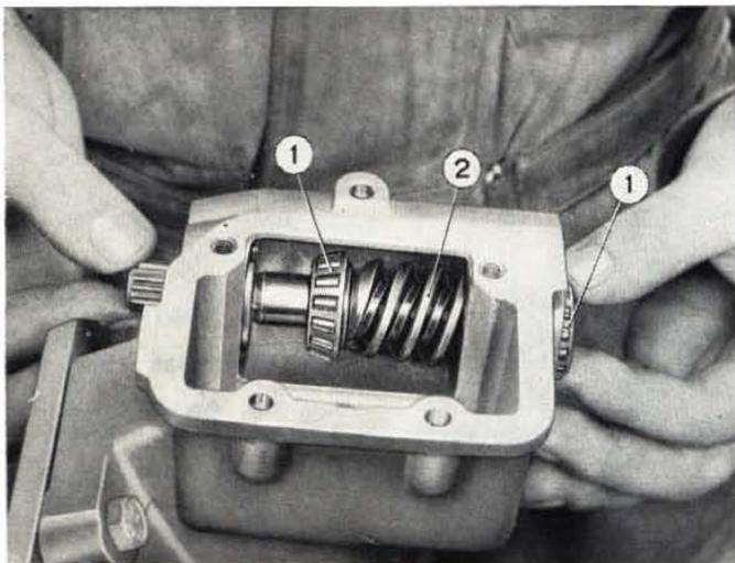
Fig. 282 - Installing steering worm and bearings.
