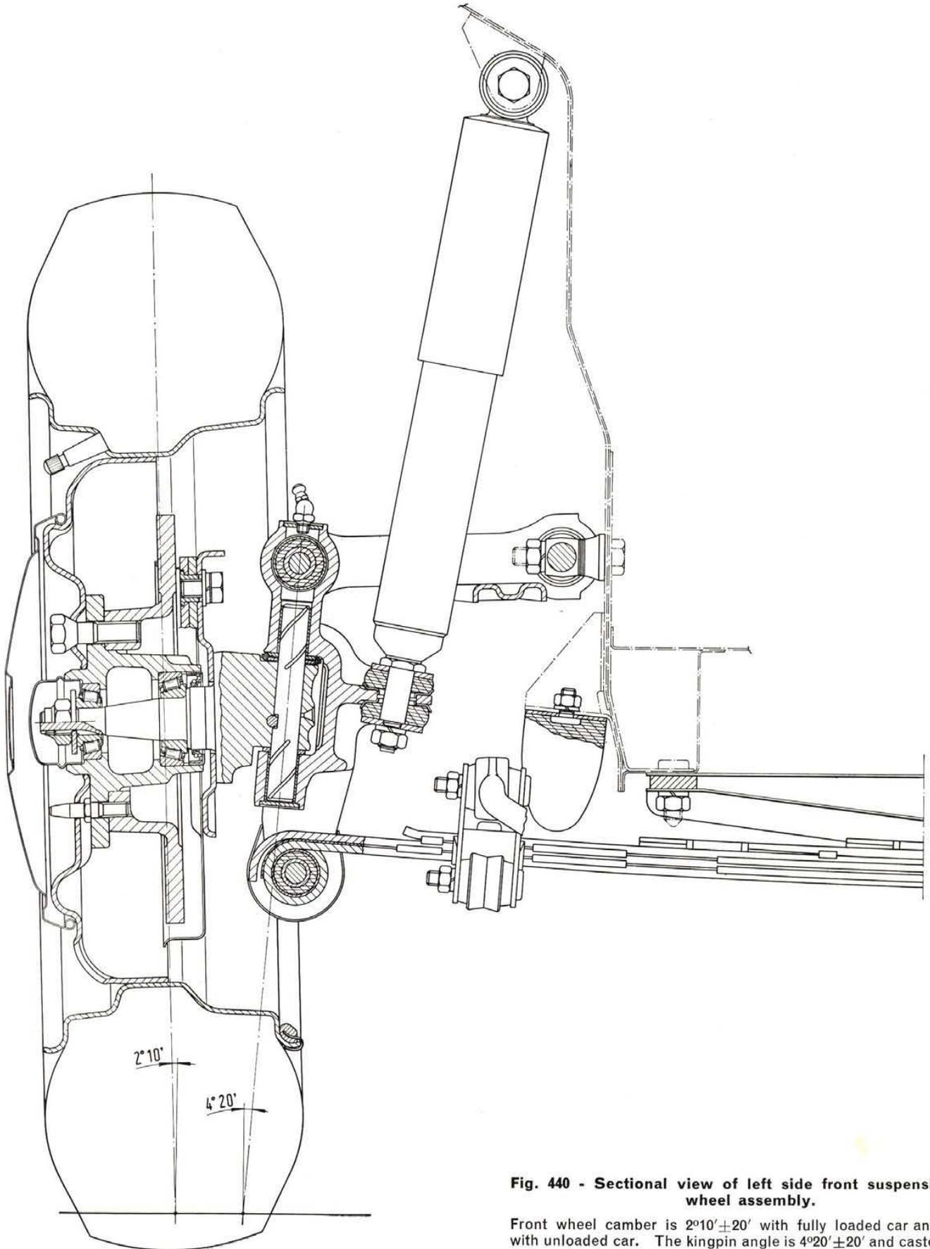
**Fig. 440 - Sectional view of left side front suspension and wheel assembly.**
