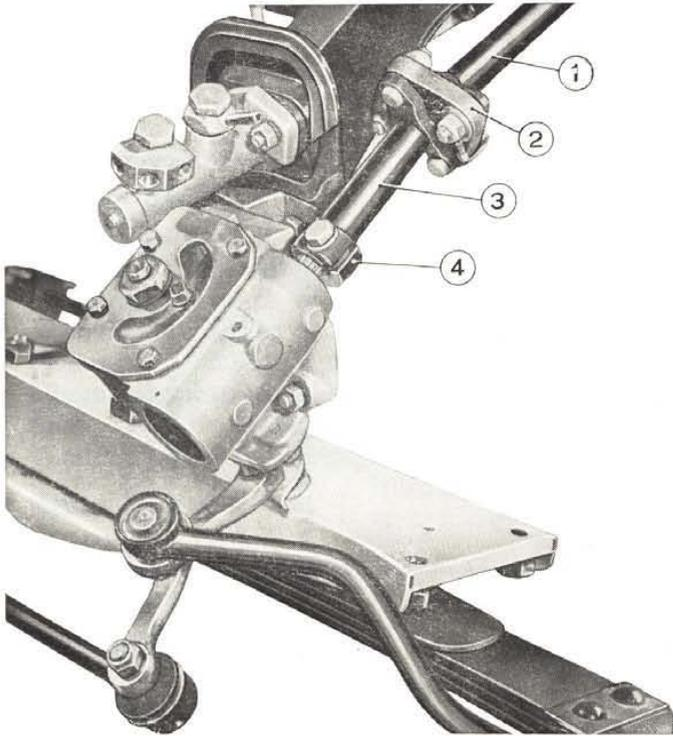
Fig. 444 - Scrap view of the steering system showing the column flexible joint.
