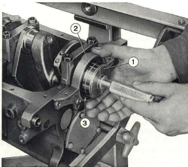
**Fig. 20 - Installing crankshaft front oil seal cover.**
