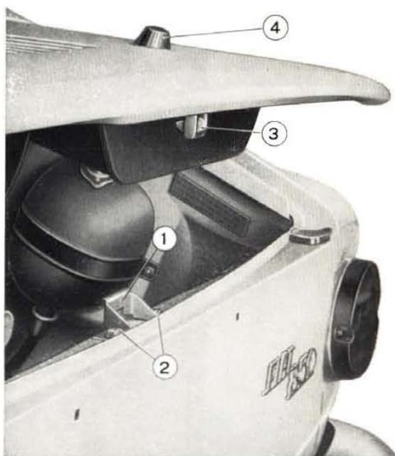
Fig. 479 - Detail of rear compartment lid catch.
