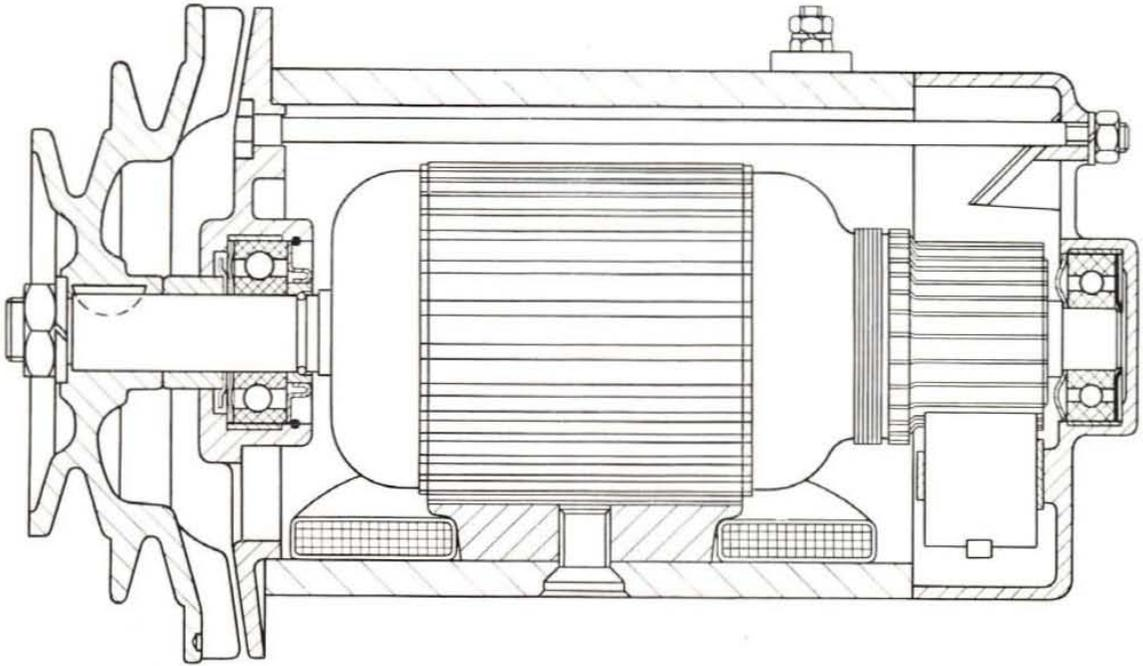
Fig. 549 - Side sectional view of generator.
