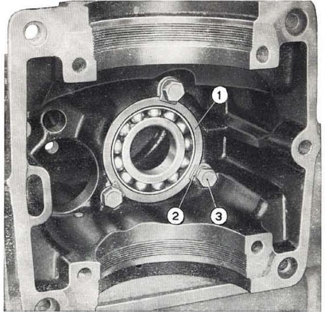
Fig. 192 - Drive pinion ball bearing.
