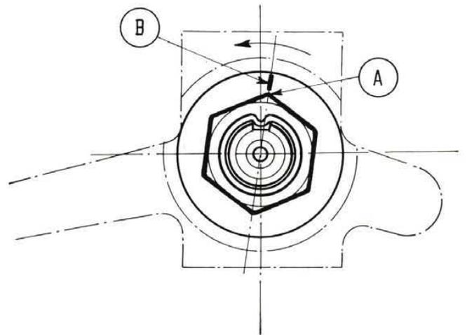
Backing out hub nut  $30^\circ$ .
