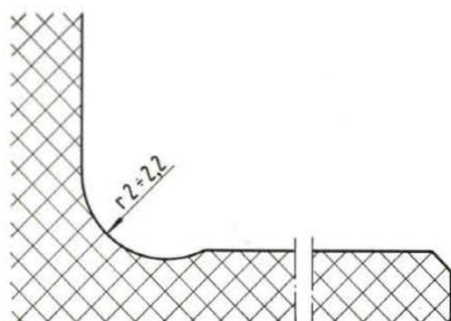
Fig. 66 - Fillet radii for chain end main bearing journal shoulder.
