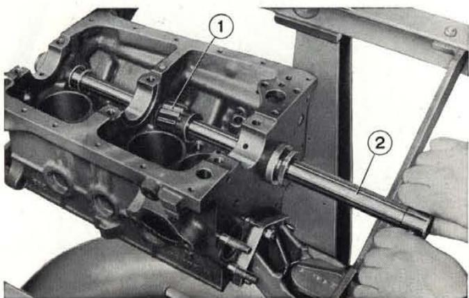
Fig. 17 - Reaming intermediate camshaft bushing.
