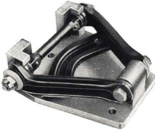
Fig. 218 - Control arm installed on fixture A. 74135.
