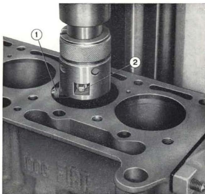
Fig. 31 - Aligning cylinder bore, preparatory to boring operation.
