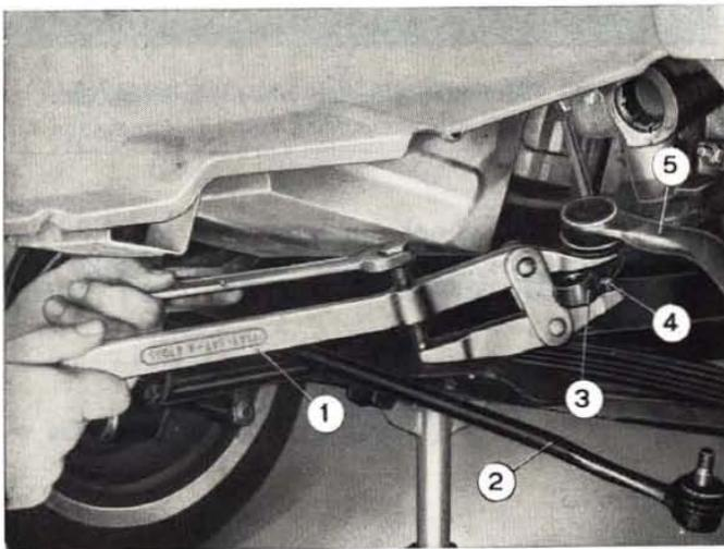
**Fig. 274 - Removing steering rods.**
