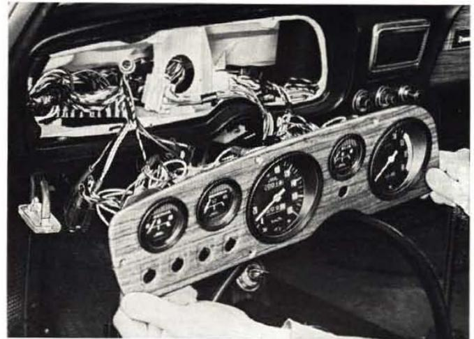
Fig. 507 - Removing instrument assembly from dashboard.
