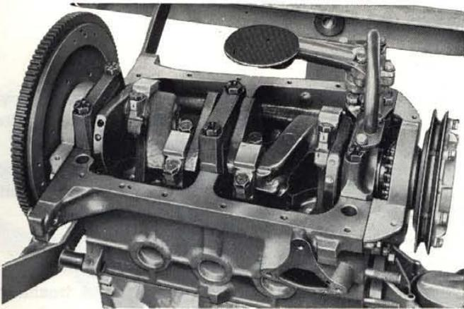
Fig. 12 - Crankcase without oil sump.
