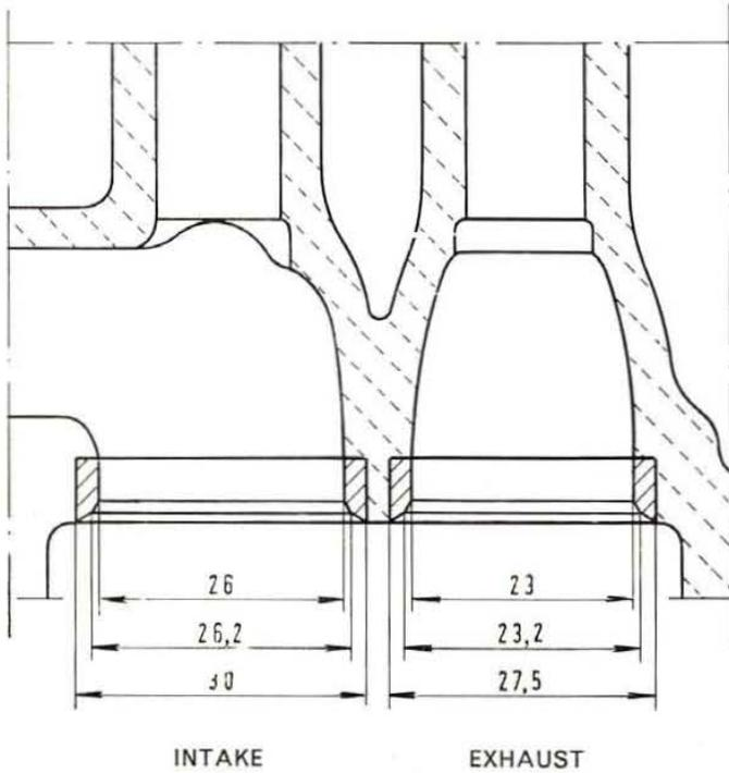
Fig. 428 - Diameters of intake and exhaust valve seats in head.
