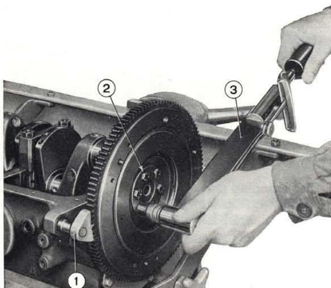
Fig. 72 - Tightening flywheel mounting nuts.
