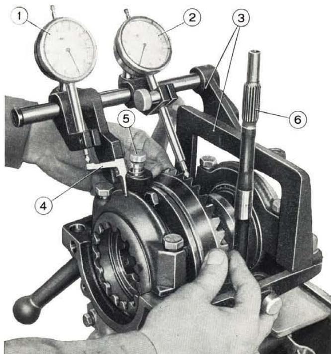
Fig. 199 - Checking ring gear-to-pinion backlash.
