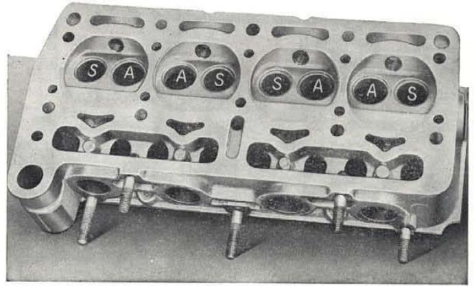
Fig. 99 - View of valve seats in head.
