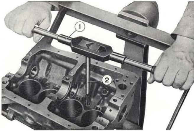
Fig. 38 - Reaming tappet seats on crankcase.
