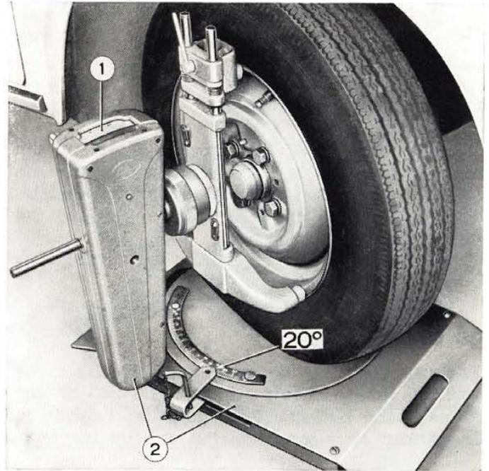
Fig. 236 - Checking caster (first step).
