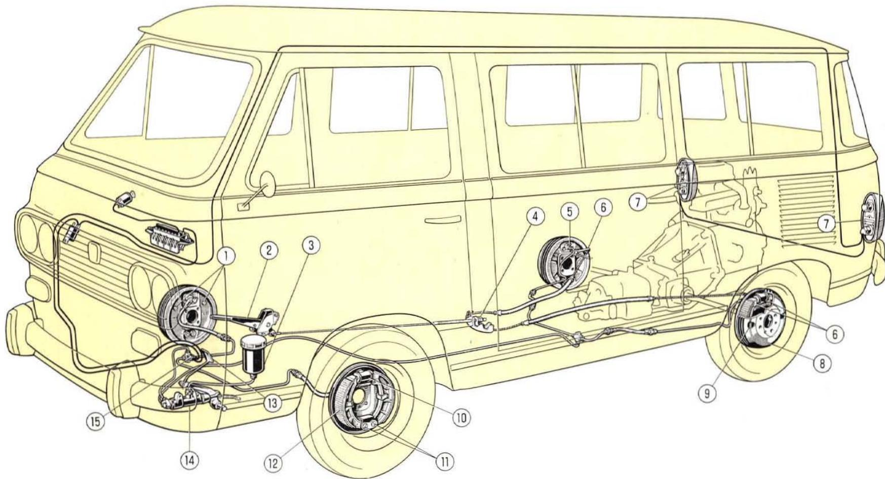
**Fig. 540 - Diagram of hydraulic service brakes and emergency and parking brake.**
