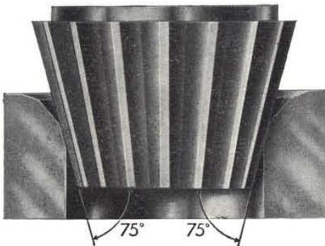
Fig. 97 - Narrowing valve seat at bottom with 75° cutter.
