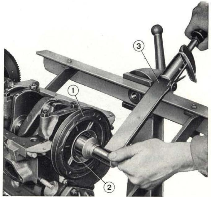
**Fig. 21 - Tightening hub-pulley nut.**
