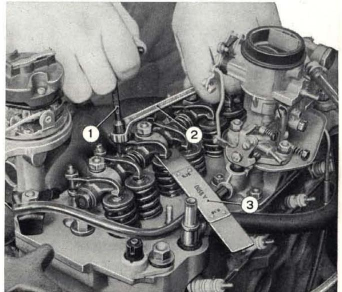
Fig. 119 - Adjusting valve tappet clearance.
