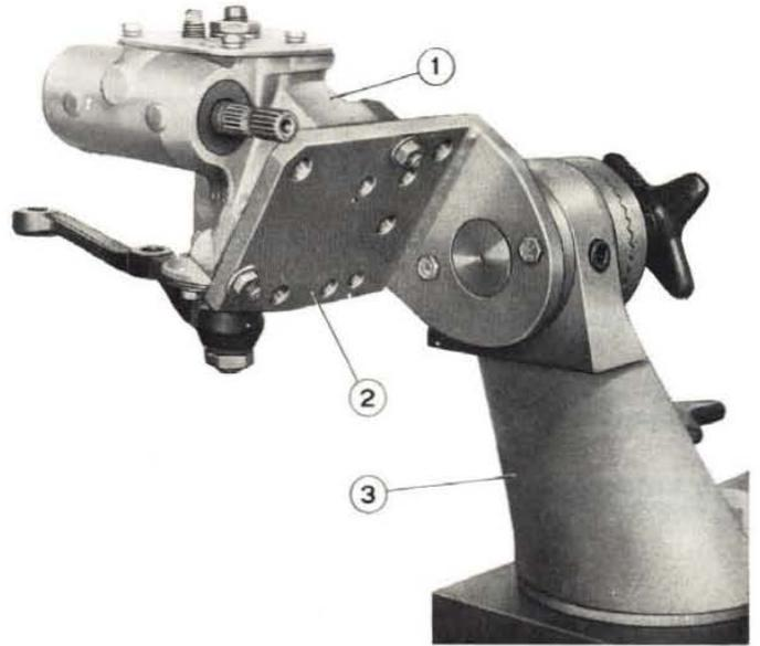
**Fig. 275 - Steering gear on service fixture.**
