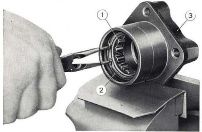
**Fig. 252 - Installing roller bearing snap ring.**
