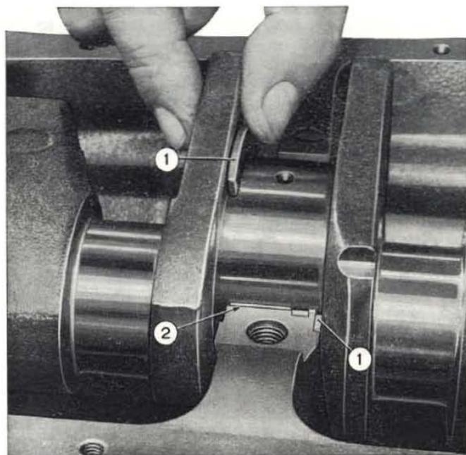
Fig. 78 - Fitting thrust ring halves.
