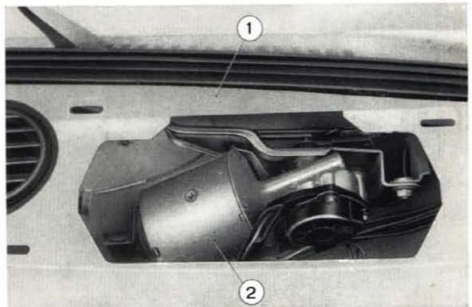
Fig. 375 - Arrangement of windshield wiper.
