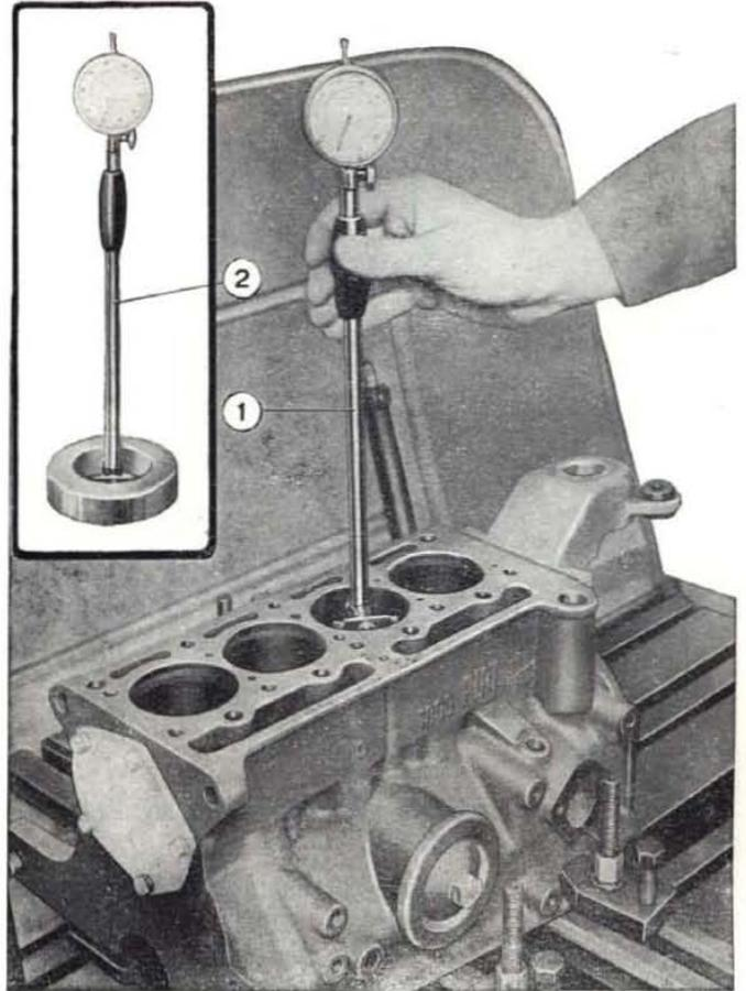
Fig. 28 - Using dial indicator to measure cylinder bores.
