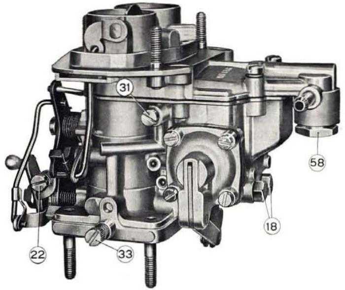
**Fig. 435 - Carburetor viewed from the volume control screw end.**
