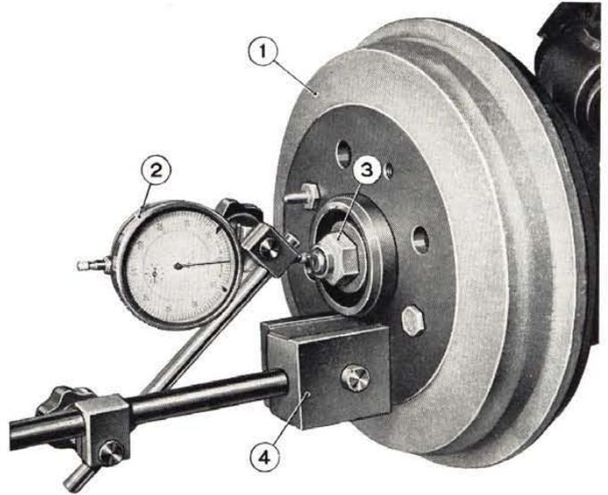
Fig. 239 - Using dial indicator with magnetic base to check wheel hub end play.
