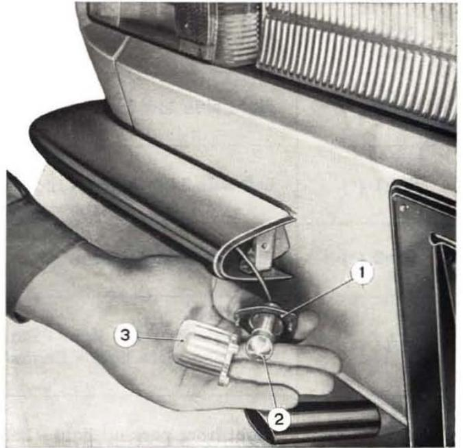
Fig. 499 - License plate lamp components.
