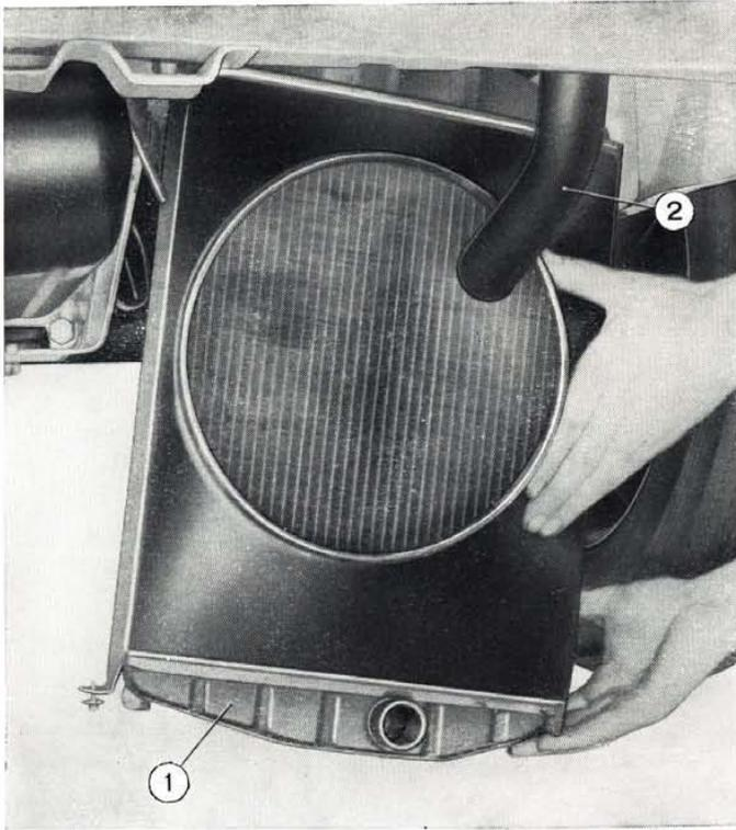
**Fig. 133 - Lifting out radiator from underside of car.**
