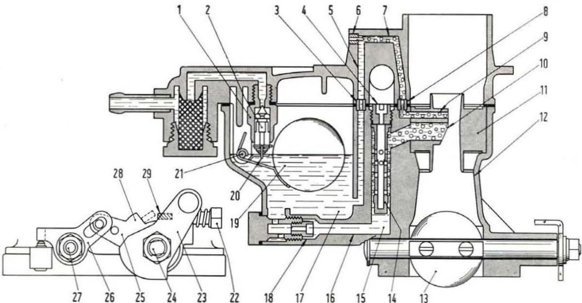
Fig. 431 - Diagrammatic section views of Weber 30 DIC 1 carburetor.
