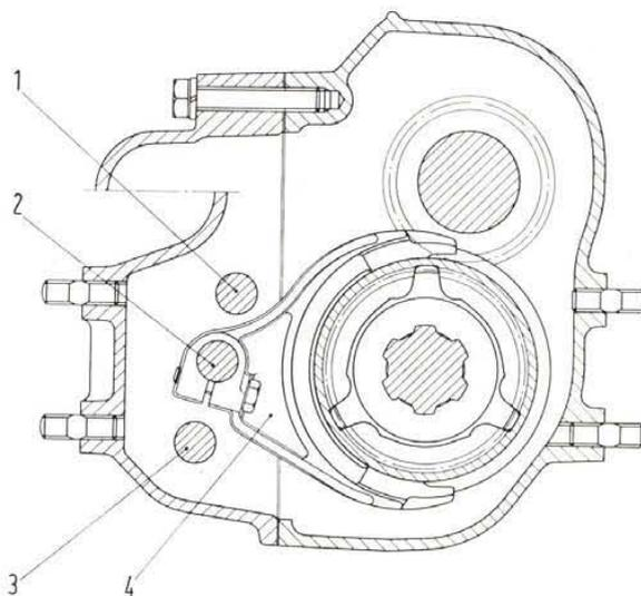
Fig. 181 - End sectional view of transmission across shifter rails.
