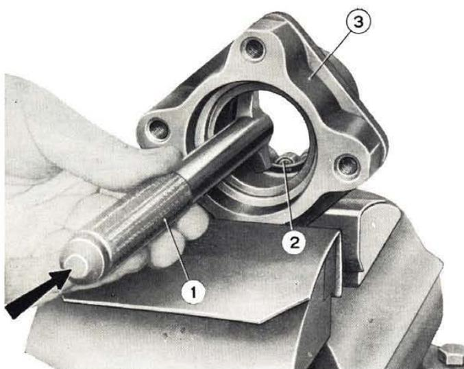
**Fig. 247 - Removing roller bearing cup.**
