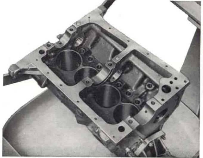
Fig. 36 - Bottom view of crankcase.
