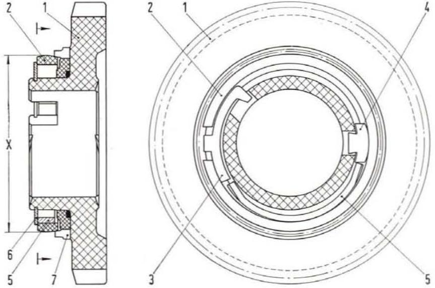
When sleeve and gear teeth are in full mesh, the synchro ring settles down inside the slip sleeve, which makes for the solid engagement of the gear attached.
