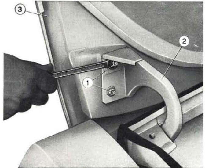
**Fig. 401 - Repositioning front compartment lid.**
