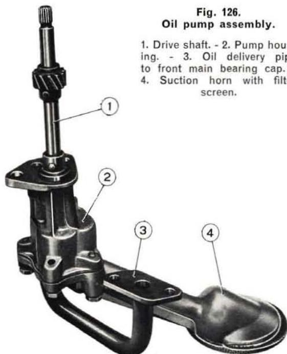
1. Drive shaft. - 2. Pump housing. - 3. Oil delivery pipe to front main bearing cap. - 4. Suction horn with filter screen.
