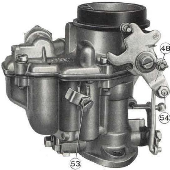
Fig. 144 - View of Weber carburetor from choke control lever end.
