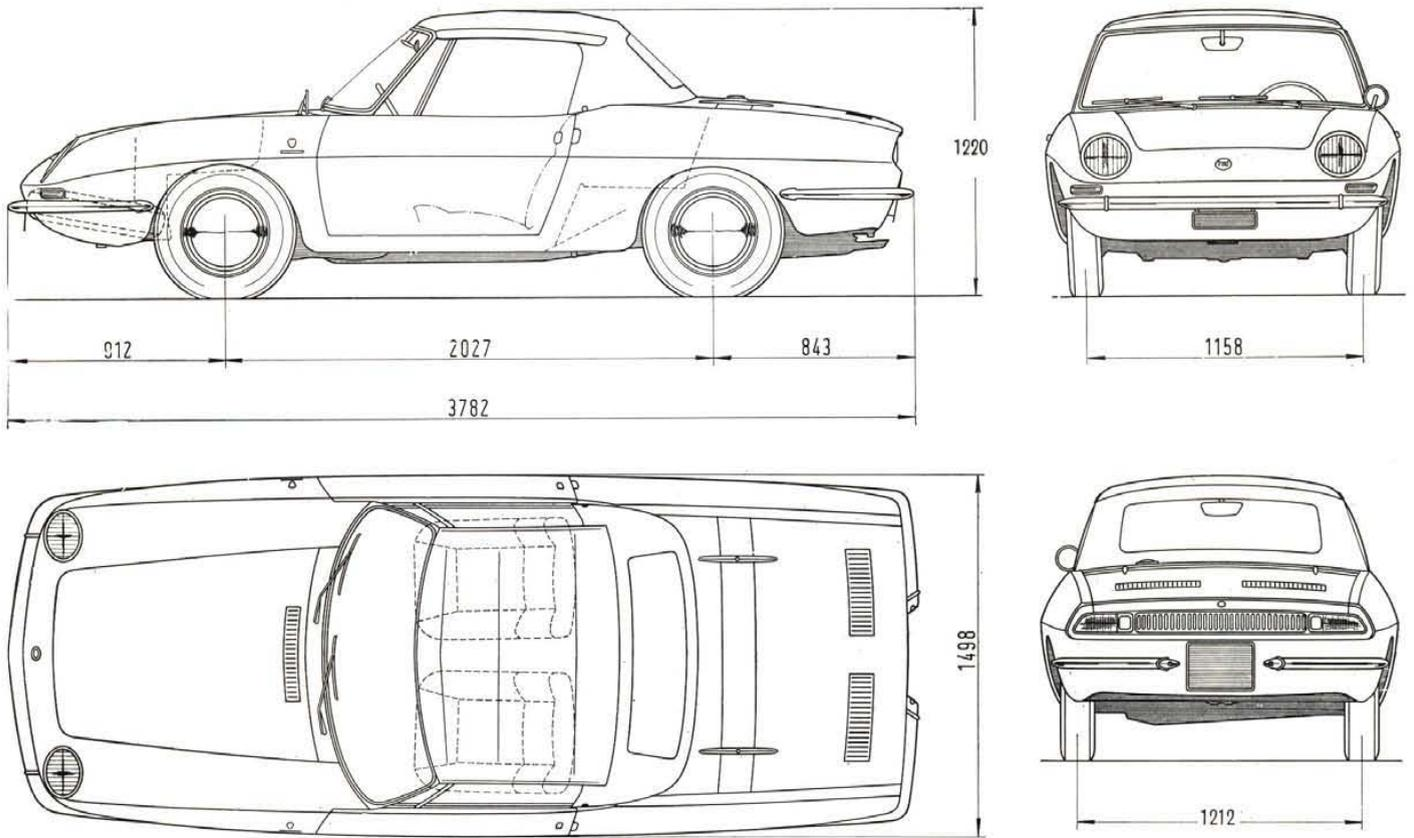
**Fig. 482 - Leading dimensions (metric).**
