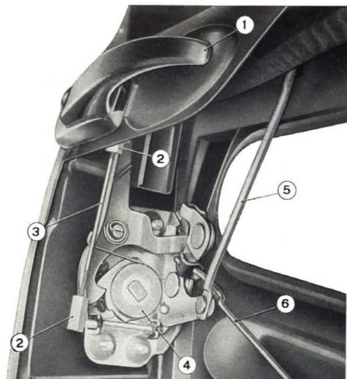
**Fig. 396 - Interior view of door latch.**
