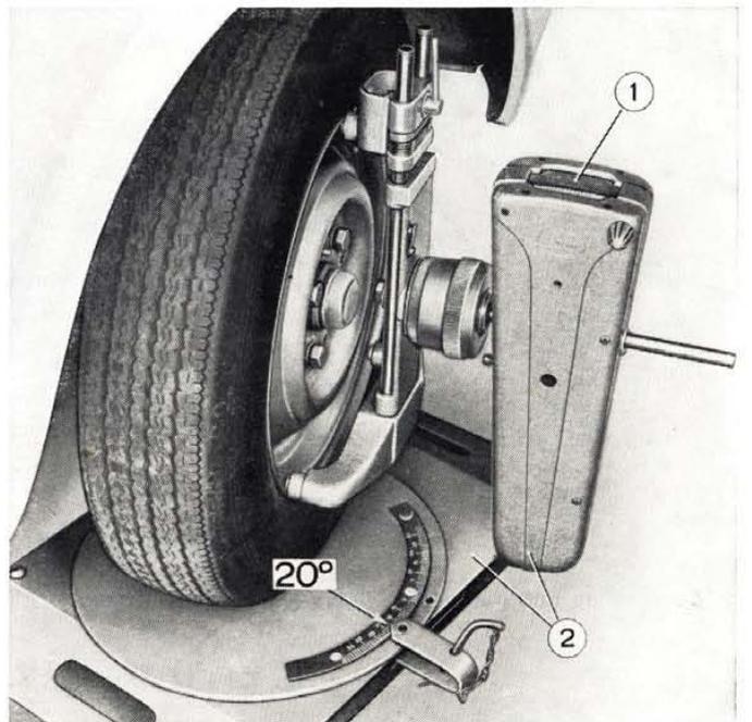
Fig. 237 - Checking caster (second step).
