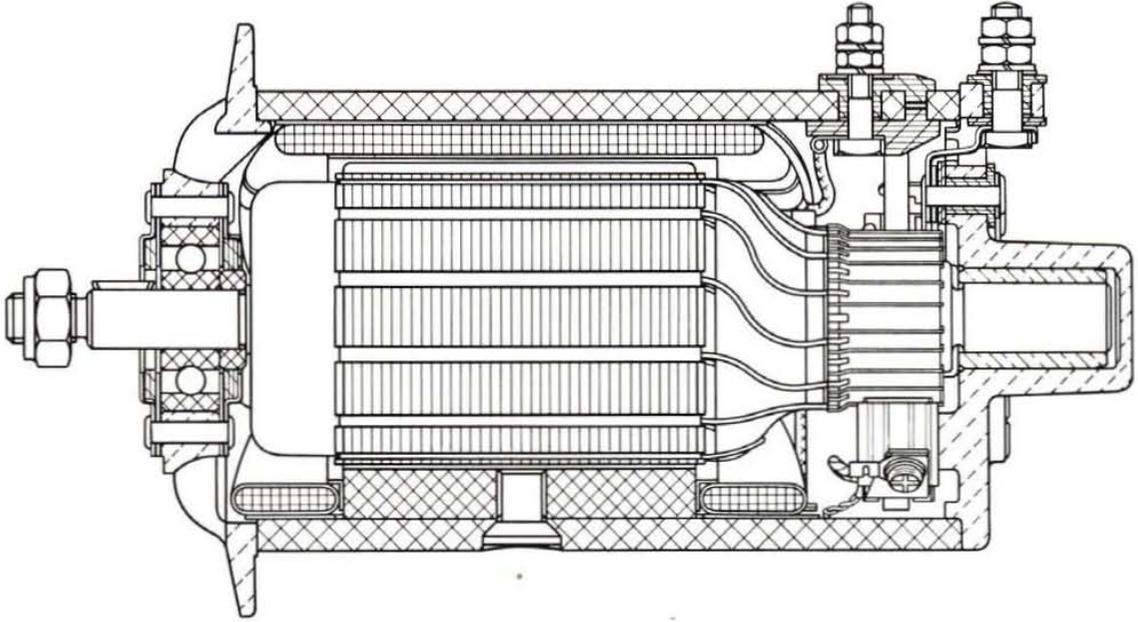
Fig. 315 - Side sectional view of generator.
