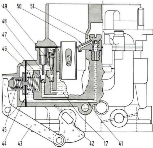
**Fig. 434 - Diagrammatic sections of Weber 30 DIC 1 carburetor.**
