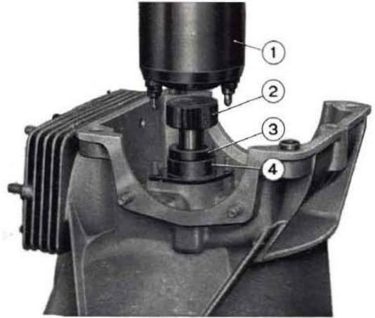
Fig. 577 - Fitting the seal on torque converter support.
