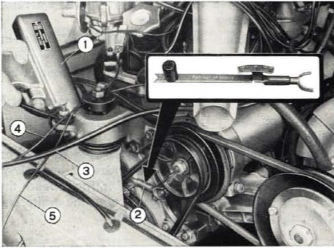
**Fig. 357 - Checking ignition timing.**
