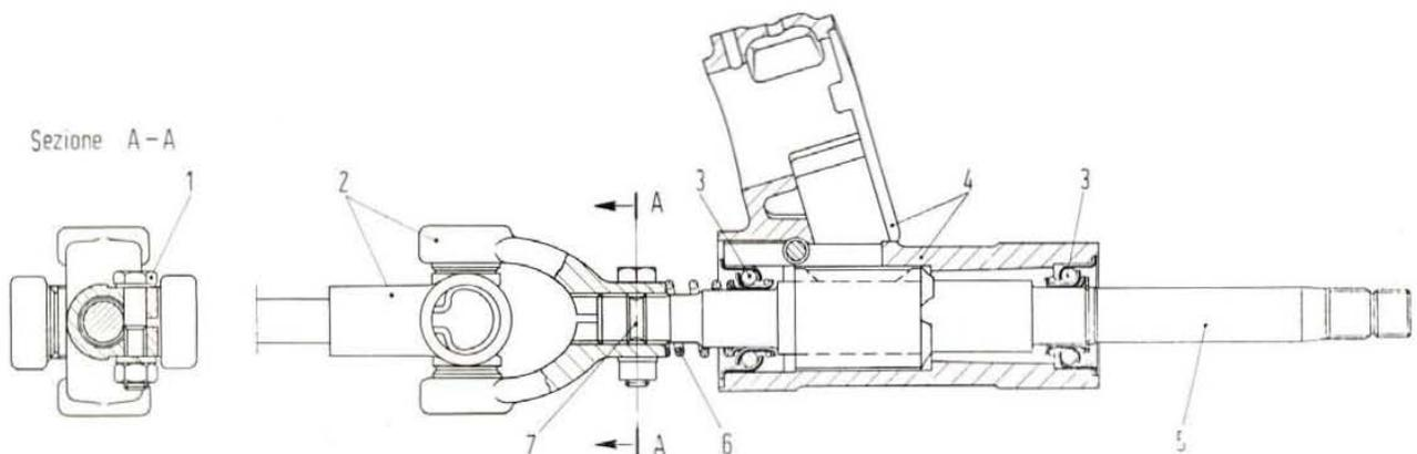
**Fig. 487 - Section view of the steering column and mounting bracket.**
