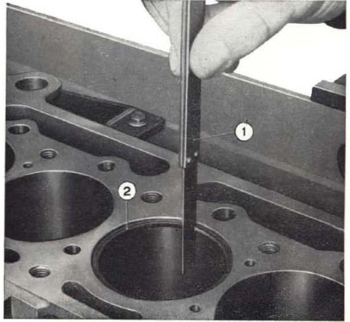
**Fig. 48 - Checking end gap of piston rings in cylinder.**
