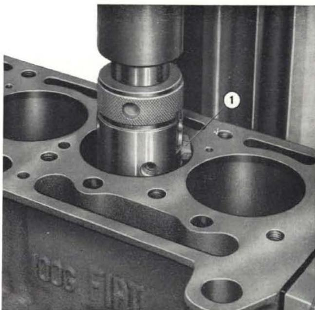
Fig. 33 - Reboring cylinders.
