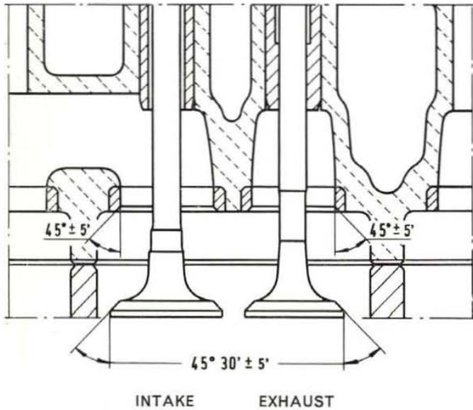
Fig. 91 - Inclination angles of valves and seats in head.
