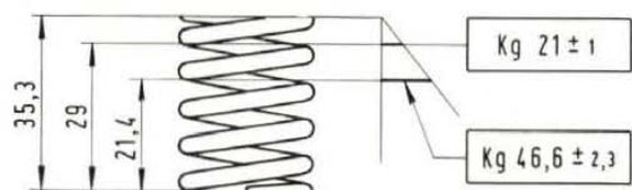
Fig. 106 - Valve spring specifications.
