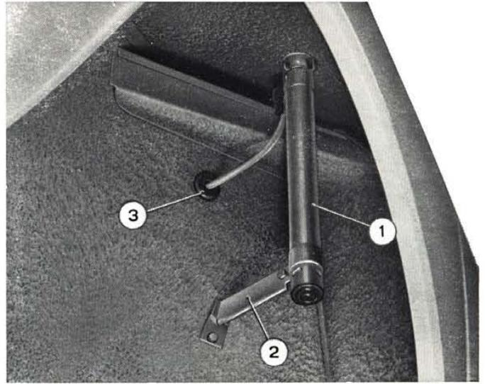
**Fig. 466 - Detail showing antenna mounting.**
