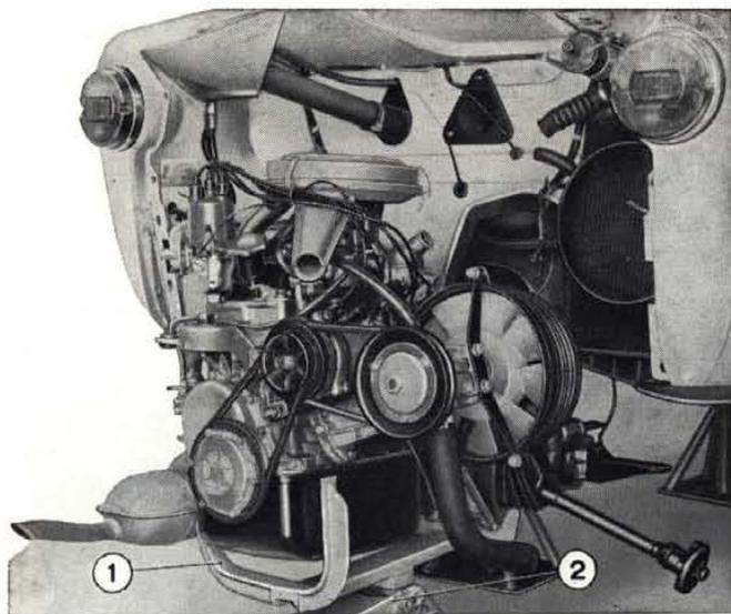
Fig. 10 - Removing engine and transmission assembly.
