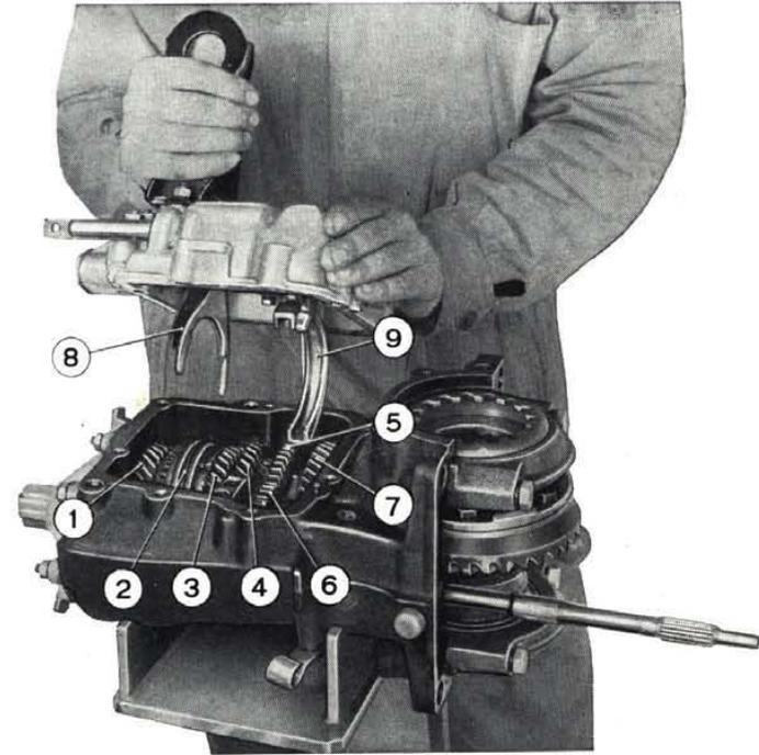
Fig. 172 - Removing side cover, complete with shifter rails and forks.
