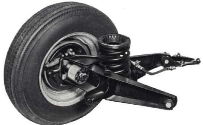
Fig. 257 - Left side rear suspension and wheel assembly.
