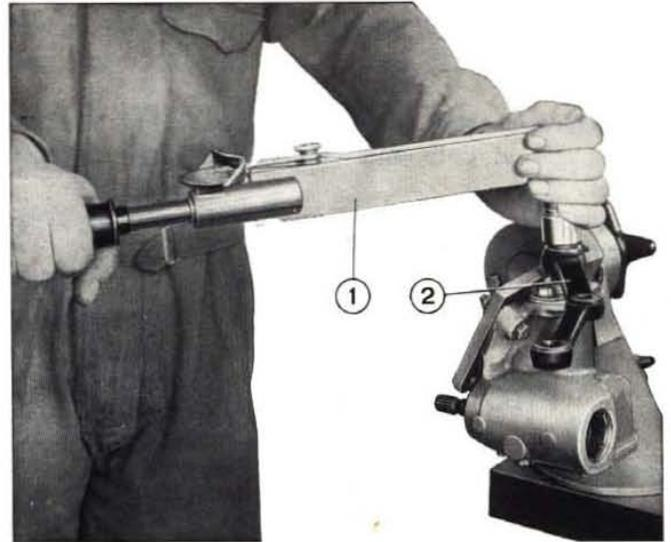
Fig. 283 - Installing pitman arm.
