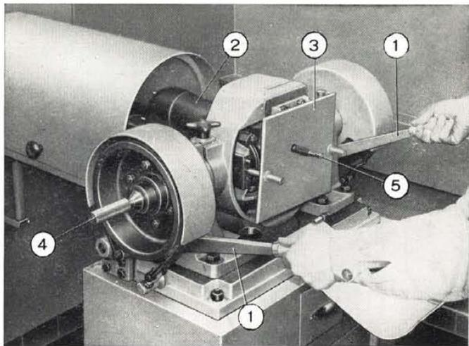
Fig. 200 - Bench testing differential unit.
