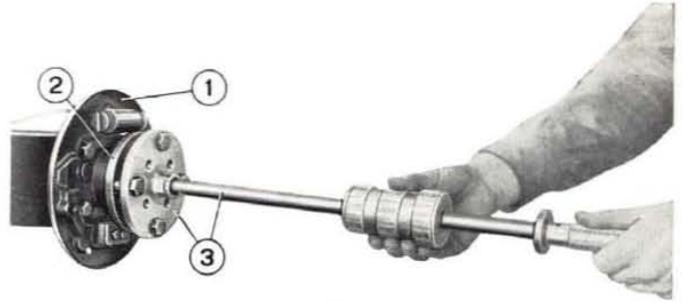
**Fig. 245 - Pulling rear wheel hub.**
