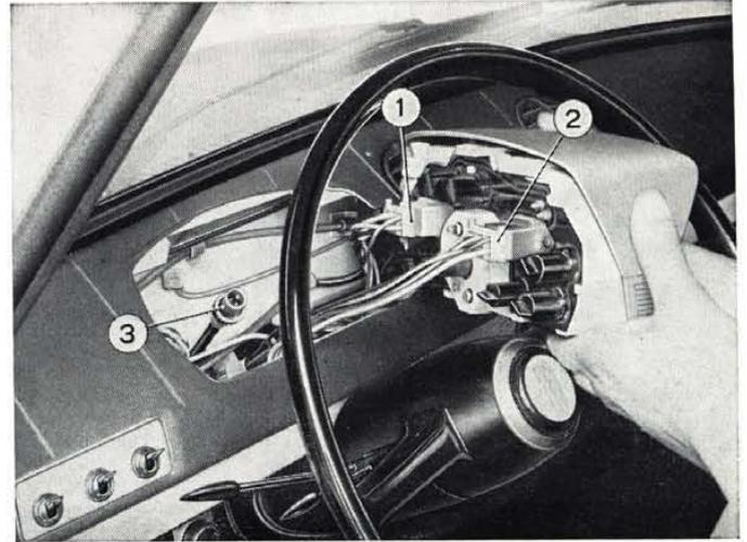
**Fig. 367 - Removing instrument cluster for replacement of bulbs.**
