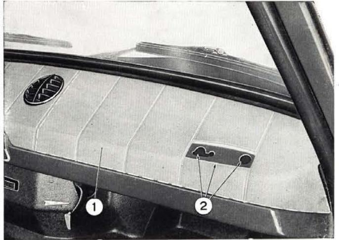
Fig. 380 - Fitting the templet for cutting out the instrument panel lining and fashioning the panel holes, preparatory to the radio set installation.
