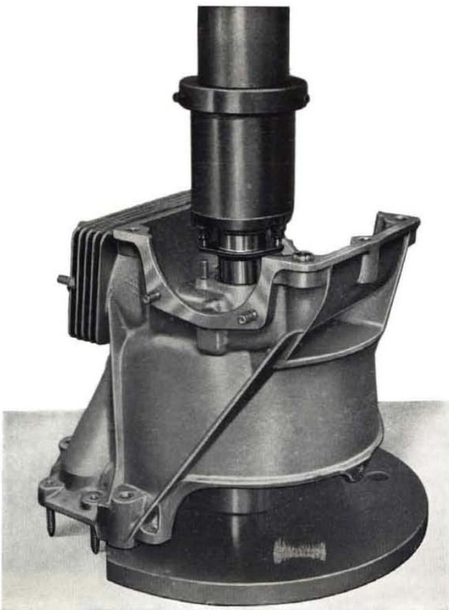
Fig. 576 - Assembling torque converter support.
