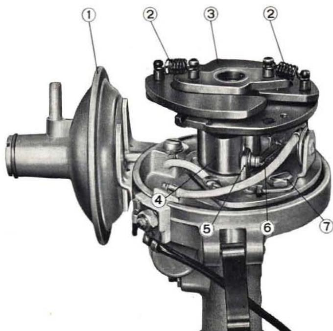
Fig. 352 - Ignition distributor with cover removed.
