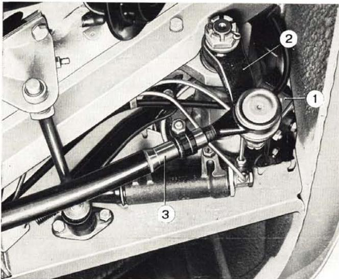
**Fig. 533 - Detail of steering linkage.**
