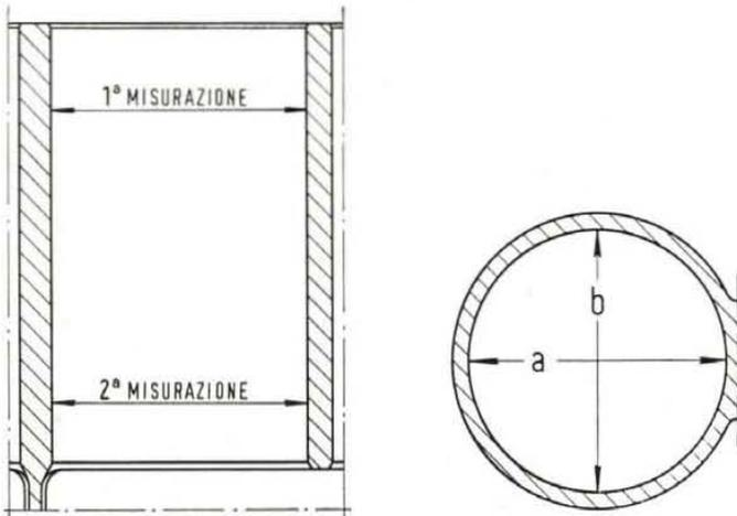
Fig. 27 - Diagram for measuring cylinder bores.
