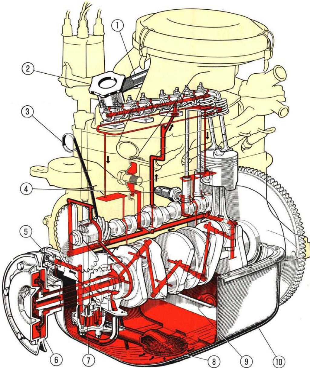
**Fig. 124 - Engine lubrication diagram (cut-away view).**
