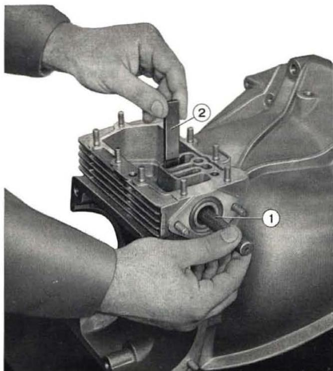
**Fig. 584 - Reassembling plunger valve.**
