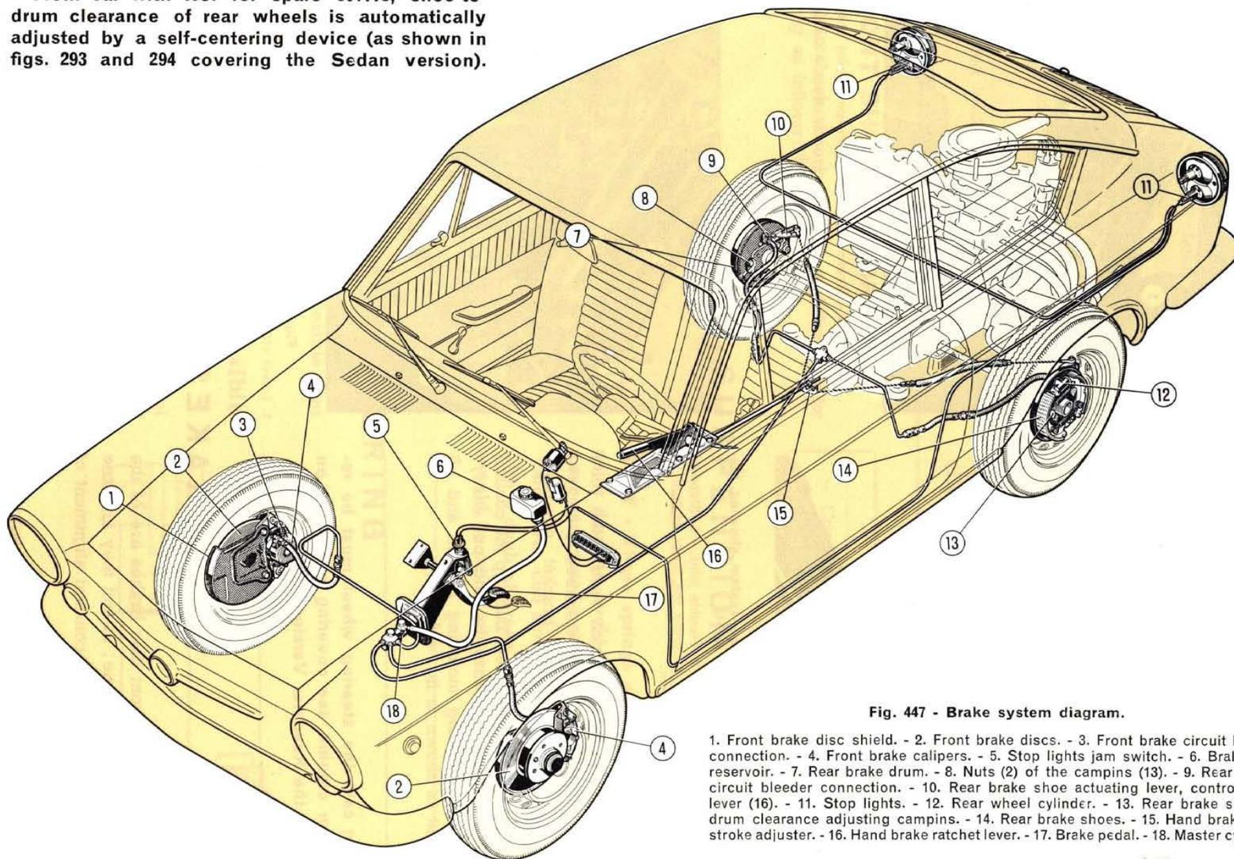
Fig. 447 - Brake system diagram.
