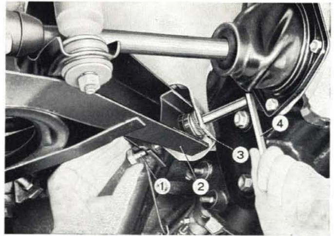
Fig. 256 - Securing rear control arm to body shell.
