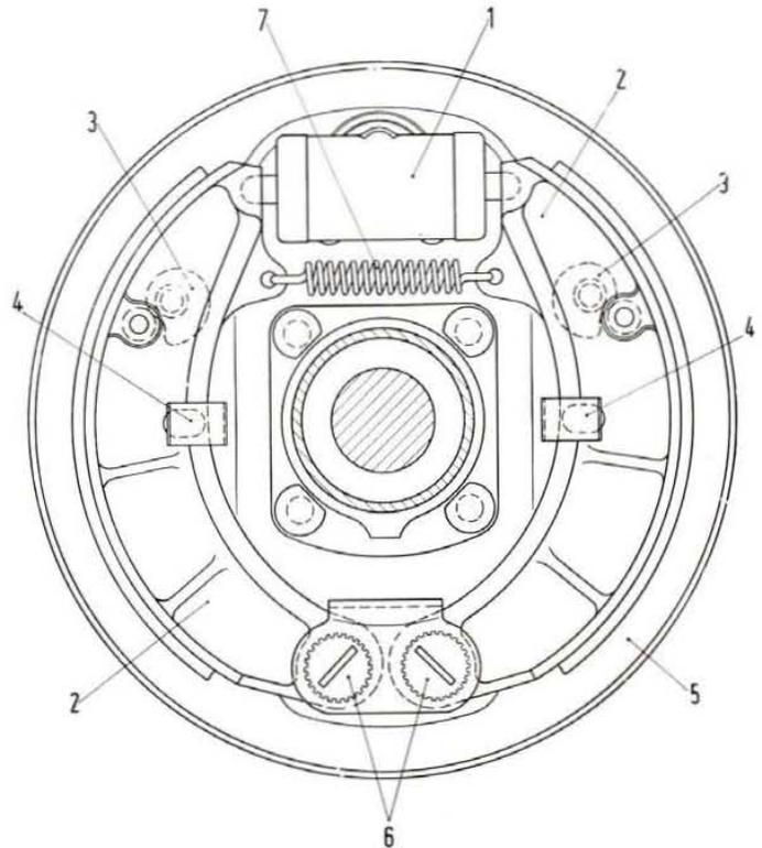
**Fig. 539 - Front wheel brake assembly.**
