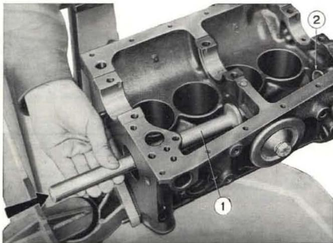
**Fig. 114 - Fitting intermediate camshaft bushing.**
