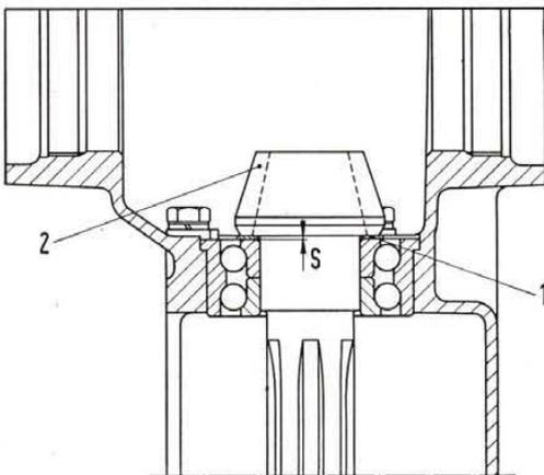
**Fig. 195 - Drive pinion and shim fitting diagram.**
