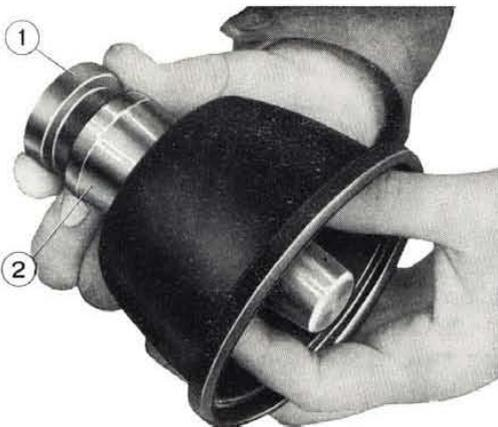
Fig. 191 - Fitting differential cage oil boot bushing.
