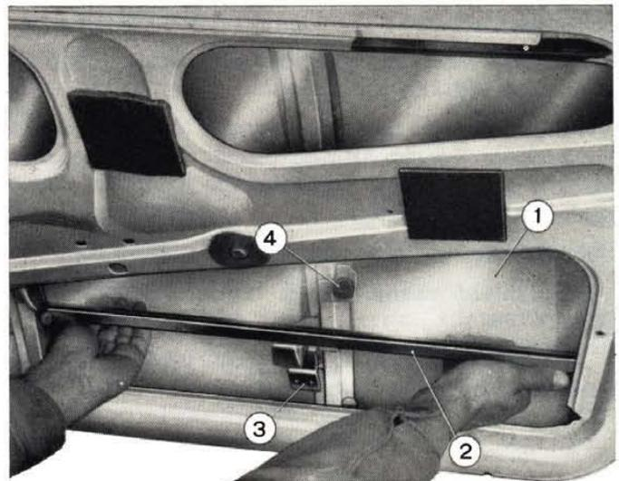
**Fig. 393 - Removing drop glass.**
