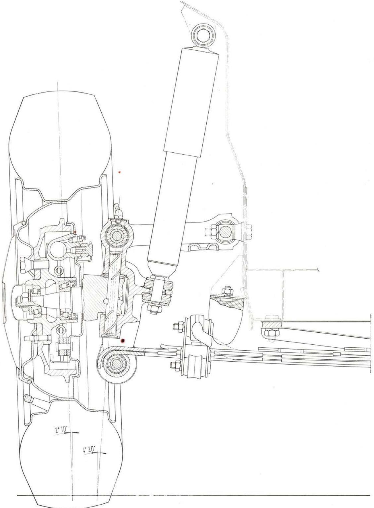
Fig. 209 - Sectional view of left side front suspension and wheel assembly.
