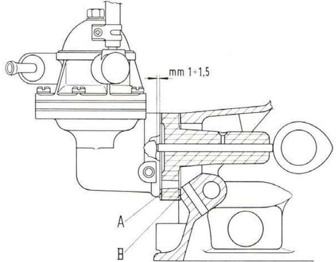
**Fig. 140 - Setting fuel pump push rod projection.**
