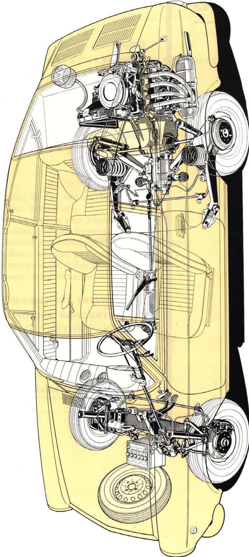
Fig. 415 - Phantom view of running gear units.
