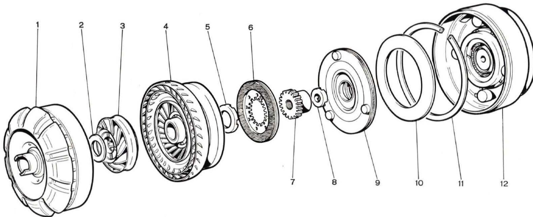
**Fig. 563 - Exploded view of torque converter.**
