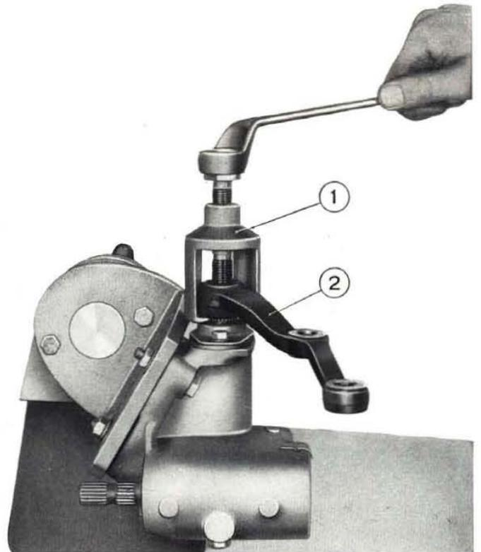
**Fig. 276 - Removing pitman arm.**
