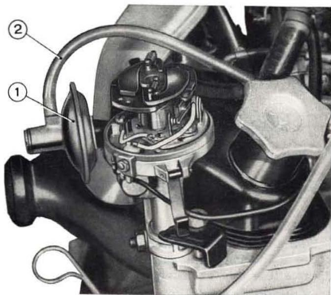
Fig. 353 - Ignition distributor in place on engine, with cover removed.
