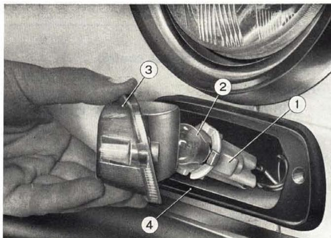
Fig. 363 - Opening front parking lamp.
