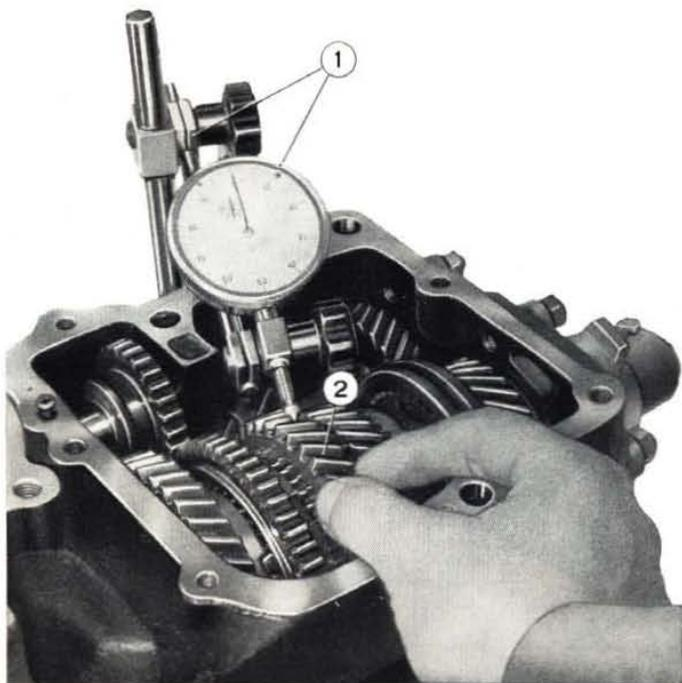
Fig. 175 - Checking gear backlash.
