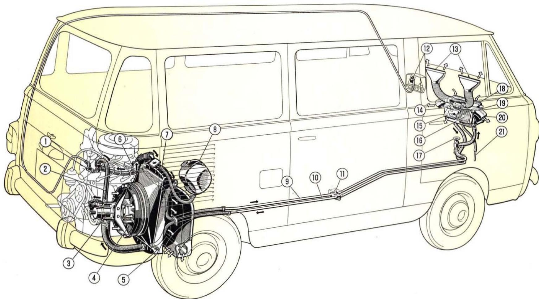
Fig. 545 - Engine cooling and car heating system.
