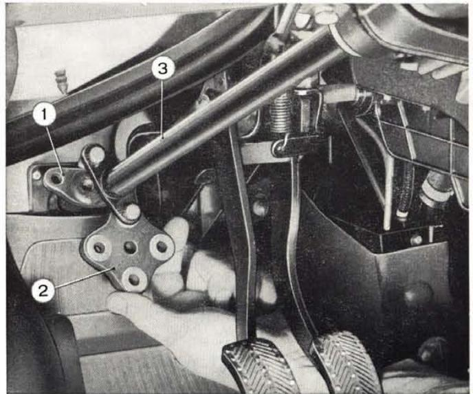
Fig. 446 - Removing steering column joint.
