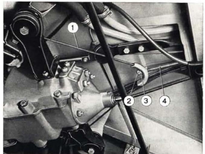
**Fig. 302 - Close-up view of manual parking brake control cable and stretcher.**
