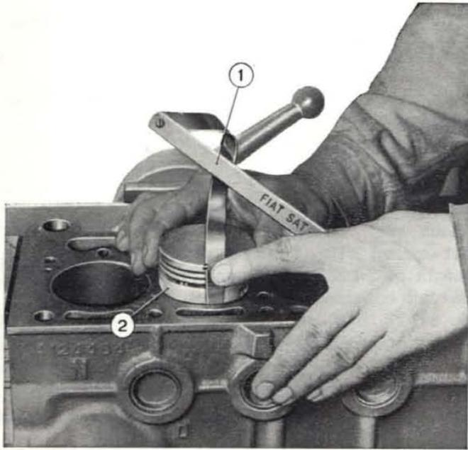
Fig. 40 - Checking piston clearance in cylinder bore.
