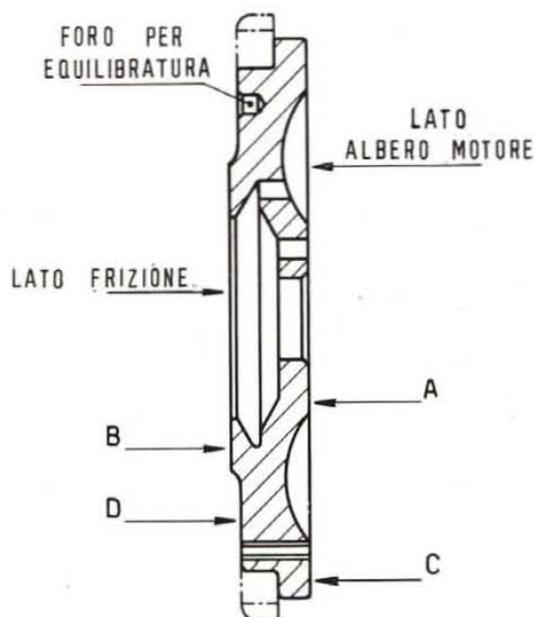
Fig. 71 - Diagram for checking flywheel mating faces to driven plate and crankshaft mounting flange.
