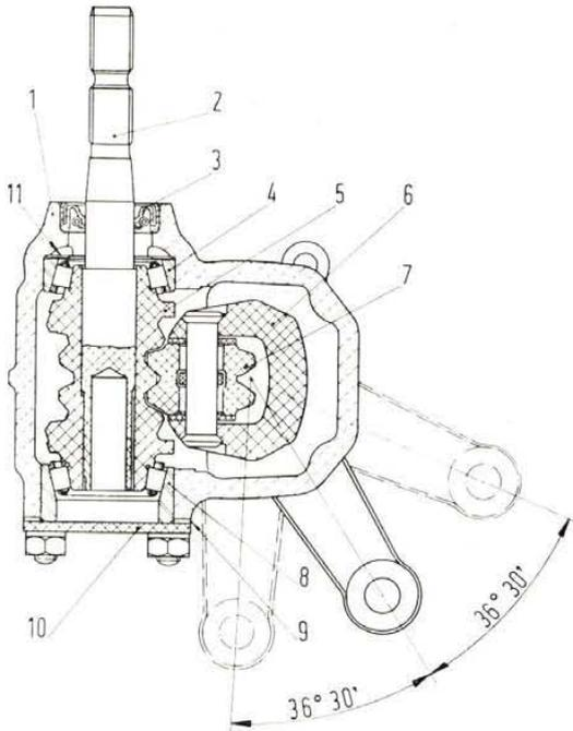
**Fig. 535 - Sectional view of steering gear at worm-to-roller shaft meshing plane.**
