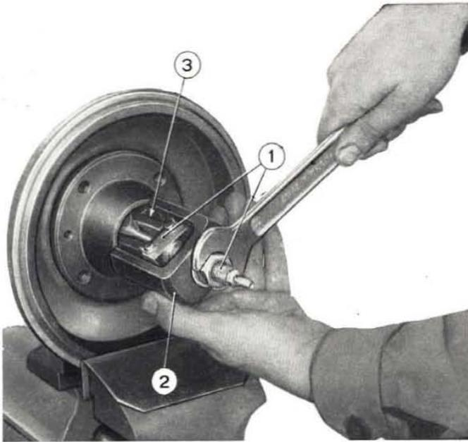
Fig. 224 - Pulling inner bearing cup.
