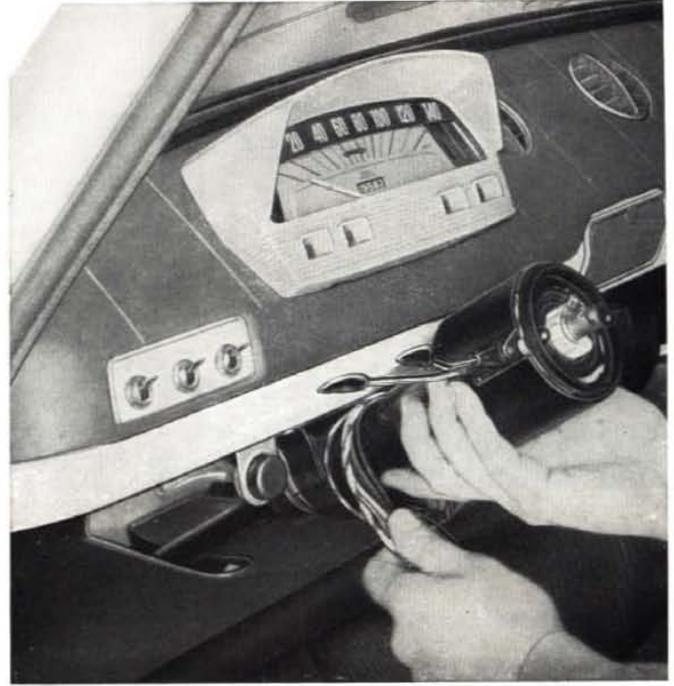
Fig. 374 - Removing direction signal and outer lighting selector switch.
