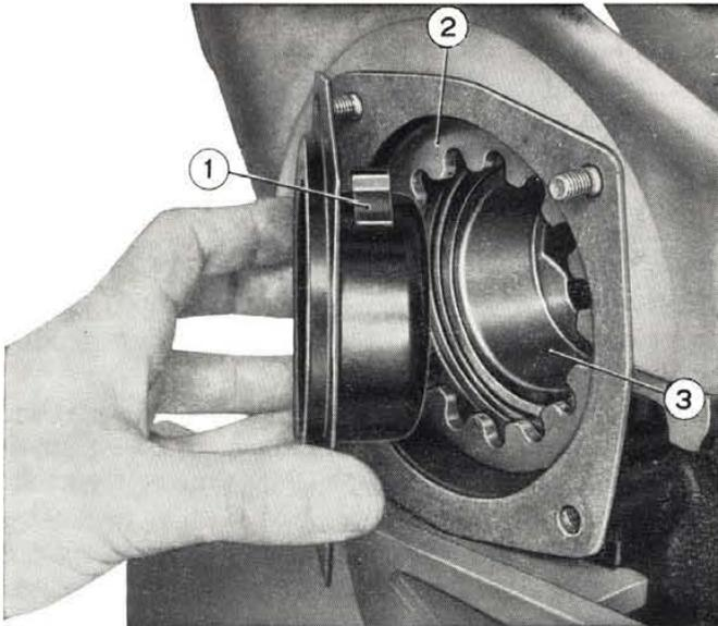
Fig. 190 - Fitting bearing adjuster stop plate.
