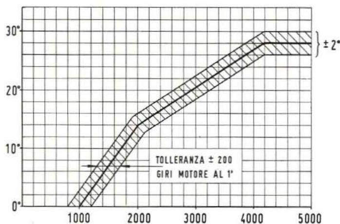
Fig. 349 - Diagram showing automatic advance of ignition distributor to engine 100 G.000.
