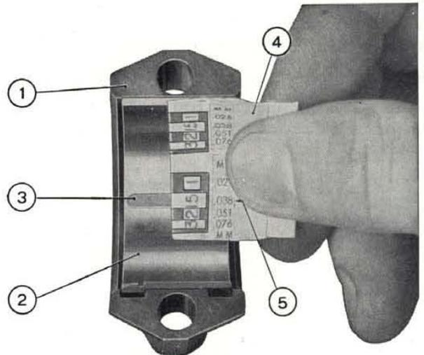
**Fig. 64 - Comparing the width of the flattened « Plastigage » with the envelope graduation scale to check connecting rod bearing insert-to-journal clearance.**
