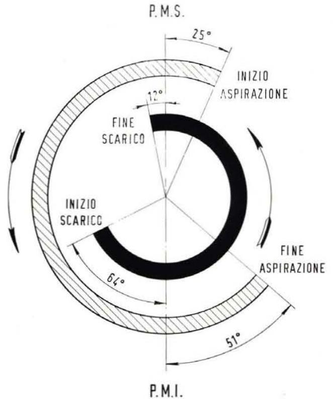
Fig. 429 - Valve timing diagram at increased tappet clearance of .0148" (0.375 mm).
