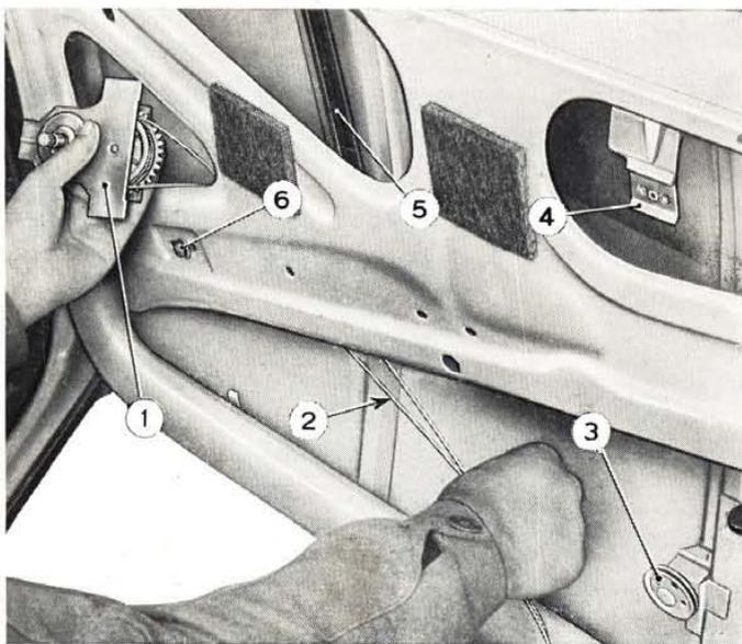
**Fig. 392 - Taking down window regulator assembly.**
