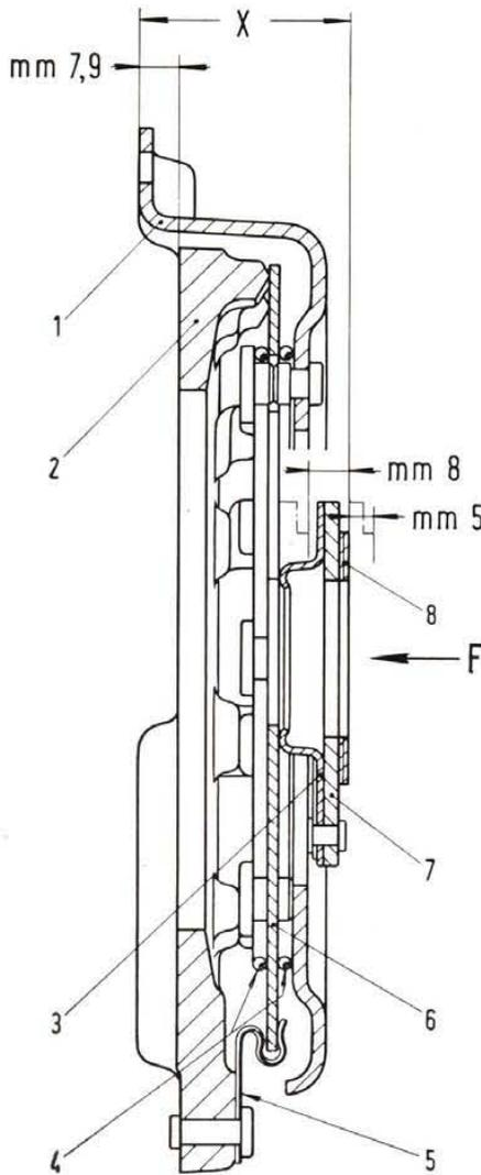
Fig. 161 - Clutch cover assembly inspecting diagram.
