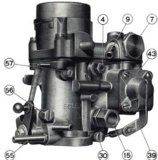
**Fig. 153 - View of Solex carburetor from idle setscrews end.**
