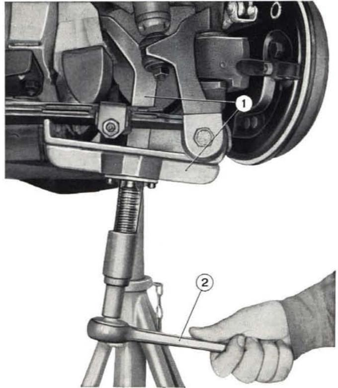
Fig. 232 - Setting semi-elliptic spring at « static load ». 1. Tool A. 74134 stressing semi-elliptic spring. - 2. Ratchet wrench A. 89854 for tool operation.
