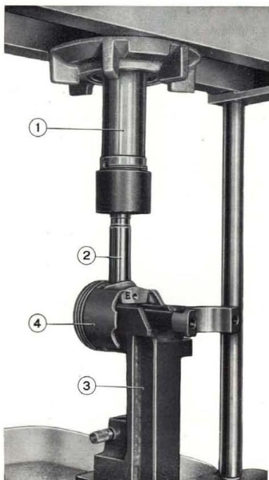
**Fig. 49 - Pressing out piston pin.**
