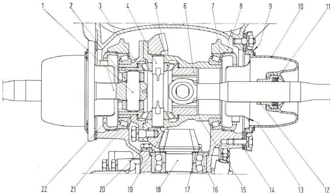
**Fig. 186 - Side sectional view of transmission-differential across differential cage, final gear set and axle shaft slip joints.**
