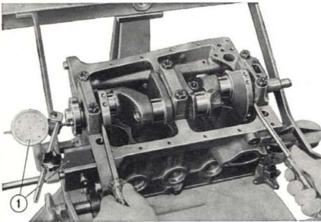
Fig. 80 - Checking crankshaft end play.
