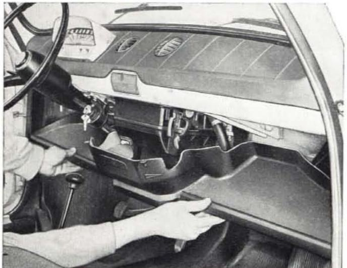
Fig. 306 - Withdrawing utility shelf.
