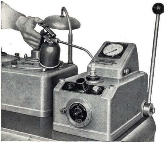
Fig. 355 - Testing a spark plug for gas tightness.
