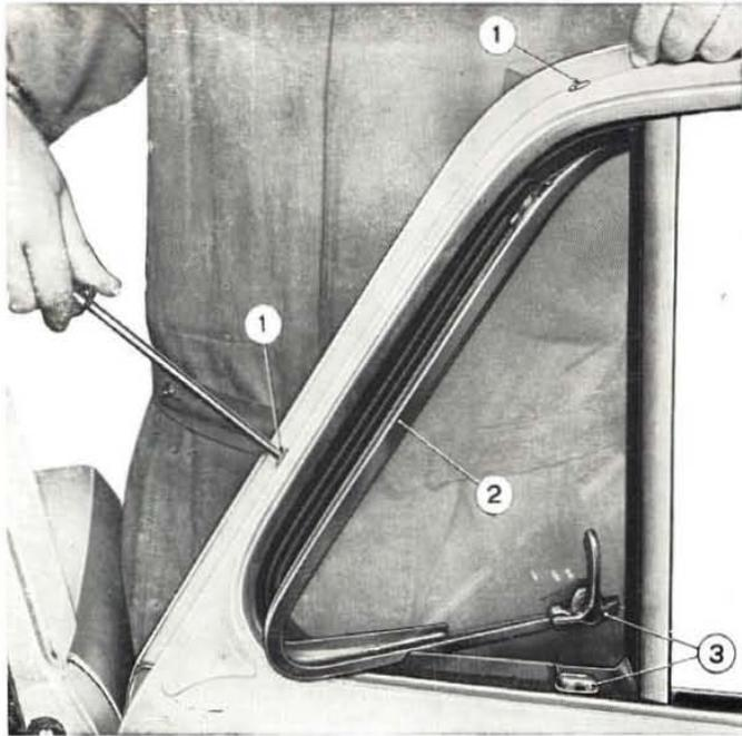
Fig. 389 - Removing ventilator window.
