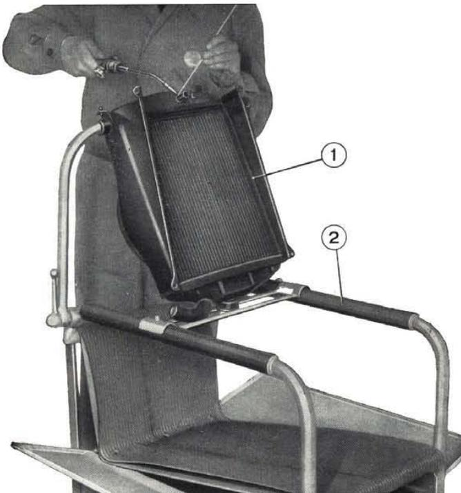
**Fig. 134 - Tinning the radiator.**
