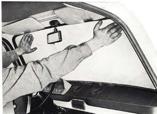
Fig. 405 - Removing windshield glass.
