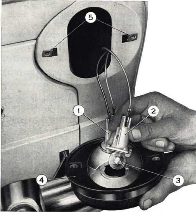
**Fig. 365 - Removing tail light.**
