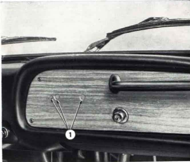
Fig. 503 - Instrument panel with location marks for drilling radio receiver mounting holes.
