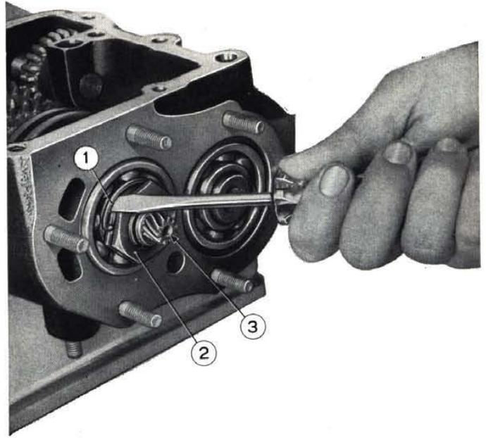
Fig. 173 - Prying out countershaft-drive pinion nut lock ring.
