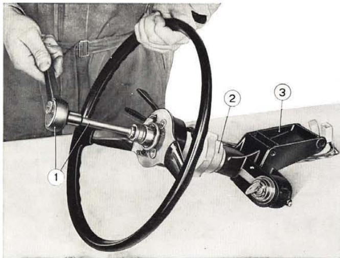
**Fig. 489 - Removing steering wheel on work bench.**
