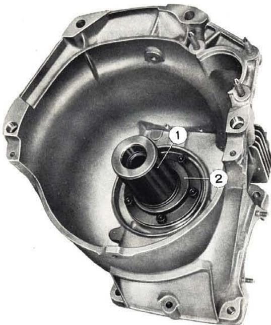
**Fig. 580 - Fitting pump oil seal.**
