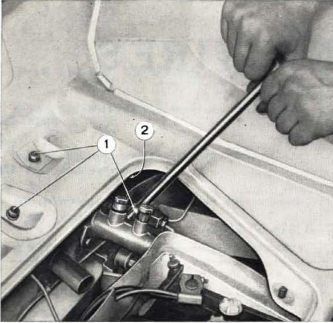
**Fig. 300 - Removing brake and clutch pedal mounting board.**
