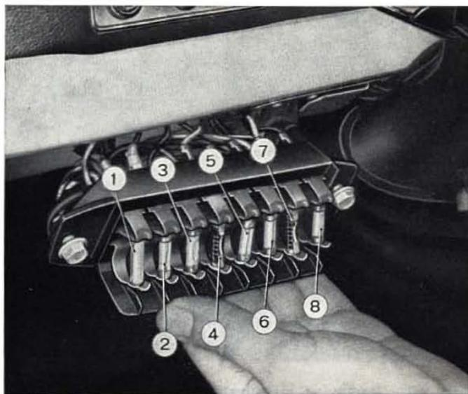
**Fig. 369 - Electrical system fuses.**
