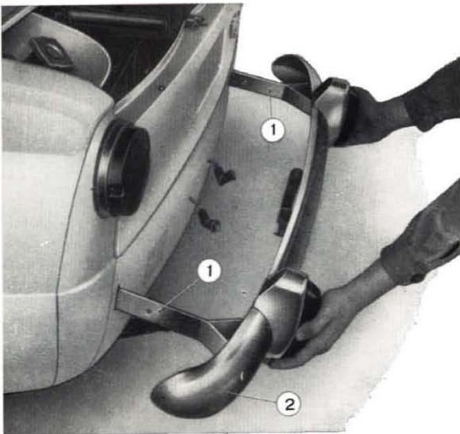
Fig. 408 - Removing rear bumper.
