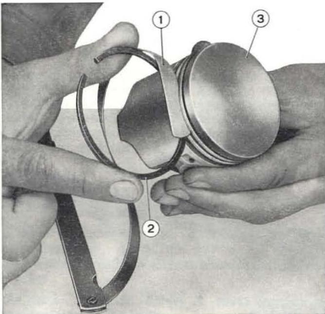
**Fig. 47 - Checking piston ring side clearance.**
