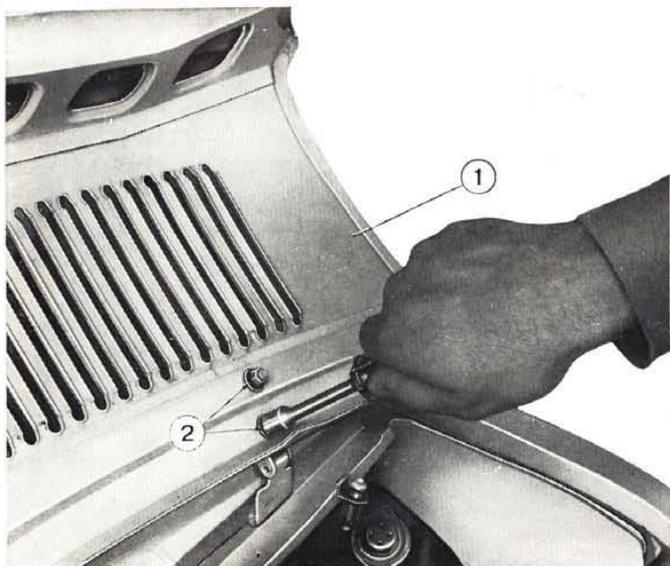
Fig. 403 - Repositioning engine compartment lid.
