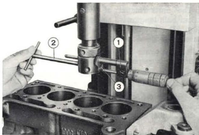
Fig. 32 - Measuring cutter projection, preparatory to boring operation.
