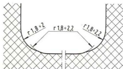
Fig. 68 - Fillet radii for intermediate main bearing journal shoulder.
