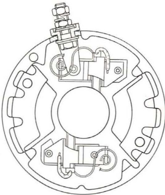
Fig. 550 - End sectional view of generator across commutator end head.
