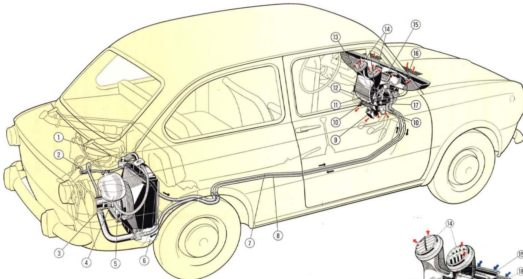
**Fig. 303 - Phantom view of air conditioning system in car interior.**
