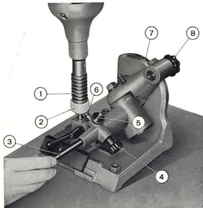
Fig. 92 - Dressing taper grindwheel A. 94084 on dressing machine Ap. 5050.
