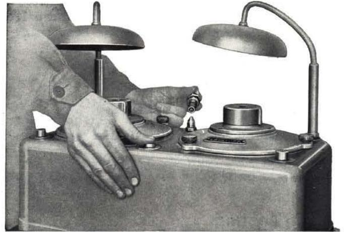
Fig. 356 - Blowing a spark plug after sanding and washing.
