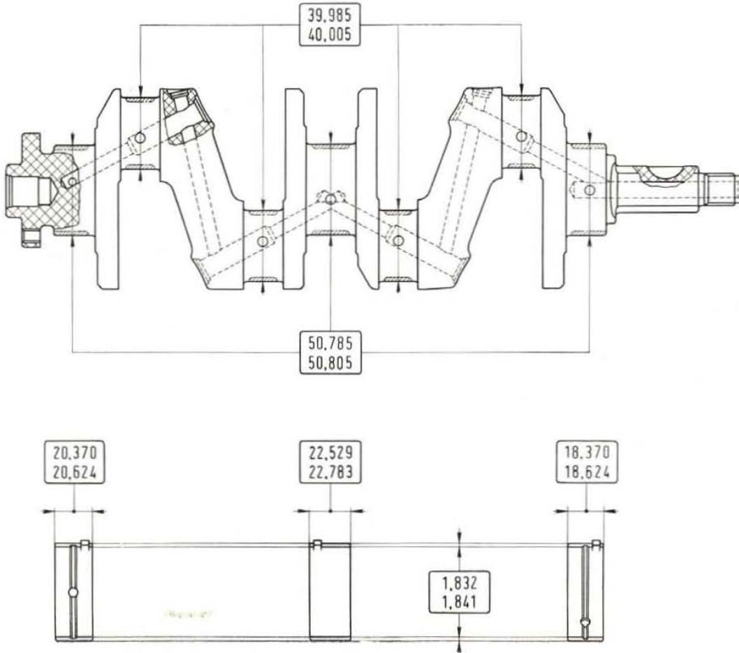
Fig. 75 - Critical dimensions (metric) of crankshaft and main bearing inserts.
