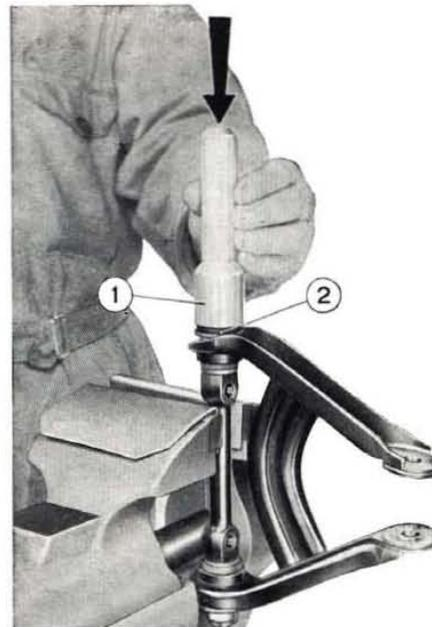
Fig. 227 - Installing upper control arm bushings.
