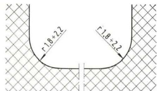
Fig. 69 - Fillet radii for connecting rod bearing journal shoulders.
