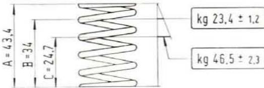
Fig. 424 - Outer valve spring specifications.
