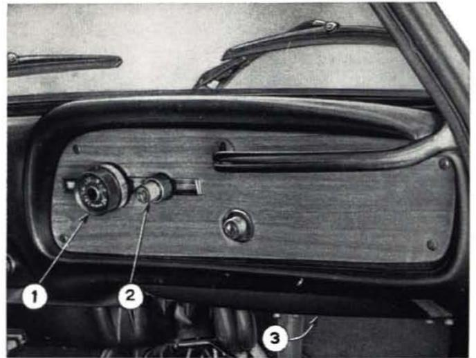
Fig. 505 - Radio receiver installed on car.
