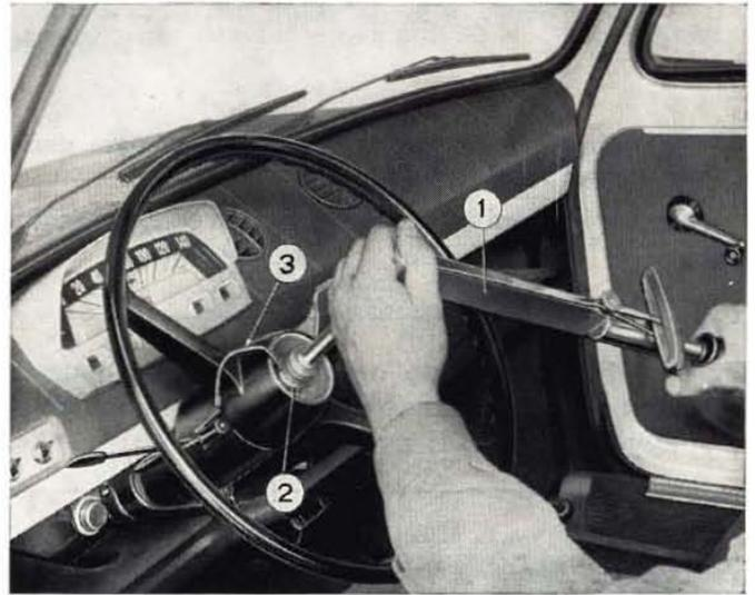
**Fig. 272 - Tightening steering wheel mounting nut.**
