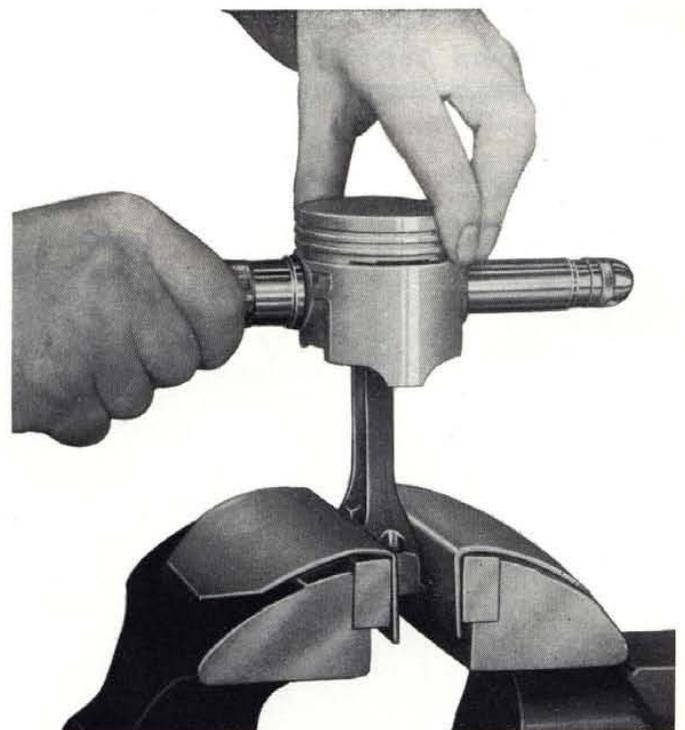
**Fig. 55 - The piston pin will be installed correctly when the shoulder of tool A. 60275 abuts against the piston boss.**
