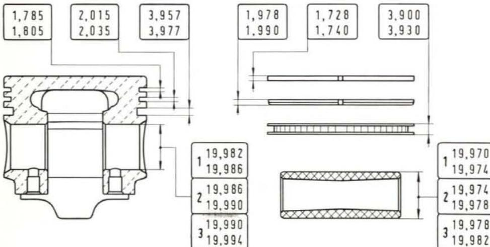
Fig. 43 - Critical dimensions (metric) of pistons, pins and rings.
