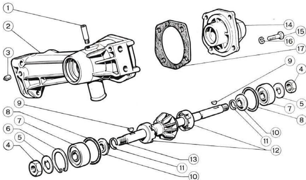
Slide off cover (14) and from cover interior take out ball bearing (7), retainer (8) and thrust washer (10).
