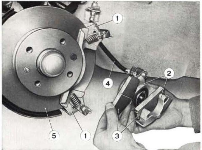
Fig. 453 - Replacing lining pads.
