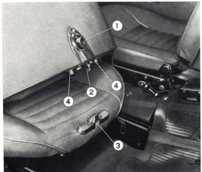
Fig. 477 - Front seat back rest catch device.
