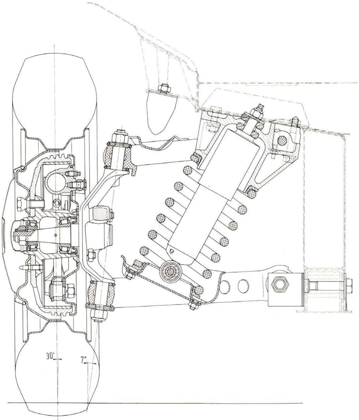
**Fig. 522 - Sectional view of left side front suspension and wheel assembly.**
