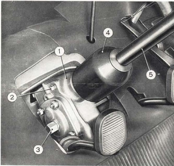
**Fig. 532 - Steering gear viewed from car interior.**
