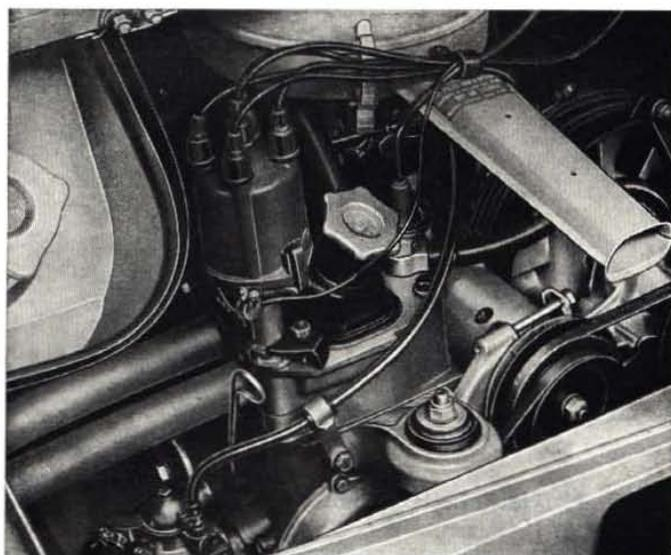
Fig. 459 - Scrap view of engine compartment. In foreground, the ignition distributor without vacuum advance corrector.
