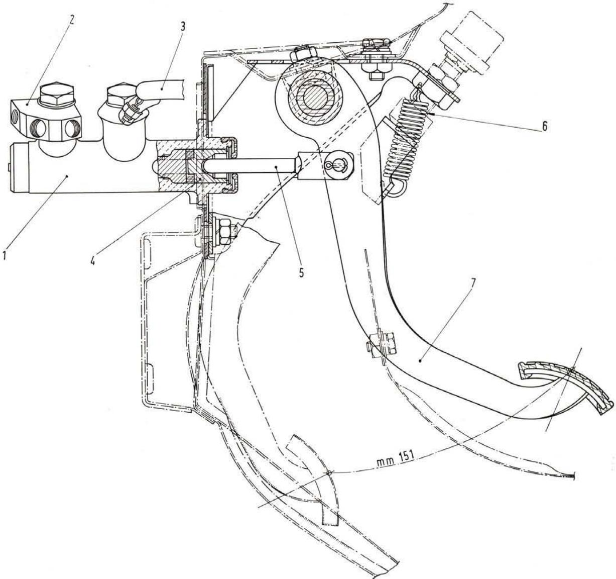
Fig. 299 - Brake pedal and master cylinder assembly.
