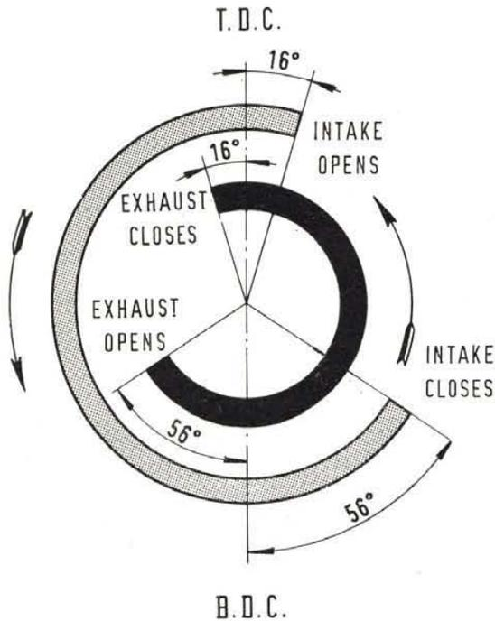
Fig. 118 - Valve timing diagram at increased tappet clearance of .0148" (0.375 mm).
