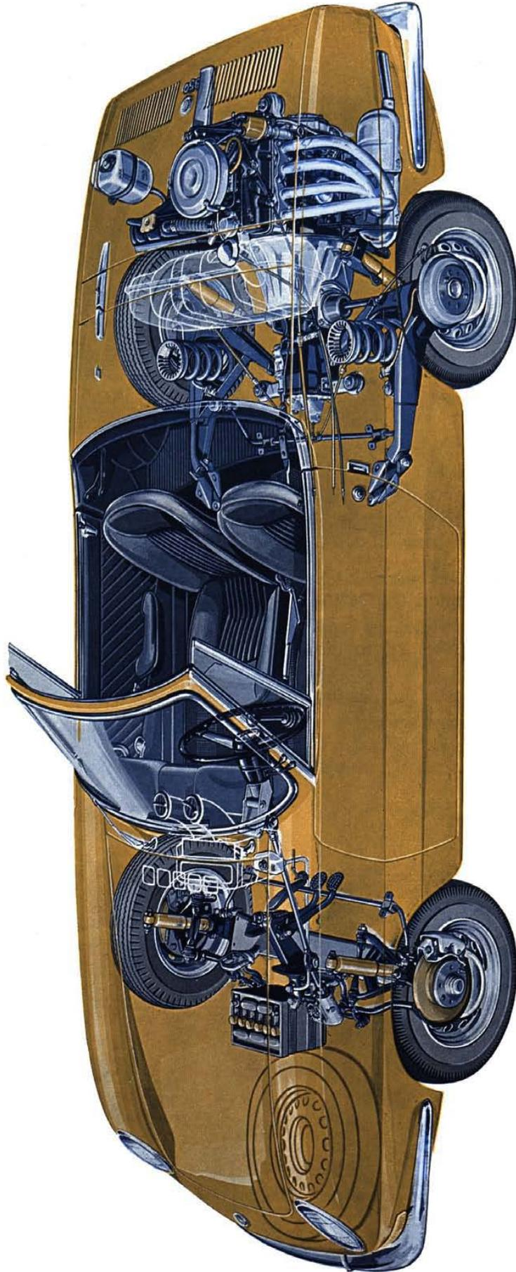
Fig. 480 - Phantom view of 850 Roadster running gear units.
