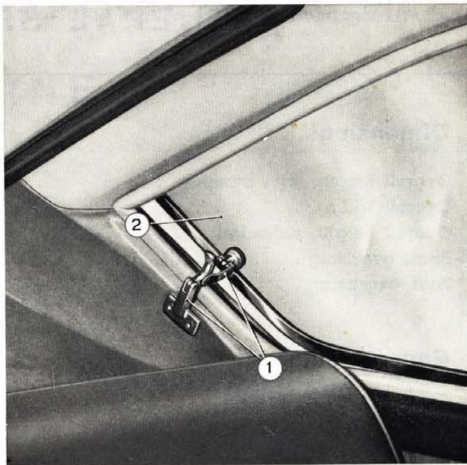
Fig. 419 - Detail of rear quarter door window adjuster.
