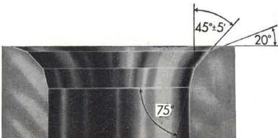
Fig. 98 - View of a valve seat which has been reseated with 20° and 75° cutters.
