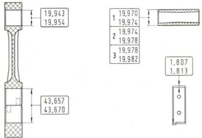
Fig. 60 - Critical dimensions (metric) of connecting rod, rod bearing insert and piston pin. (Late type)
