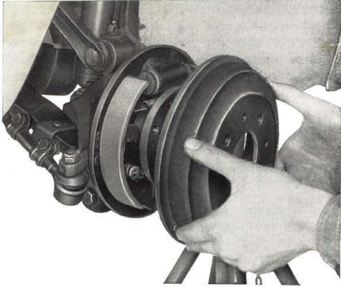
Fig. 292 - Removing brake drum.
