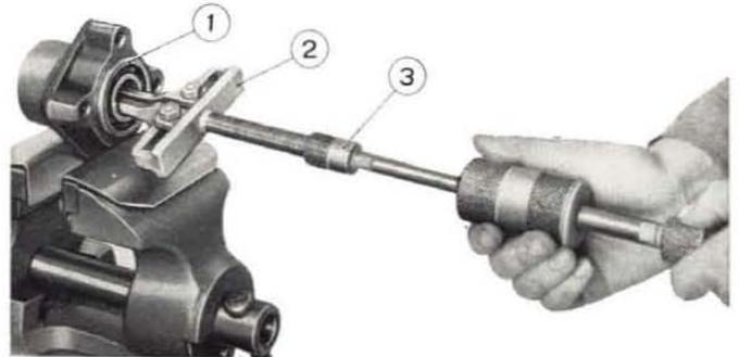
**Fig. 246 - Pulling rear wheel ball bearing.**
