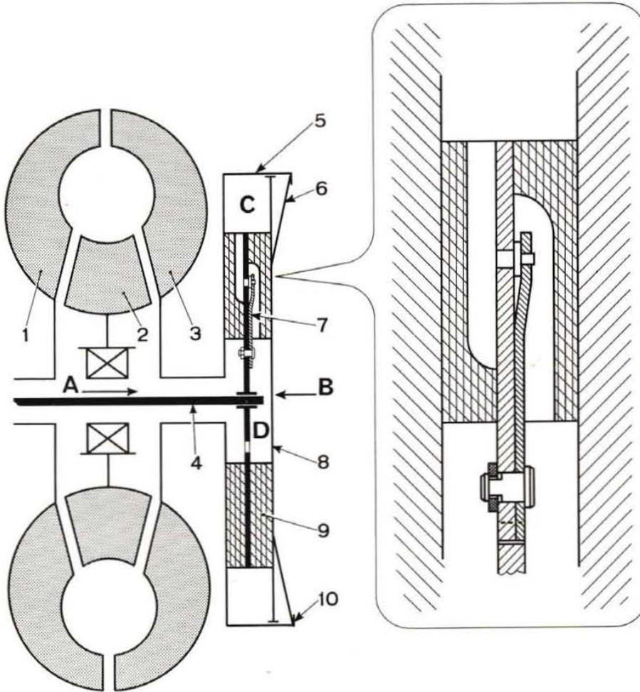
Fig. 569 - Operating diagram of release mechanism.
