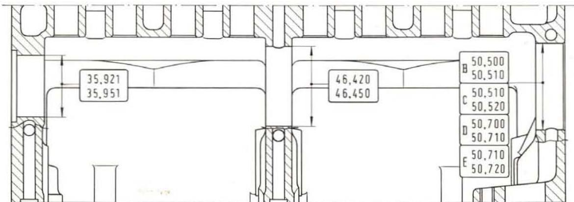
Fig. 35 - Critical dimensions (metric) of camshaft bushing seats.
