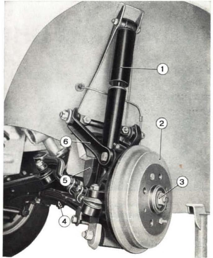
**Fig. 269 - Detail of left side front suspension and wheel.**
