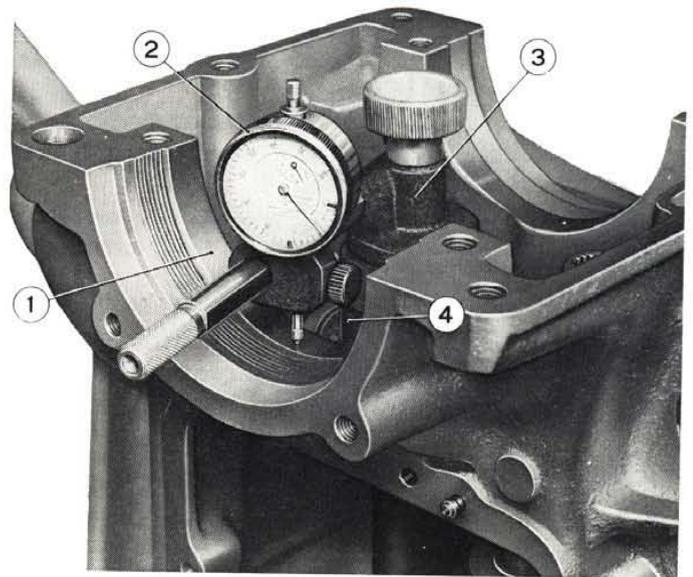
**Fig. 196 - Step for figuring the thickness of drive pinion shim.**
