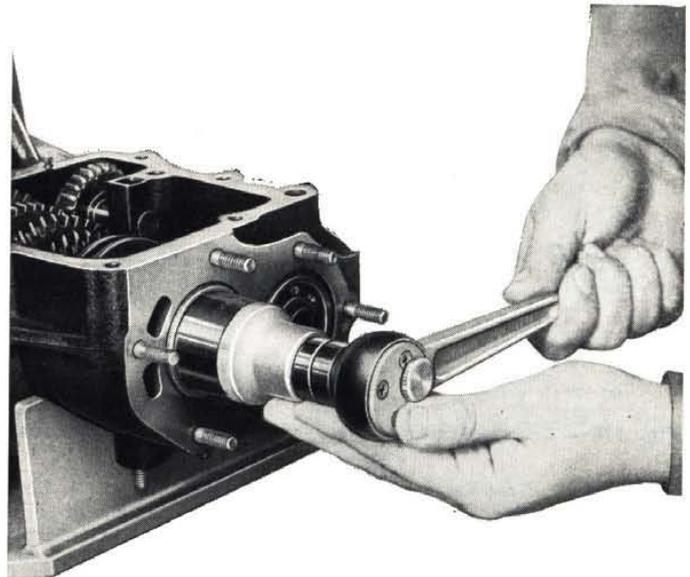
Fig. 174 - Using ratchet wrench A. 89854 to remove countershaft nut.
