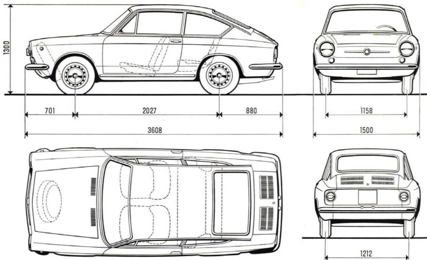
Fig. 418 - Leading dimensions (in mm).
