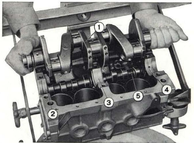
Fig. 15 - Lifting out crankshaft.
