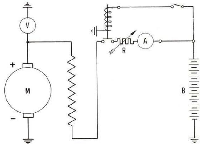
**Fig. 343 - Wiring diagram for starting motor operation test.**
