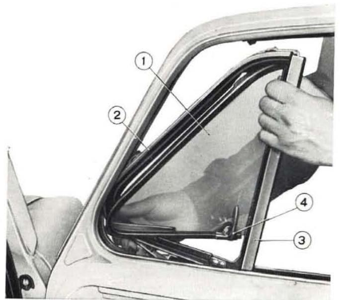
Fig. 390 - Withdrawing ventilator window assembly.
