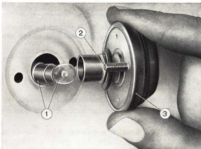
Fig. 364 - Removing side direction signal lamps.
