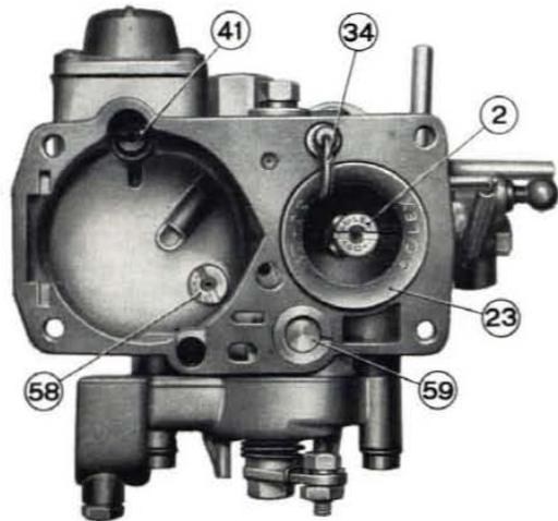
Fig. 149 - Interior view of Solex carburetor body.
