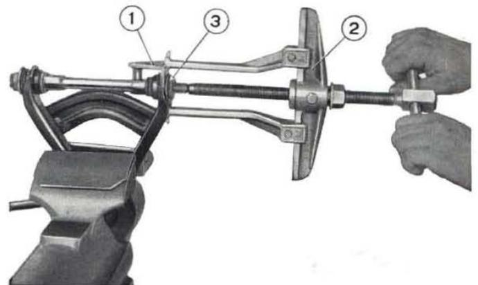
**Fig. 213 - Pulling upper control arm bushings.**
