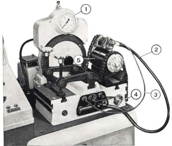
Fig. 345 - Operation test of starting motor, loaded and at no-load.
