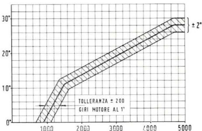
Fig. 351 - Diagram showing automatic advance of ignition distributor to engine 100 G.002.
