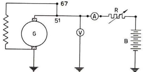
Fig. 319 - Wiring diagram for motoring test.
