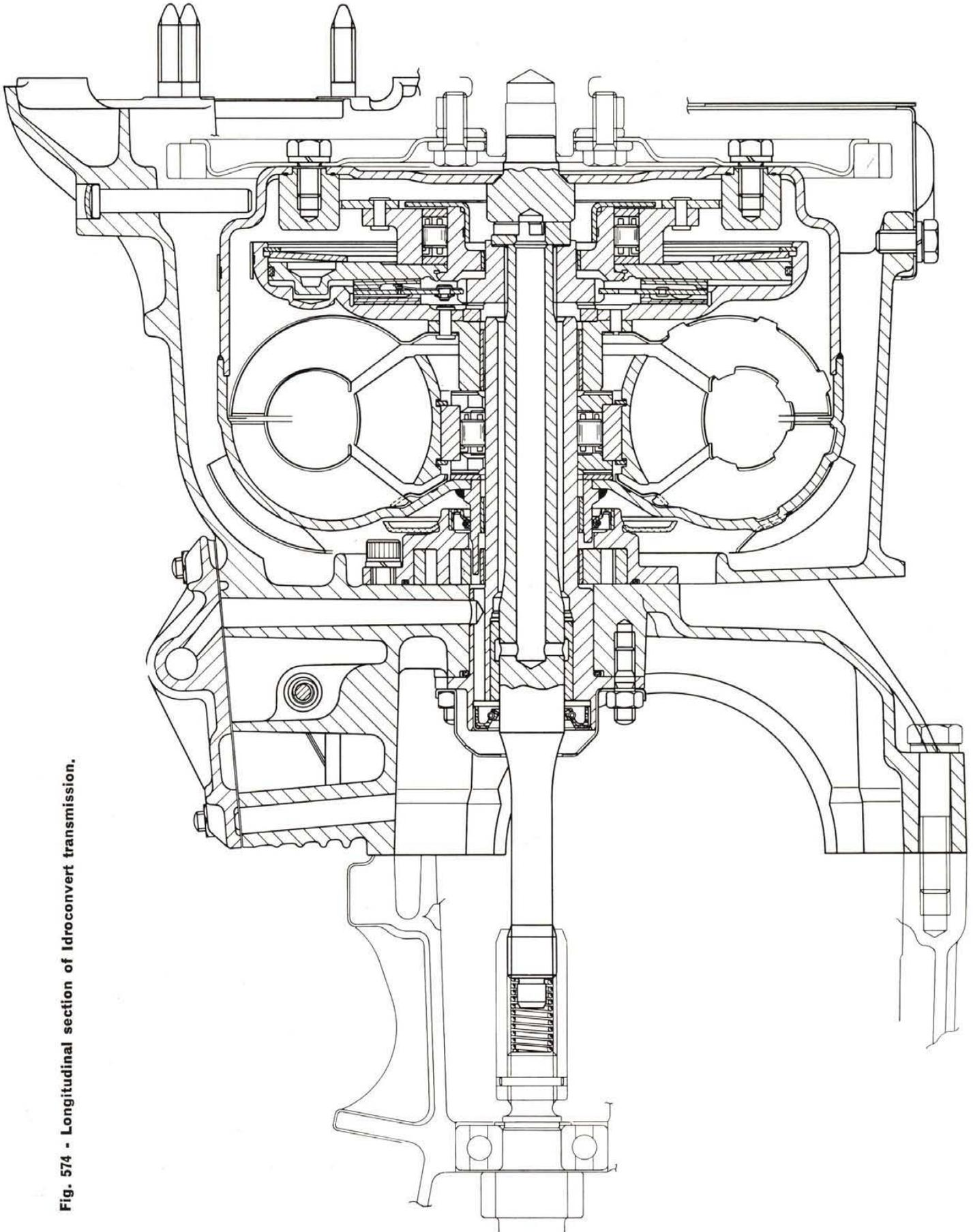
Fig. 574 - Longitudinal section of Idroconvert transmission.
