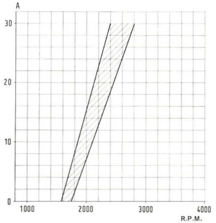
Fig. 551 - Output curve, warm, of DN 62 L generator. Steady voltage: 12.
