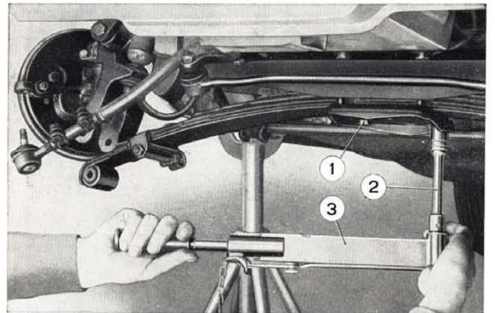
Fig. 231 - Securing semi-elliptic spring to body shell.
