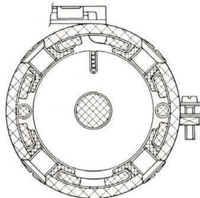
Fig. 342 - Transverse section view across pole shoes and field winding.
