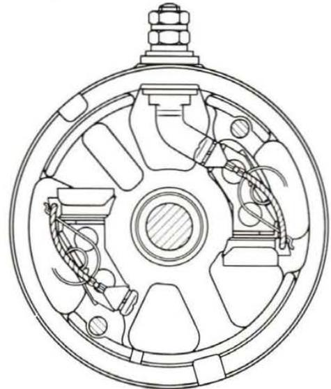
Fig. 317 - End sectional view of generator across armature shaft and view of commutator end head.
