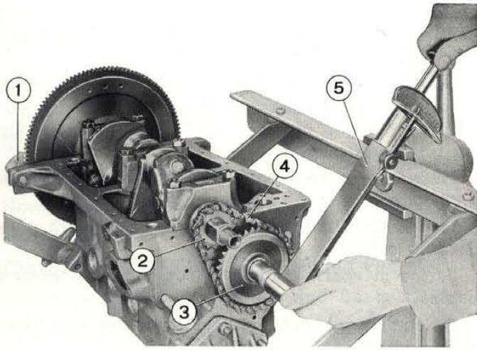
**Fig. 19 - Tightening camshaft driven sprocket screw.**
