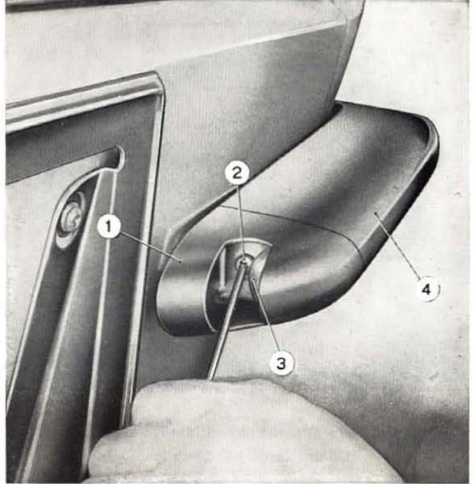
Fig. 498 - Disassembling license plate lamp.
