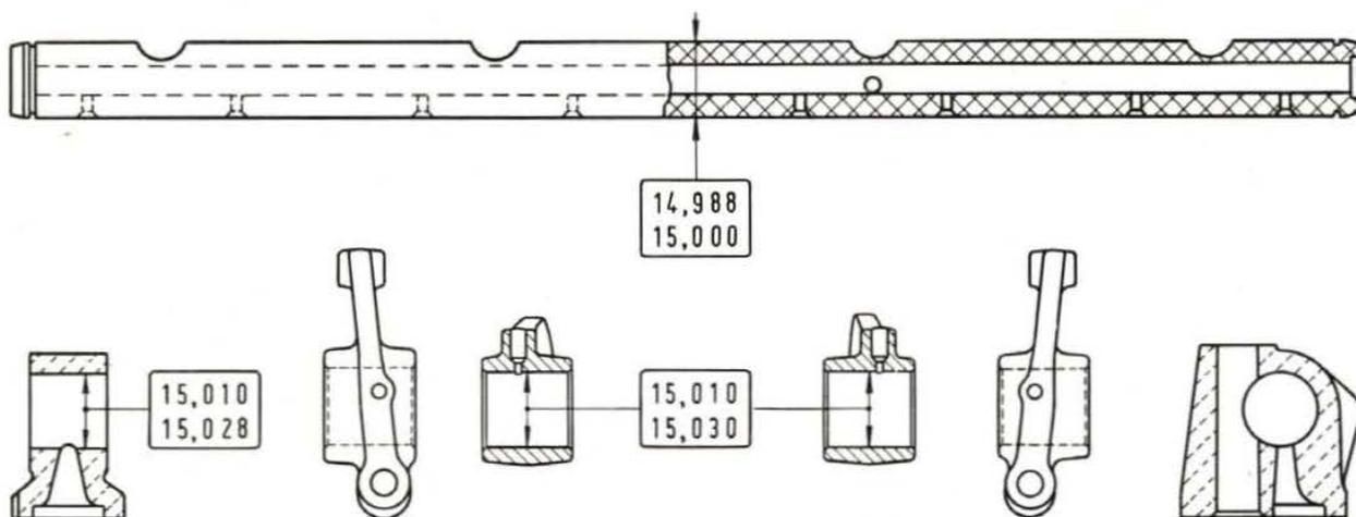
Fig. 110 - Critical dimensions (metric) of rockers, shaft and supports.
