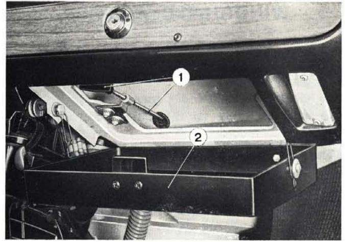
Fig. 514 - Close-up view of utility compartment. 1. Engine compartment lid release control. - 2. Utility drawer, drop type.
