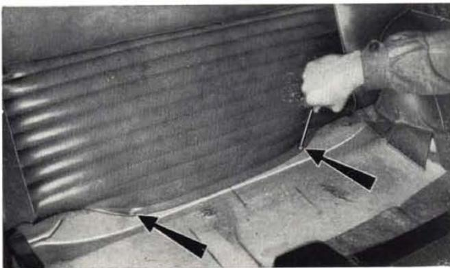
Fig. 475 - Removing rear seat back rest. Arrows point to back rest holding screws.
