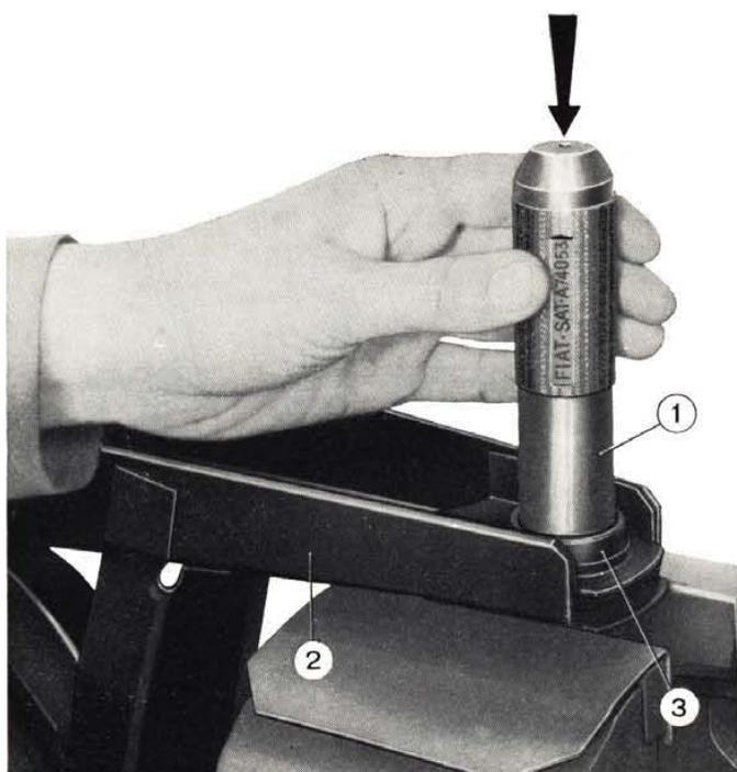
**Fig. 248 - Installing control arm bushing.**
