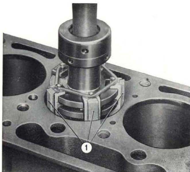
Fig. 30 - Honing cylinder barrels.
