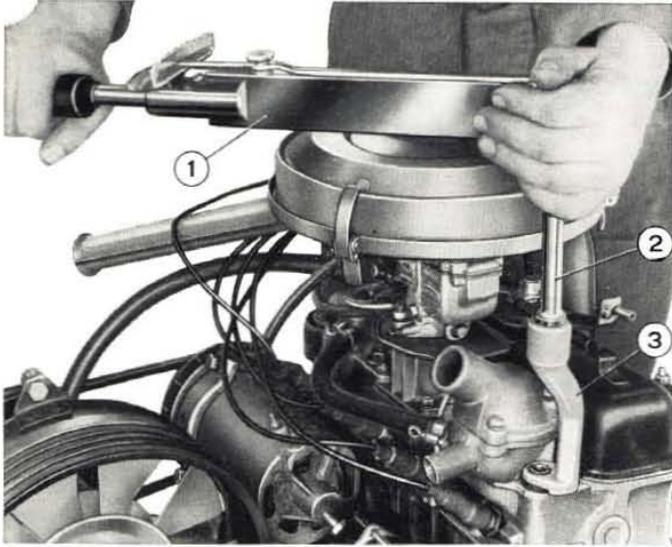
Fig. 136 - Fitting thermostat to engine.
