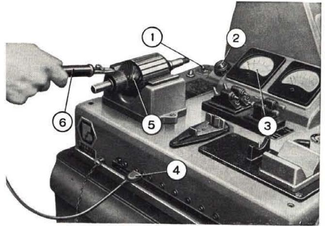
Fig. 324 - Testing generator armature for open coils.
