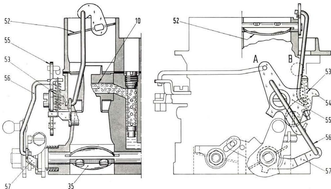
Fig. 433 - Diagrammatic section views of Weber 30 DIC 1 carburetor.
