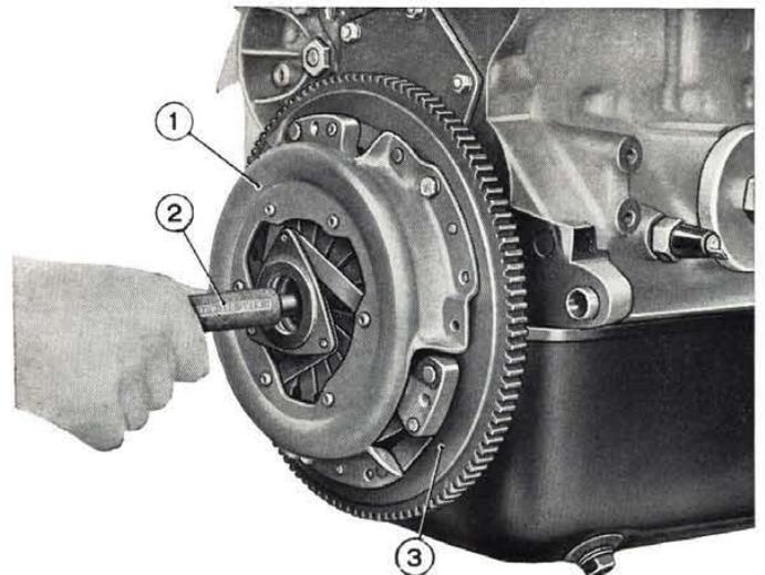
Fig. 162 - Using tool A. 70085 to align the driven plate.
