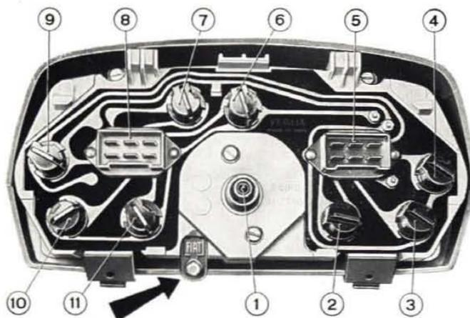
Fig. 372 - Rear view of the instrument cluster.
