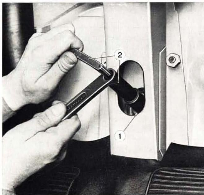
Fig. 524 - Disconnecting shock absorber at top end.
