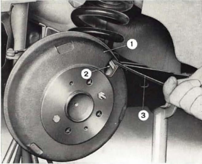
**Fig. 541 - Checking shoe-to-drum clearance at right side rear wheel.**
