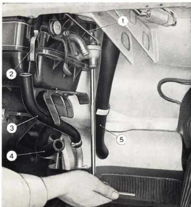
**Fig. 307 - Removing air conditioner.**
