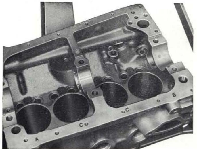
Fig. 29 - Letters showing cylinder bore classes on lower face of cylinder block.
