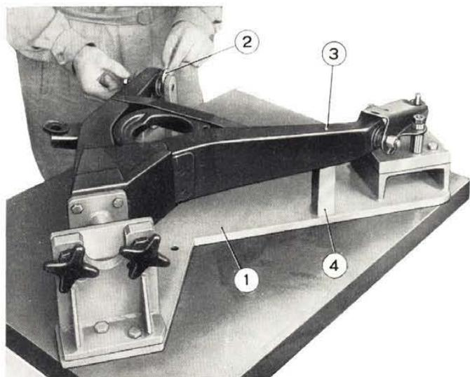
**Fig. 250 - Adjusting rear control arm.**
