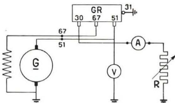
Fig. 322 - Wiring diagram for the generator heating test.
