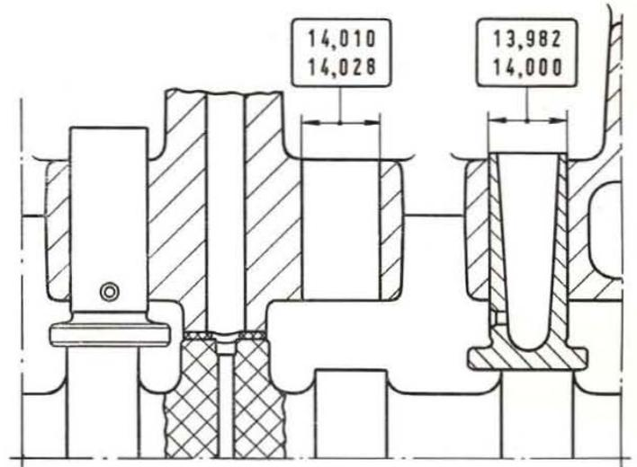
Fig. 37 - Critical dimensions (metric) of tappets and tappet seats on crankcase.
