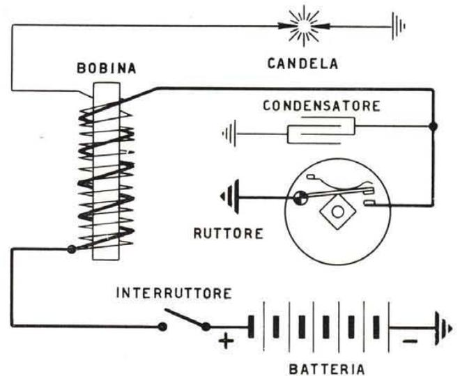
Fig. 348 - Ignition system wiring diagram.
