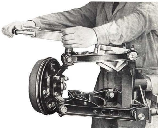
Fig. 531 - Tightening kingpin screw to upper control arm with unit on fixture **A. 22229**.
