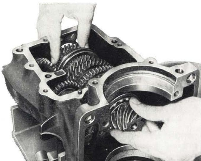
Fig. 179 - Installing the counter gear train and the countershaft-drive pinion.
