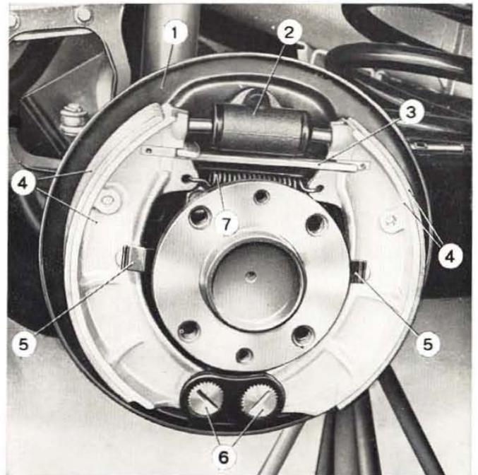
**Fig. 544 - Right side rear wheel brake assembly.**
