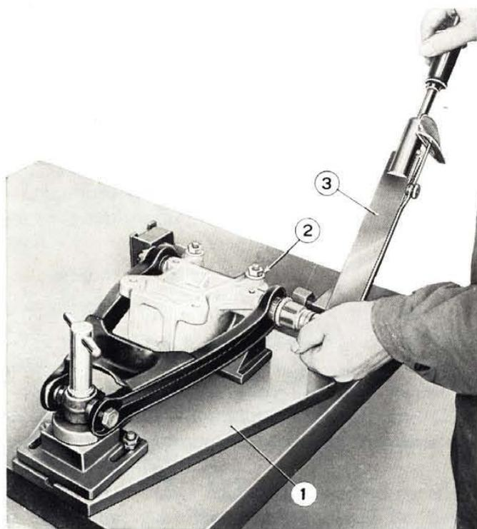
Fig. 527 - Tightening upper control arm pivot bar nuts. 1. Fixture A. 74023. - 2. Coil spring mounting bracket. - 3. Torque wrench.
