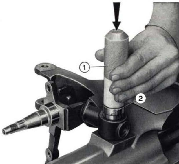
Fig. 225 - Inserting « estendblock » bushing in kingpin housing upper eye.
