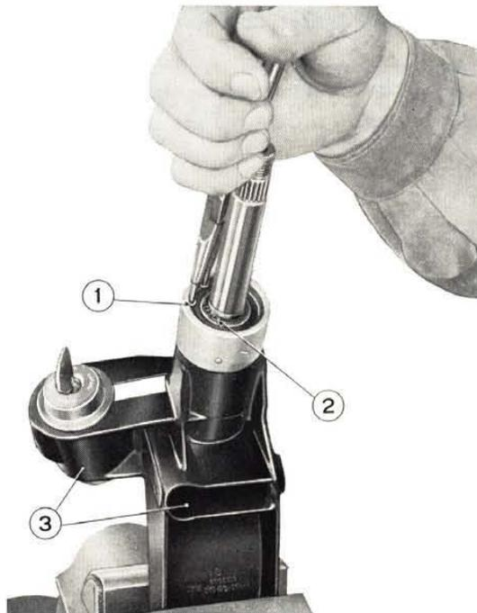
**Fig. 491 - Removing steering column bracket bearing snap rings.**
