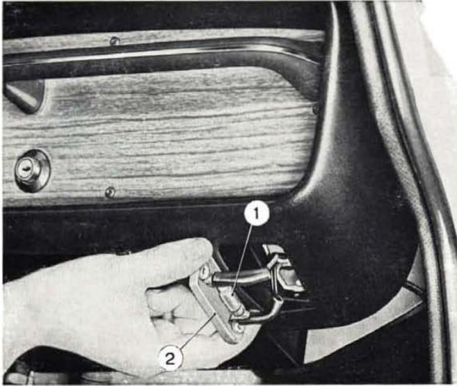
**Fig. 500 - Disassembling interior lamps.**
