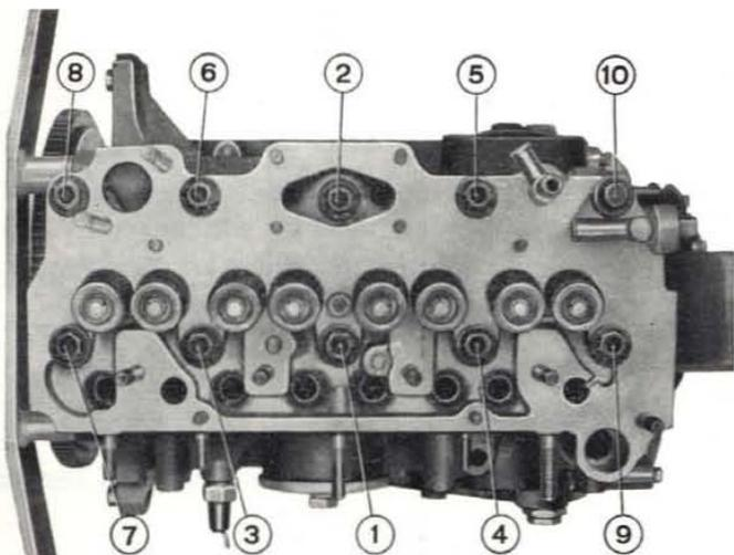
**Fig. 84 - Cylinder head screws tightening sequence.**
