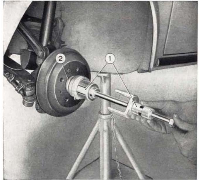
**Fig. 212 - Pulling wheel hub cap.**
