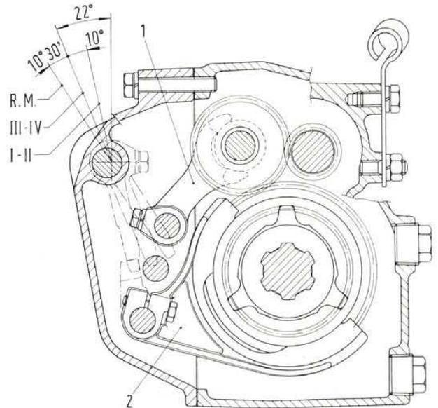
**Fig. 185 - End sectional view of transmission across shifter rail.**
