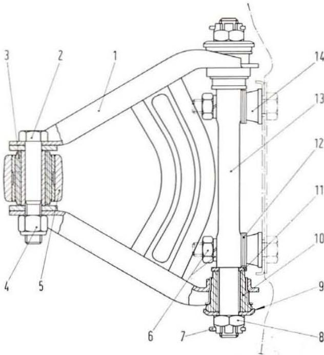
Fig. 219 - Front suspension: sectional view across control arm.
