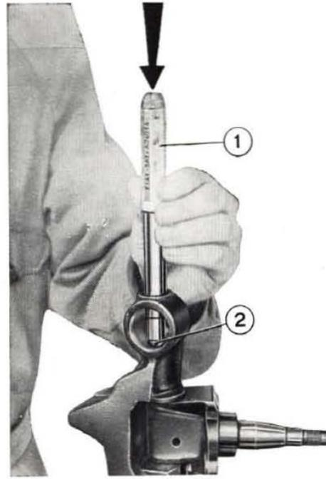
Fig. 226 - Installing kingpin.
