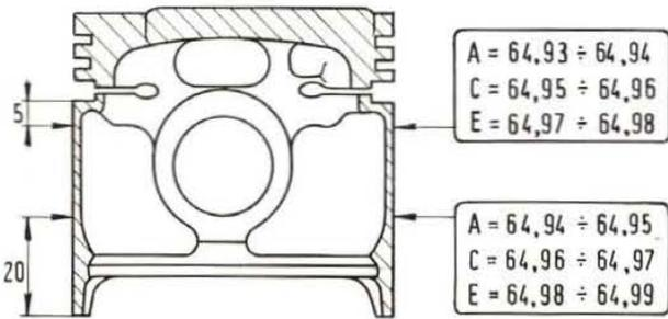
Fig. 421 - Skirt diameter (metric) of 100GC.000 engine measured at class grading points.
