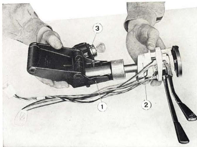
**Fig. 490 - Removing outer light and direction signal selector switch from steering column.**
