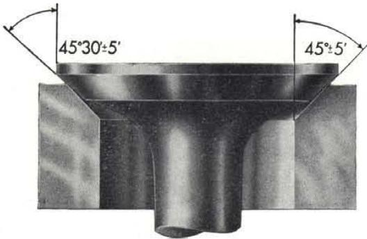
Fig. 95 - Inclination angles of valve seats in head and valve faces.
