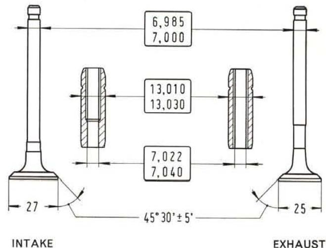
Fig. 103 - Critical dimensions (metric) of intake valves, exhaust valves and valve guides.
