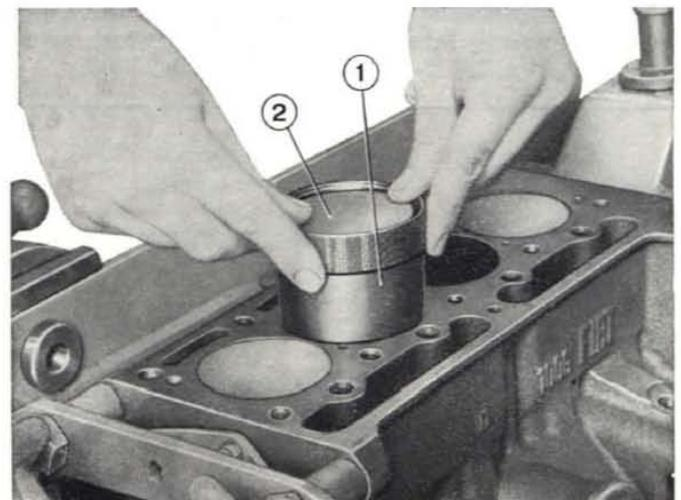
Fig. 62 - Installing connecting rod-piston assembly. 1. Tool A. 60273. - 2. Piston complete with pin and rings.
