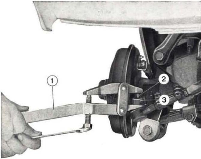
**Fig. 210 - Tying off tie rod from knuckle arm.**
