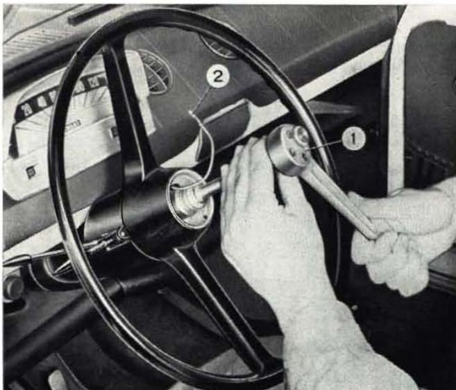
**Fig. 271 - Backing out steering wheel mounting nut.**
