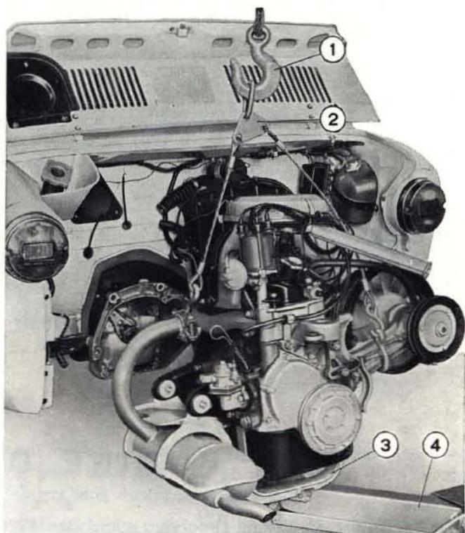
**Fig. 9 - Lifting out engine.**
