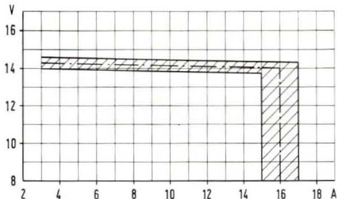
Fig. 328 - Generator regulator GN 2/12/16: Volt-Ampere curve on battery at 122°±5° F (50°±3° C). - Generator speed 4,500 rpm.
