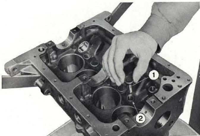
Fig. 16 - Fitting tappets.
