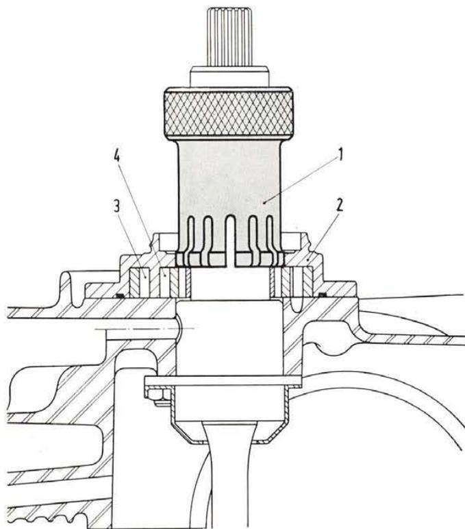
**Fig. 593 - Centralising the oil pump.**
