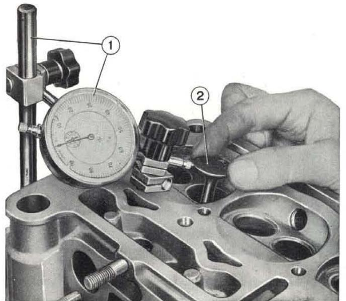
Fig. 100 - Checking clearance of valve stem in guide.
