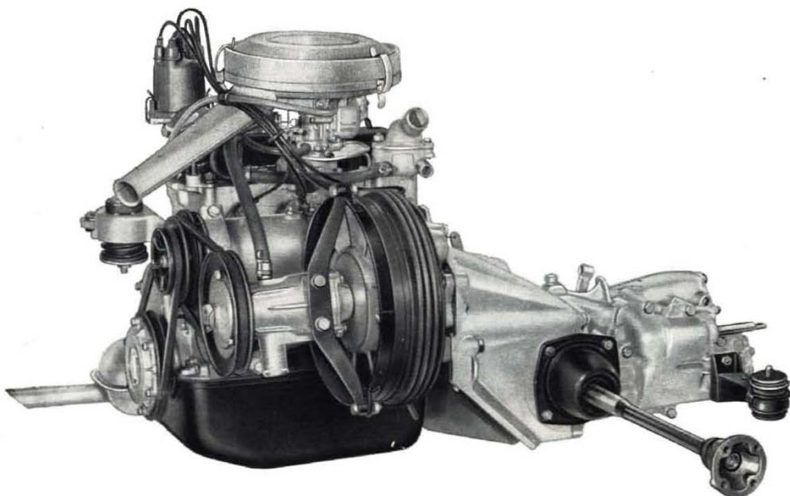
Fig. 141 - Engine transmission and differential assembly.
