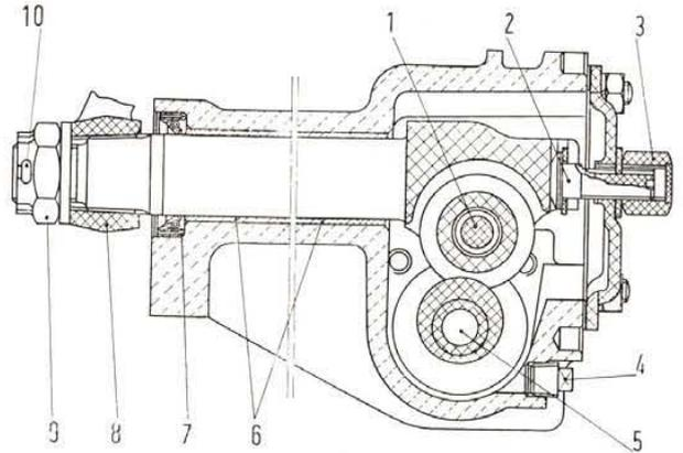
**Fig. 536 - Sectional view of steering gear across roller shaft and pitman arm.**
