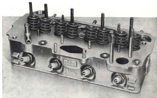
Fig. 107 - Cylinder head with valve springs and spark plugs.
