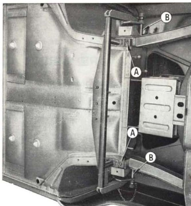
Fig. 414 - Detail showing use of gauge A. 74141 for checking underbody front.
