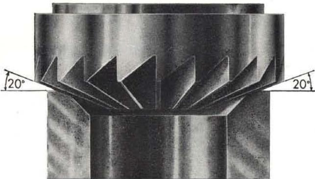
Fig. 96 - Narrowing valve seat at top with 20° cutter.
