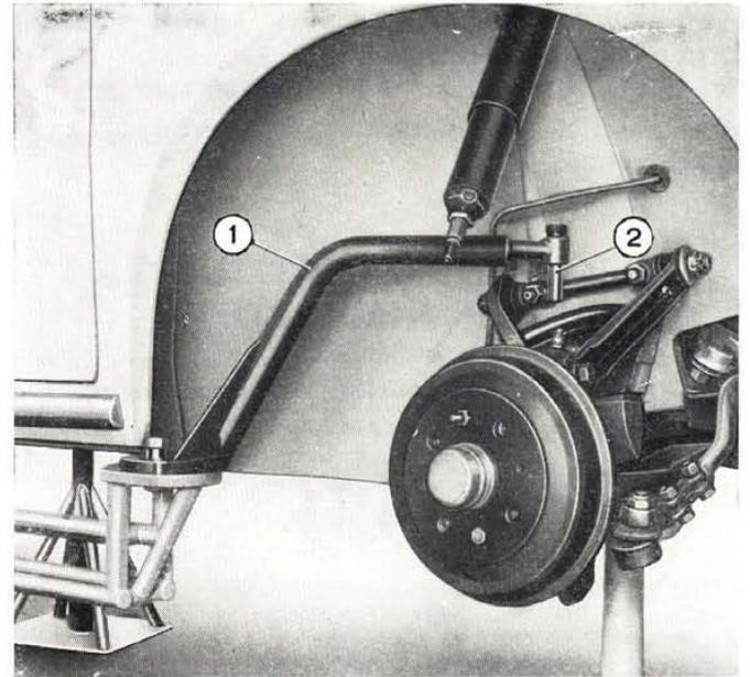
Fig. 267 - Checking rear wheel toe-in.
