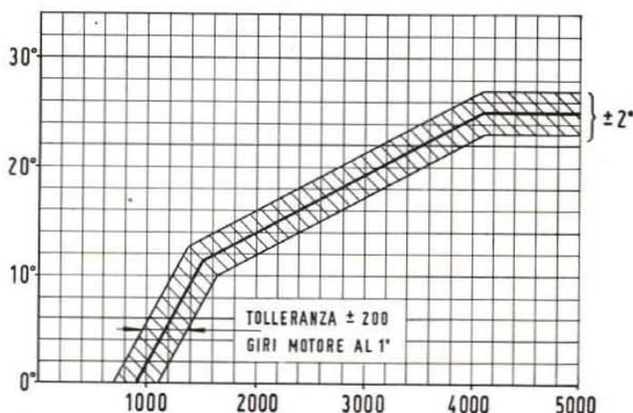
Fig. 350 - Diagram showing automatic advance of ignition distributor to engine 100 G.002.
