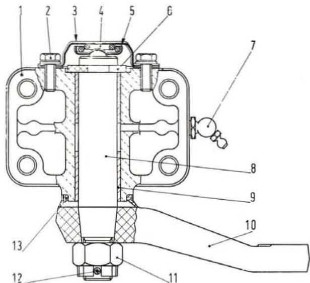
**Fig. 538 - Sectional view of idler arm and support assembly.**
