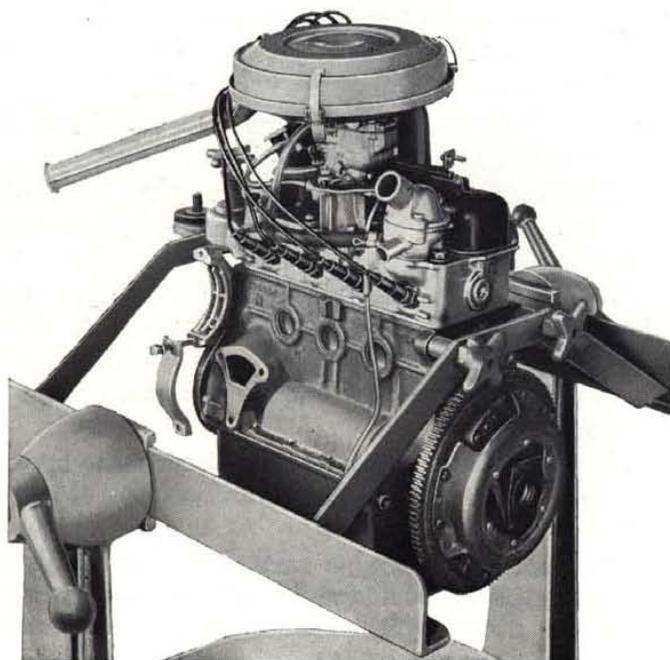
Fig. 11 - Engine on revolving stand Arr. 22204.
