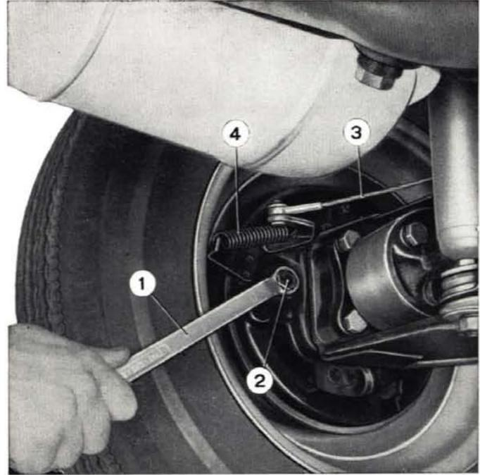
Fig. 298 - Adjusting brake shoe-to-drum clearance at rear wheels.
