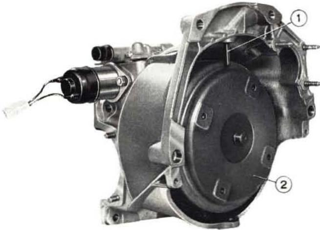
Fig. 575 - Transmission unit viewed from engine side.
