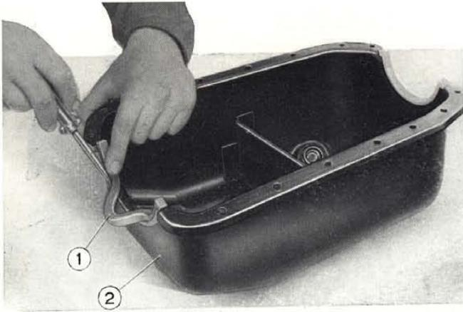
Fig. 23 - Fitting oil sump gasket.
