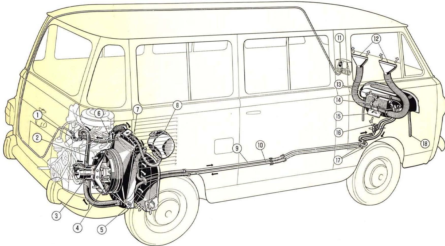
Fig. 546 - Engine cooling and car heating system.
