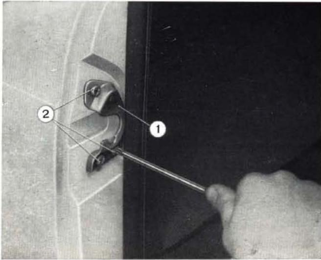
**Fig. 399 - Adjusting door lock striker plate.**
