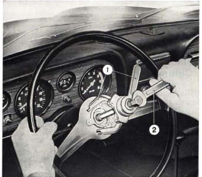
**Fig. 486 - Pulling the steering wheel.**
