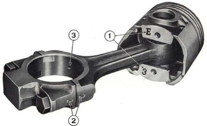
**Fig. 54 - Position of piston to connecting rod.**
