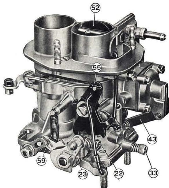
Fig. 432 - Carburetor viewed from the throttles control end.
