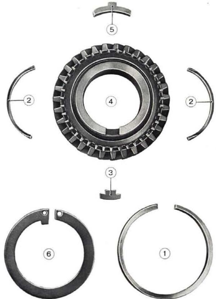
Fig. 167 - Third speed gear and synchronizer components.
