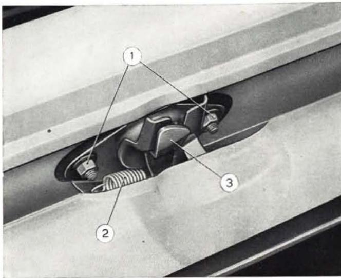
**Fig. 400 - Front compartment lid catch.**
