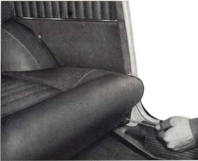
Fig. 474 - Removing rear seat cushion.
