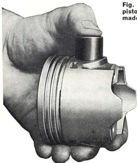
Fig. 44 - Insertion of piston pin should be made by sheer thumb pressure.
