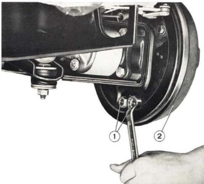
**Fig. 542 - Loosening lower anchor campin nuts.**
