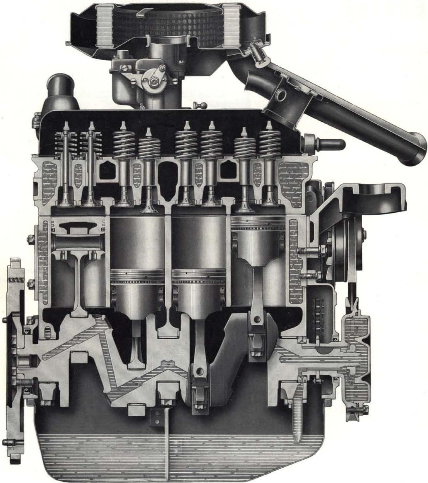
Fig. 6 - Side sectional view of engine across cylinders.
