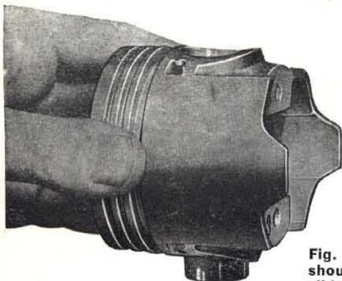
Fig. 45 - Piston pin should not be apt to slide away from boss.
