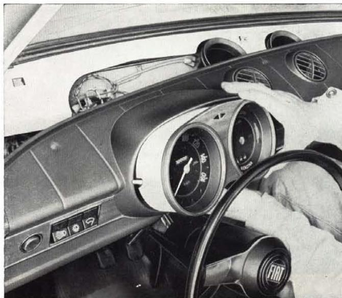
Fig. 471 - Withdrawing instrument cluster from panel lining.
