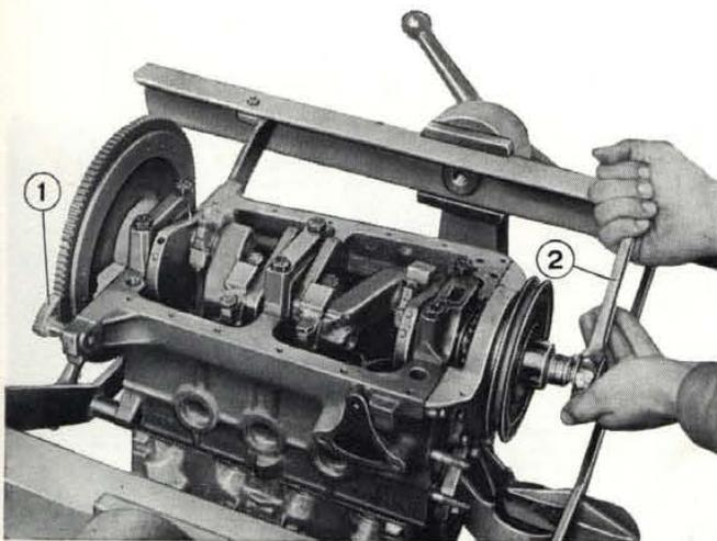
Fig. 13 - Backing out hub-pulley lock screw.
