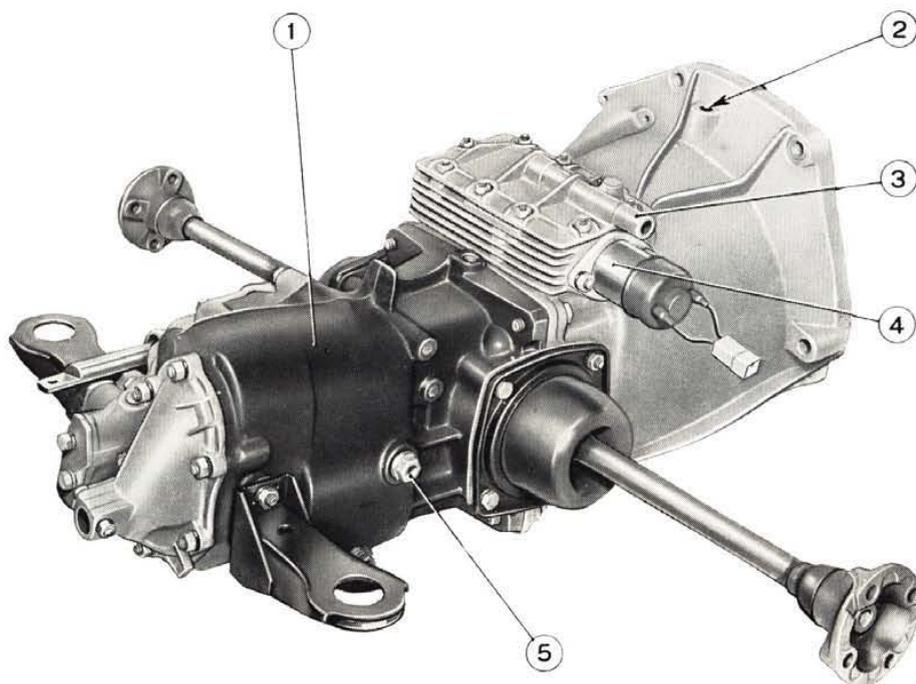
Fig. 561 - Transmission unit with hydraulic torque converter - left hand view.
