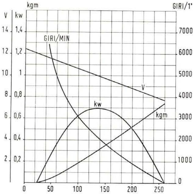
Fig. 344 - E 76-0,5/12 S Var. 9 starting motor curves.
