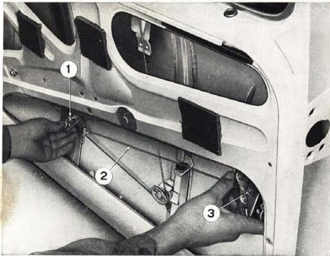
**Fig. 391 - Taking down door lock and control.**
