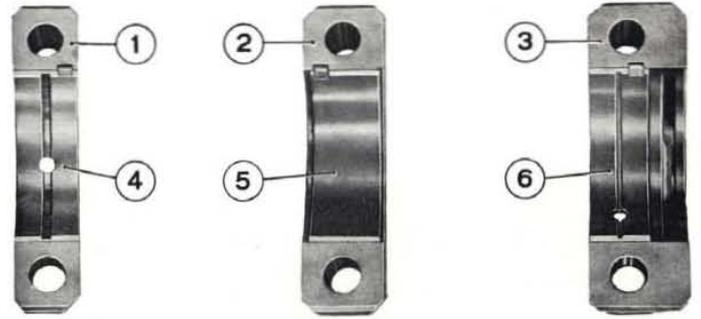
Fig. 74 - Main bearing caps with bearing inserts in place. 1. Front cap. - 2. Intermediate cap. - 3. Rear cap. - 4, 5, 6. Bearing inserts.
