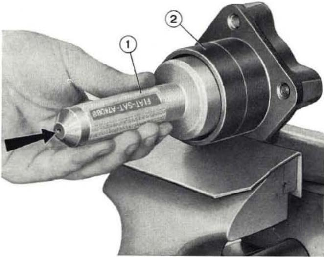
**Fig. 251 - Installing roller bearing cup.**
