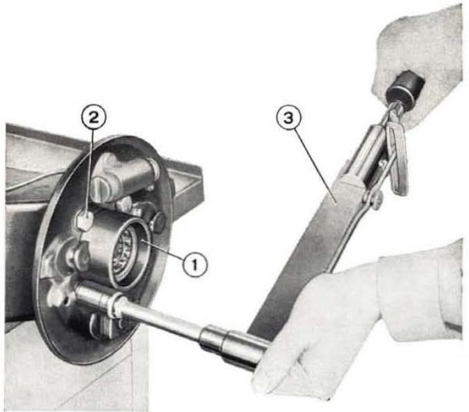
**Fig. 253 - Securing rear wheel hub and brake backing plate to control arm.**
