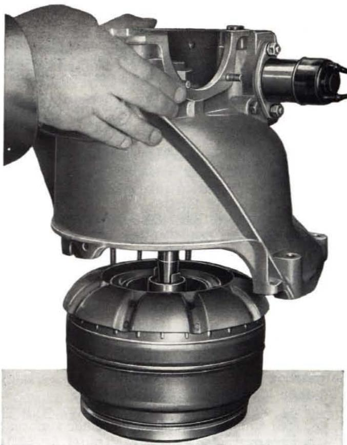
Fig. 591 - Fitting Idroconvert transmission casing onto torque converter.
