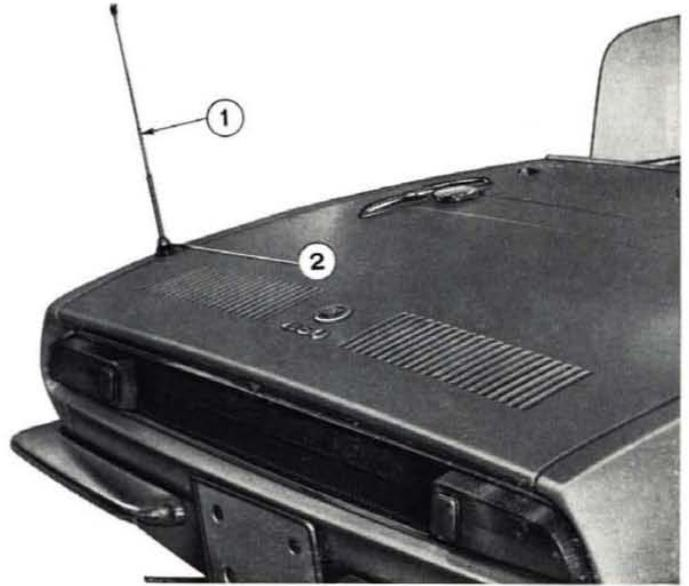
Fig. 504 - Antenna installed on rear fender.
