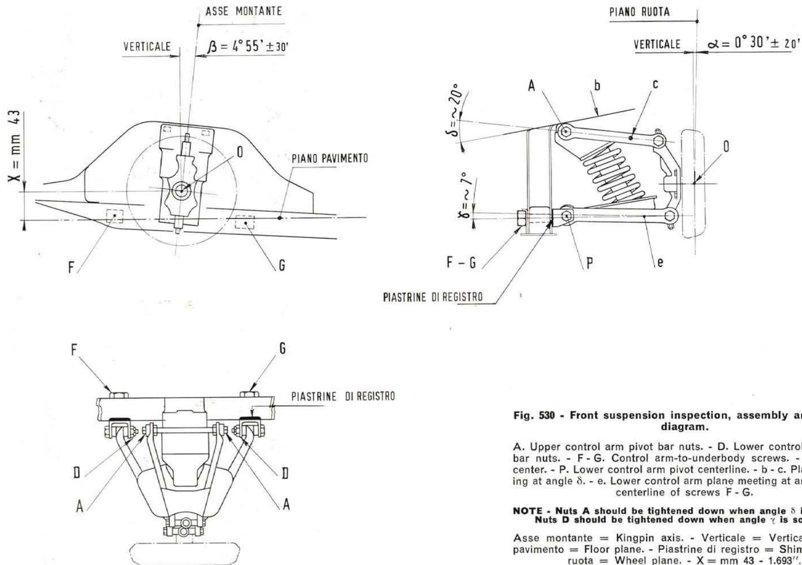
**Fig. 530 - Front suspension inspection, assembly and setting diagram.**
