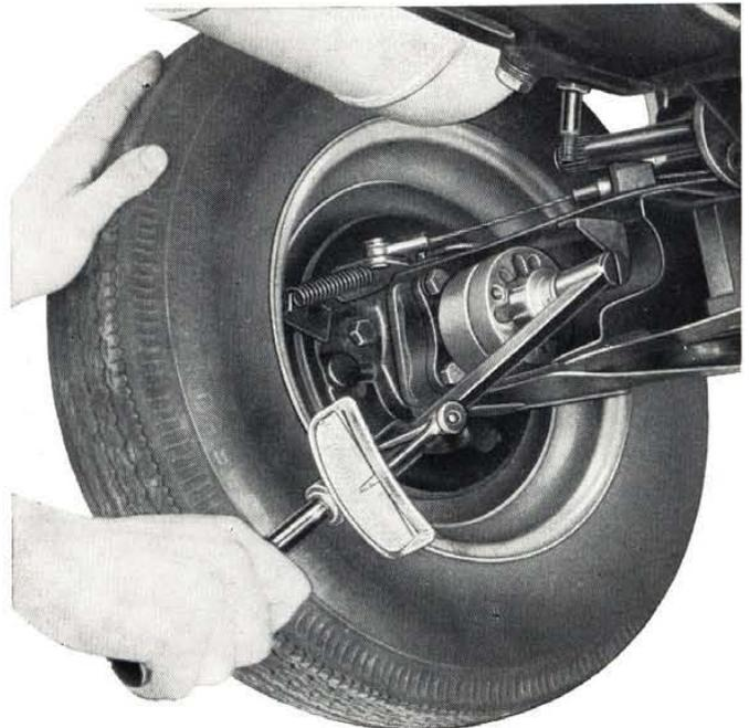
Fig. 261 - Tightening flexible joint mounting nut.
