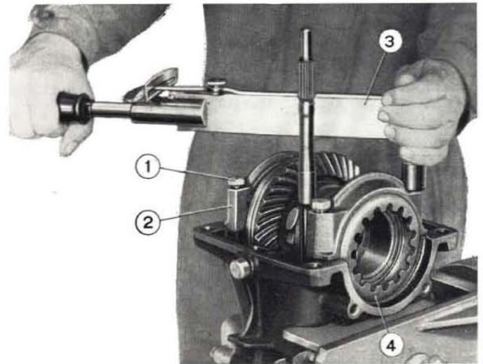
Fig. 189 - Tightening differential carrier cap screws.
