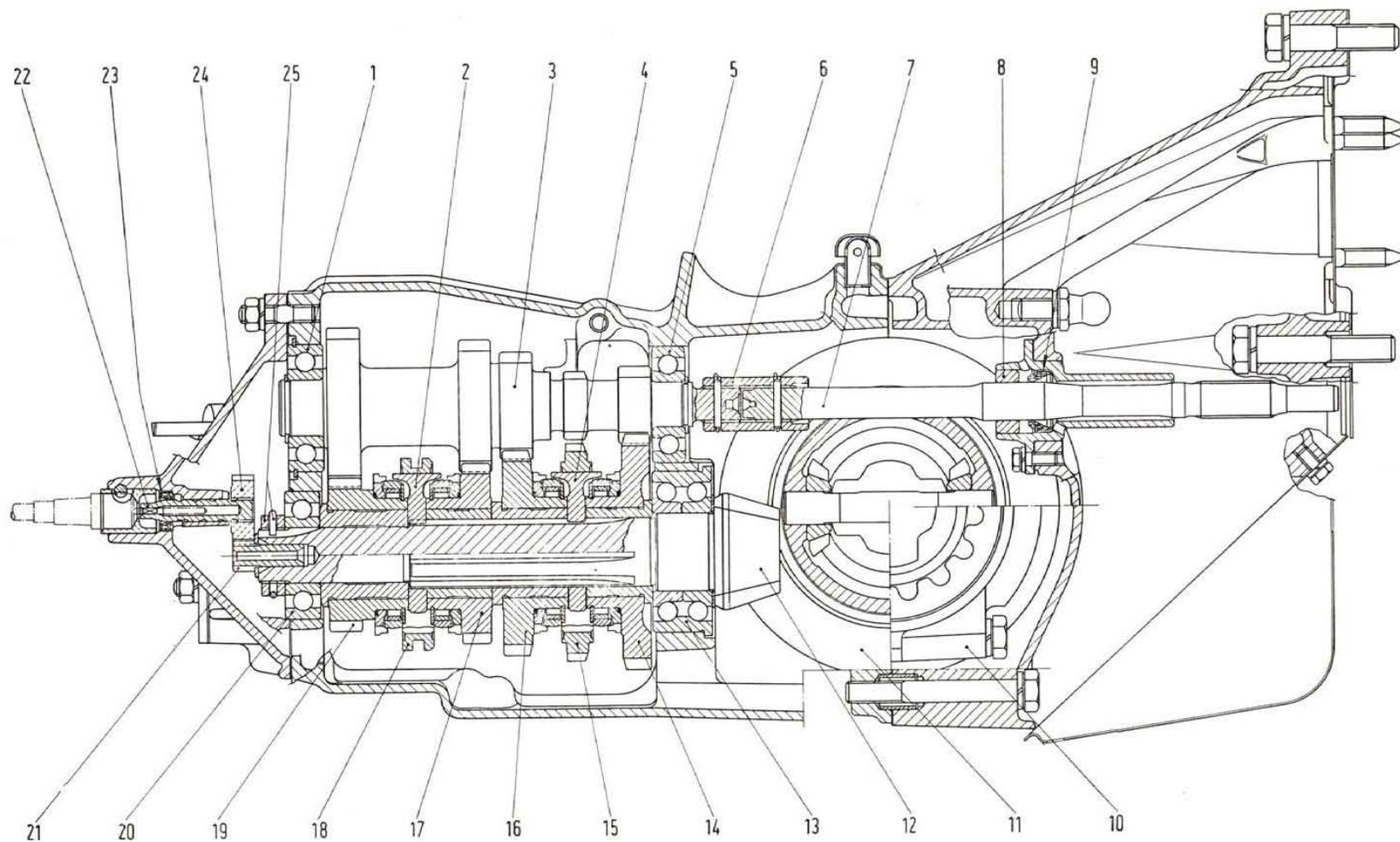
**Fig. 171 - Side sectional view of transmission-differential assembly.**
