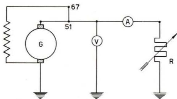
Fig. 320 - Wiring diagram for plotting the ampere-revolution output curve at a steady 12 V voltage (68° F - 20° C).
