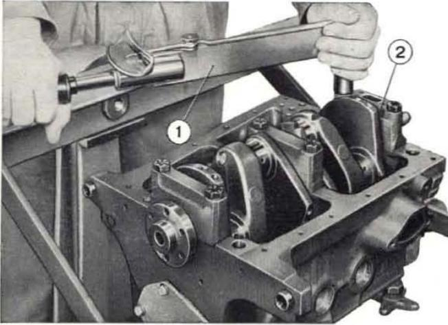
Fig. 79 - Tightening main bearing cap screws.
