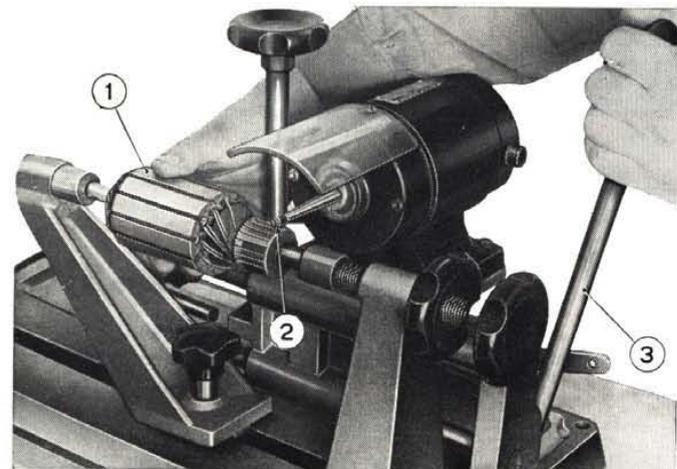
Fig. 323 - Undercutting mica between commutator bars using fixture Ap. 5015.
