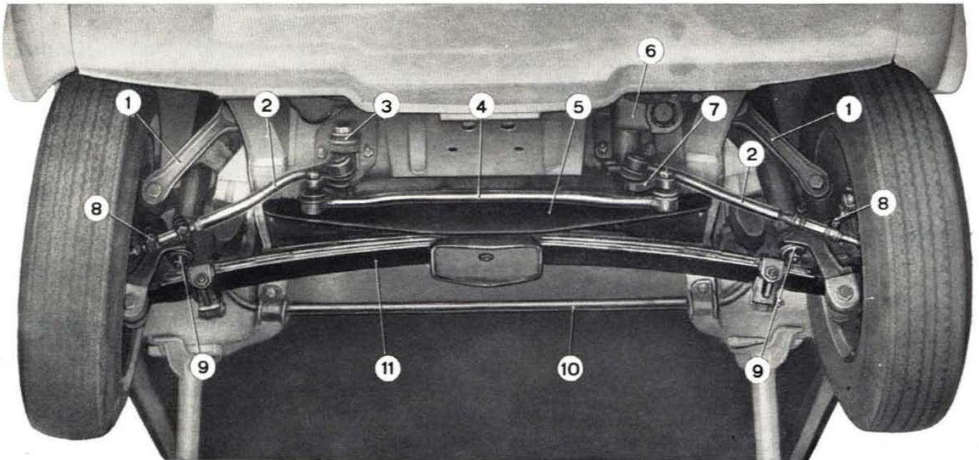
**Fig. 217 - Front suspension assembly in place on car.**
