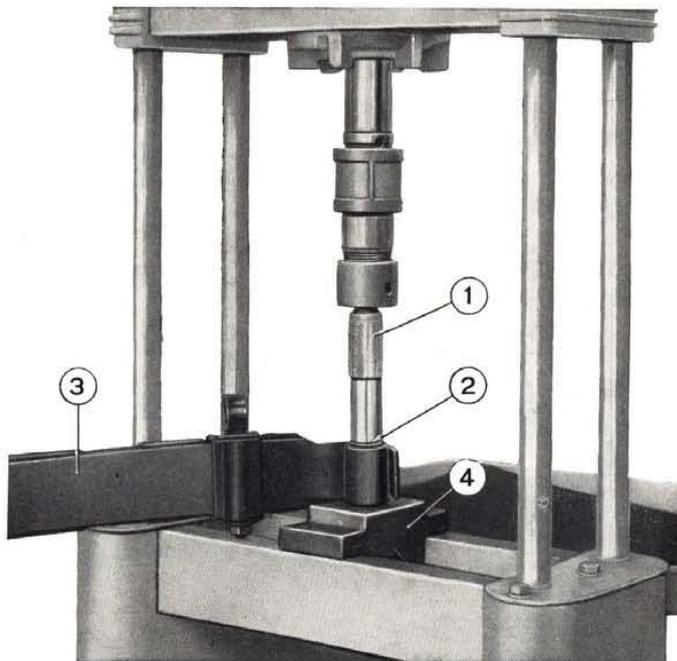
Fig. 216 - Press fitting resilient bushing into semi-elliptic spring end eye.
