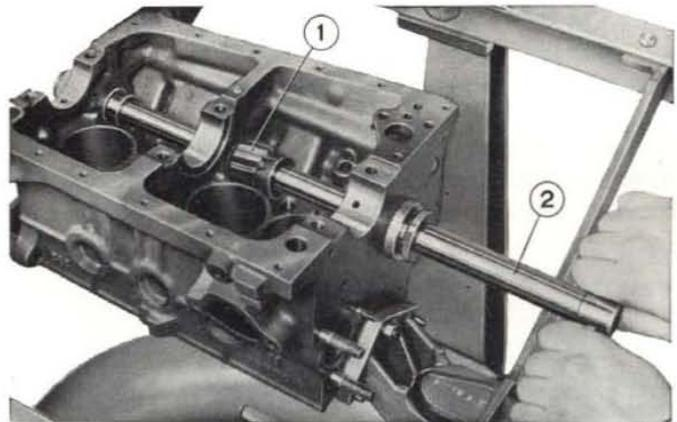
**Fig. 115 - Reaming intermediate camshaft bushing.**
