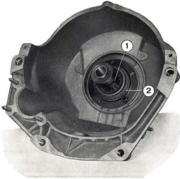
**Fig. 579 - Centralising the oil pump.**
