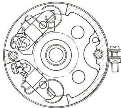
Fig. 341 - End section view across commutator end head and view of brushes.
