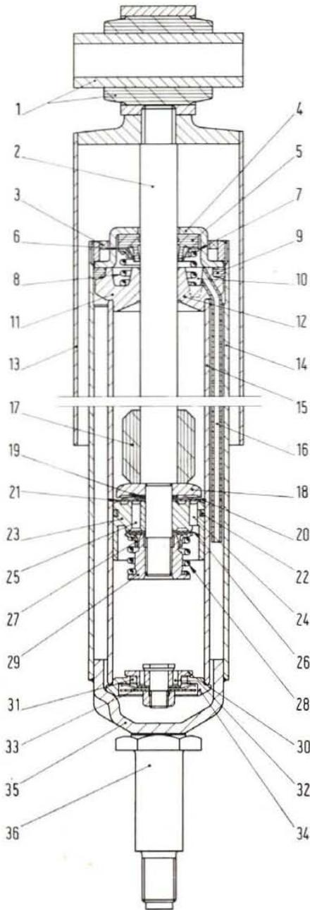
**Fig. 268 - Sectional view of shock absorber.**
