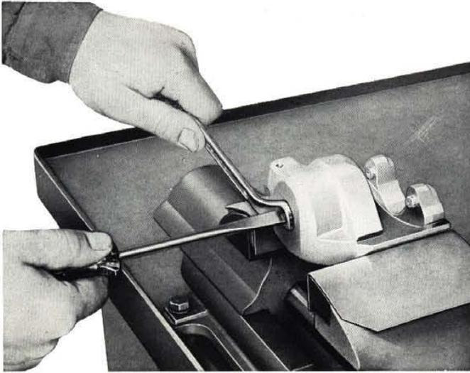
Fig. 455 - Removing brake caliper self-adjusting pin nut.
