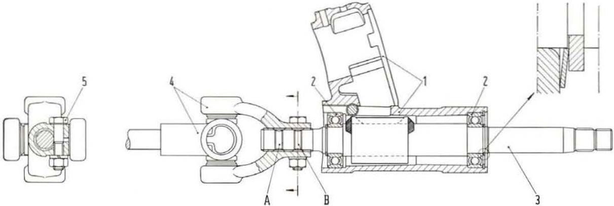
**Fig. 485 - Section view of the steering column and mounting bracket.**
