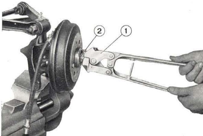
Fig. 229 - Staking steering knuckle nut.
