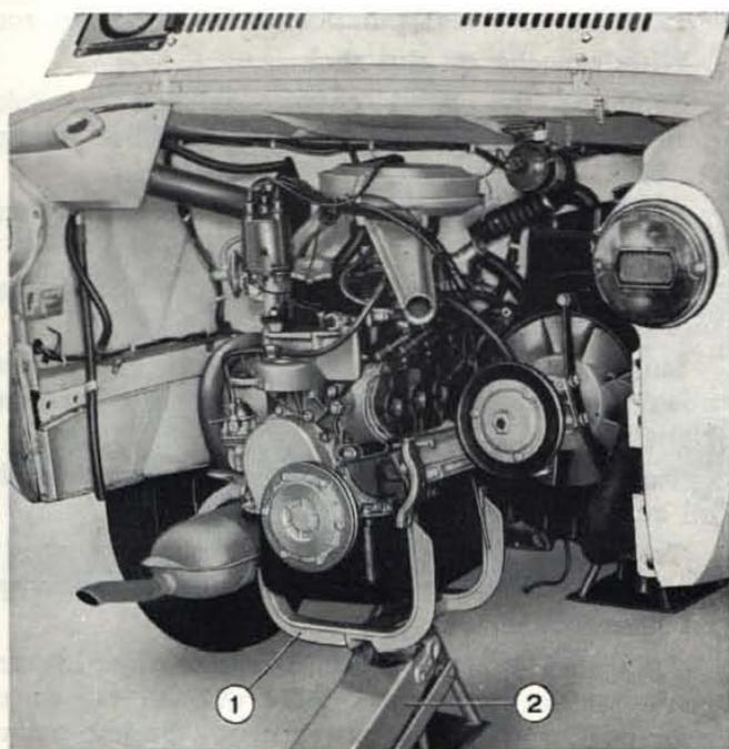
**Fig. 8 - Removing engine.**
