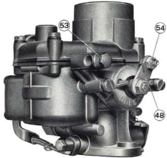
Fig. 148 - Solex carburetor viewed from choke end.
