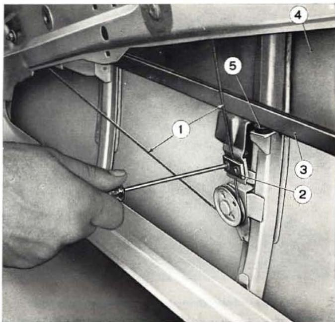
**Fig. 395 - Adjusting drop glass travel.**
