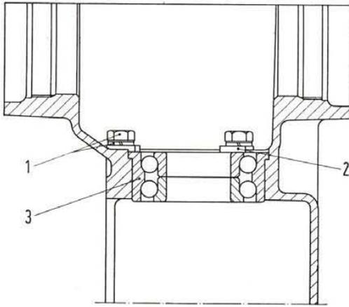
**Fig. 193 - Placing drive pinion rear bearing into transmission-differential case.**
