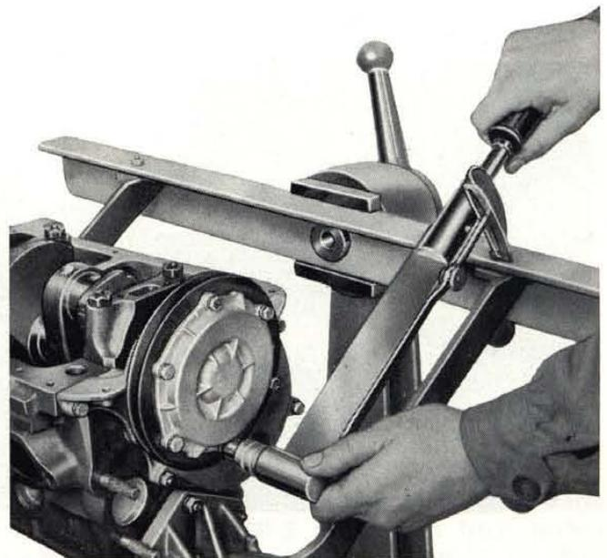
**Fig. 22 - Tightening centrifugal oil filter cover.**
