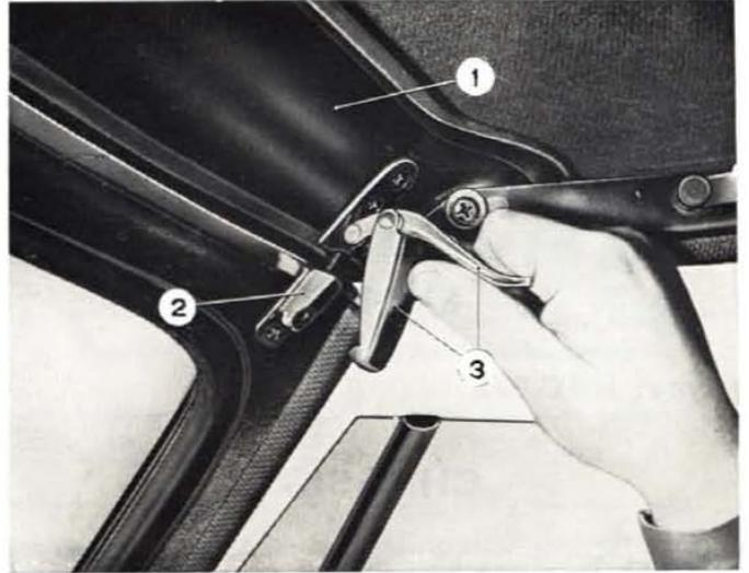
**Fig. 518 - Fastening top at front.**
