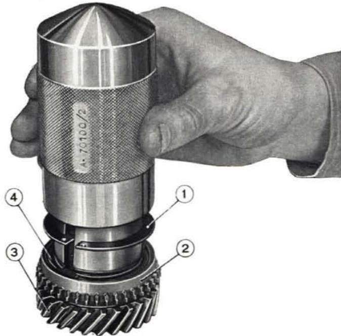
Fig. 169 - Using tool A. 70100/2 to install the synchronizer snap ring.
