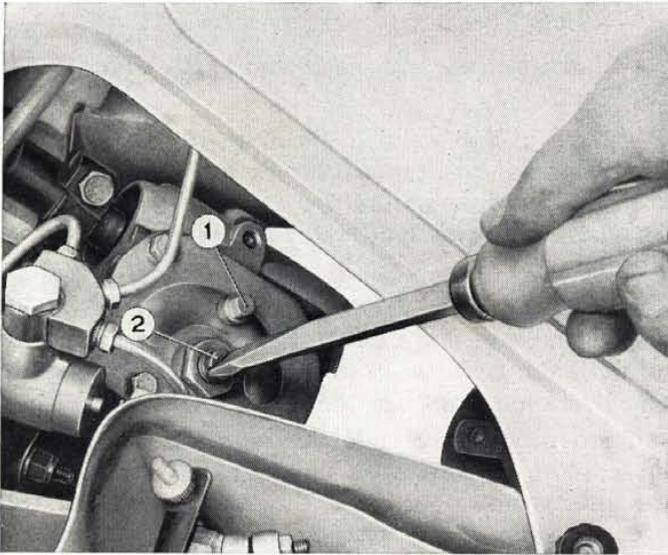
Fig. 279 - Adjusting lash between worm and sector.
