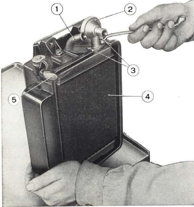
**Fig. 310 - Removing heater radiator cock.**
