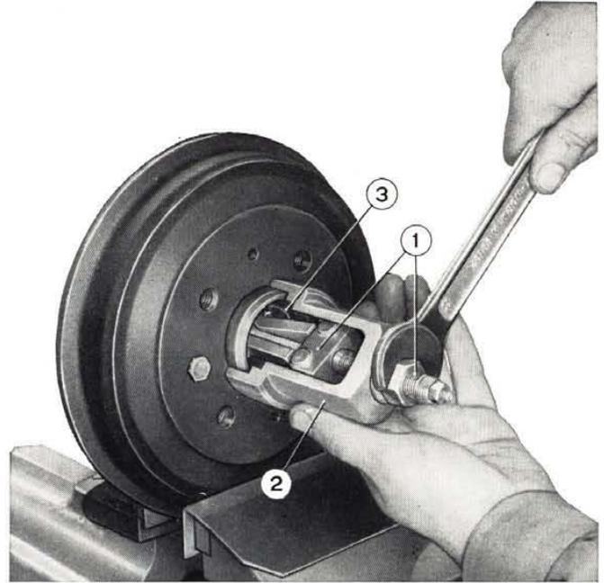
**Fig. 222 - Pulling outer bearing cup.**
