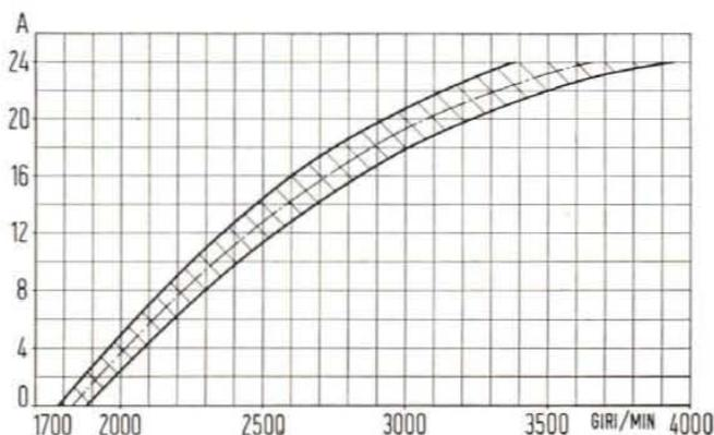
Fig. 321 - Output curve of warm D 90/12/16/3 CS generator.
