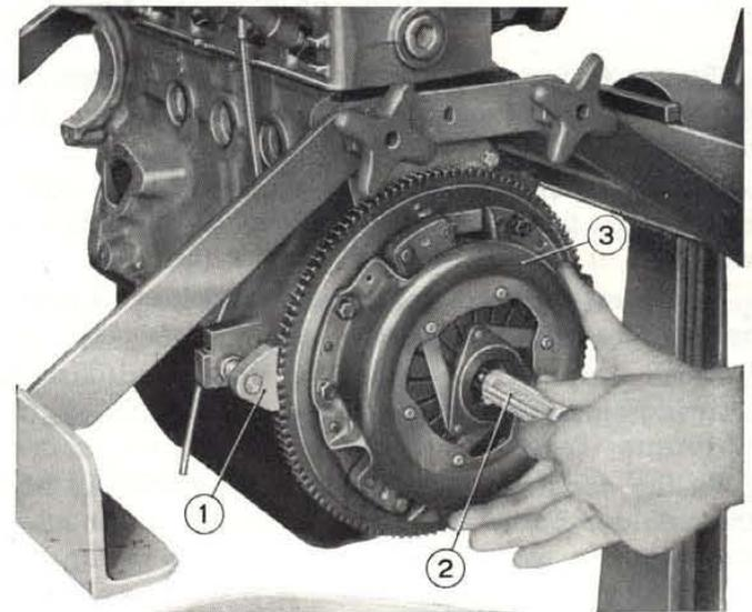
Fig. 25 - Installing clutch assembly.
