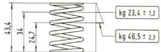
Fig. 105 - Valve spring specifications.
