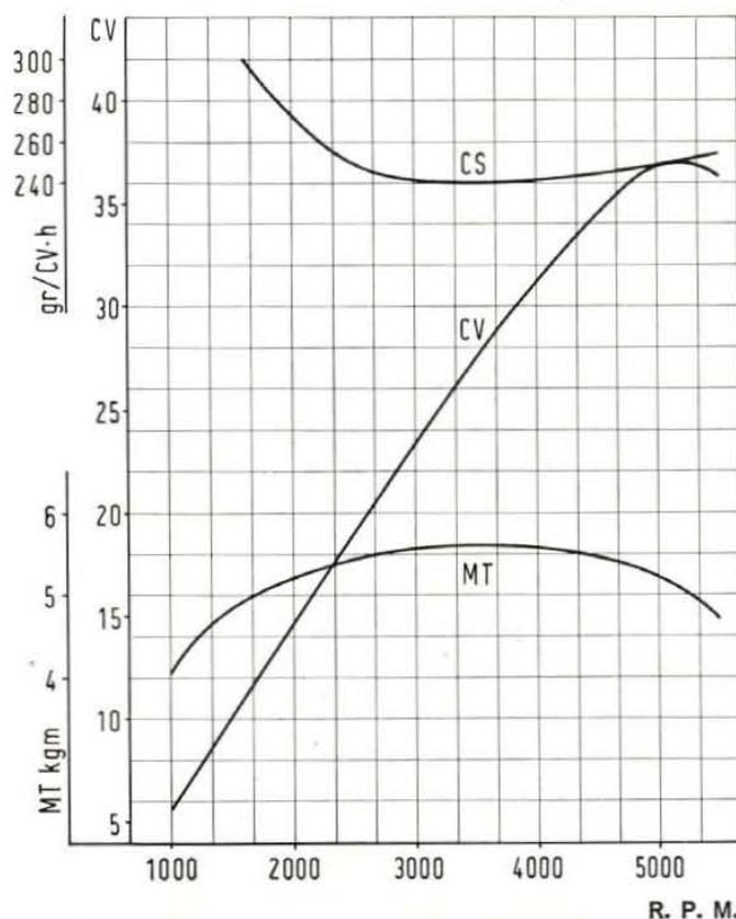
Fig. 123 - Horsepower, consumption and torque curves of 100G.002 engine.
