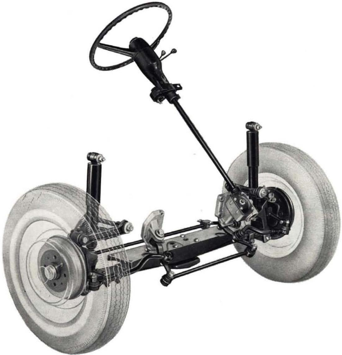
Fig. 270 - Steering system and front running gear units.
