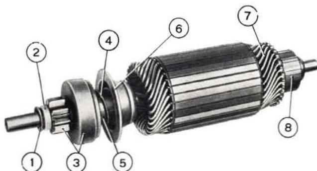
Fig. 347 - Armature assembly with overrunning clutch drive mechanism.
