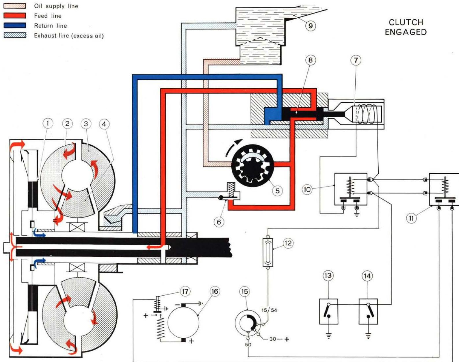
Fig. 566 - Operating diagram of Hidroconvert transmission with clutch engaged.
