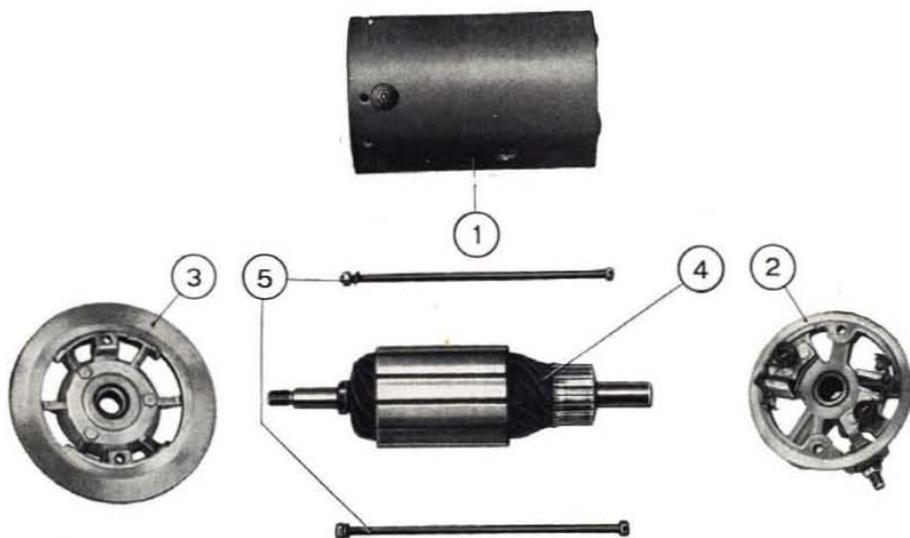
Fig. 326 - Components of D 90/12/16/3 CS generator.
