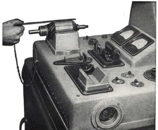
Fig. 325 - Testing the armature on bench, using a lamina. In correspondence with short-circuited coils the lamina will vibrate.
