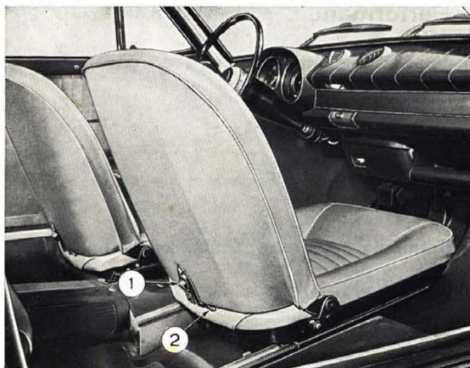
Fig. 420 - Detail of front seat back rest catch.
