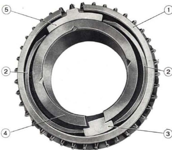
Fig. 166 - Third speed gear synchronizer in place in gear.
