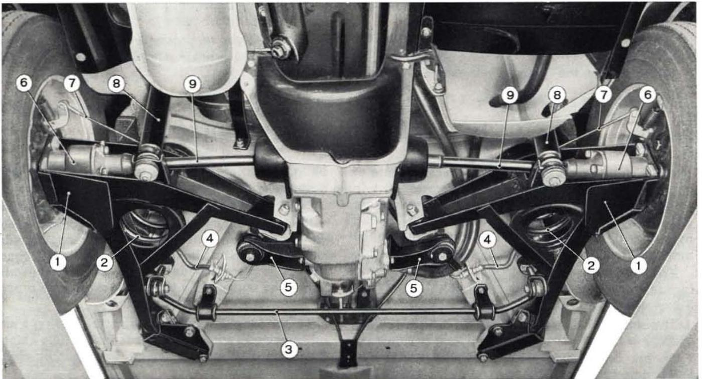
Fig. 265 - Rear suspension assembly in place on car.
