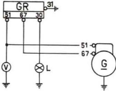
Fig. 329 - Wiring diagram for checking the cutout closing voltage.
