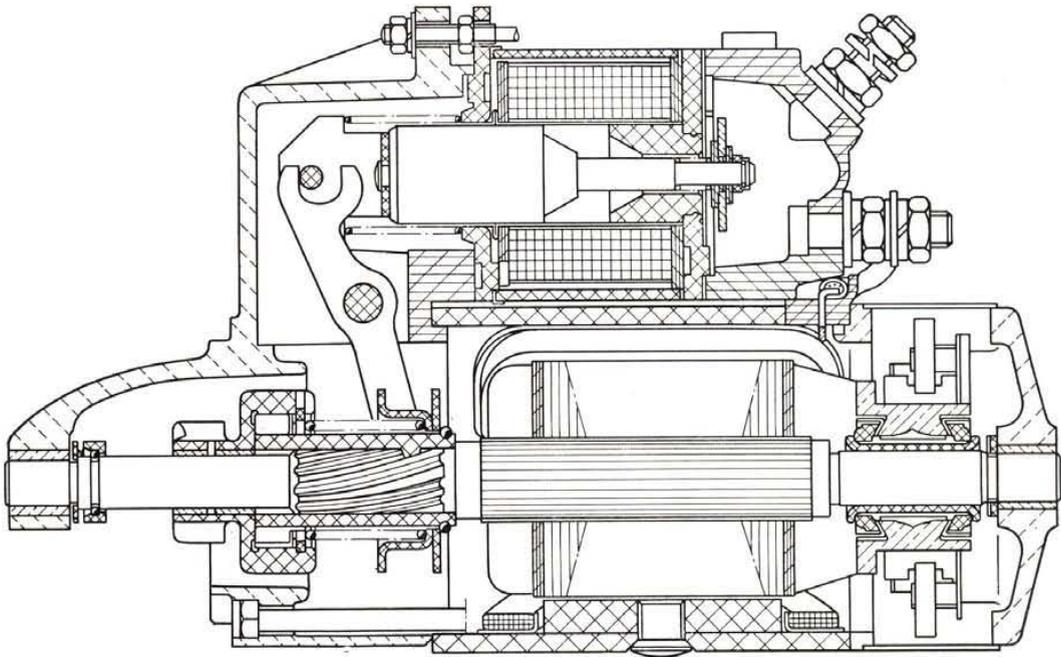
Fig. 339 - Side section view of starting motor.
