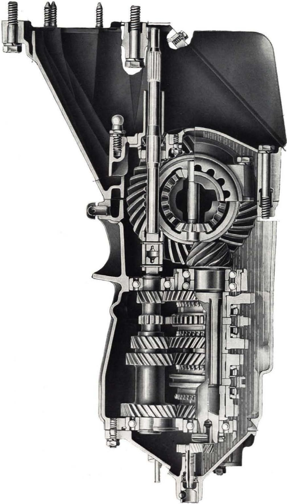
Fig. 163 - Side sectional view of transmission-differential assembly.
