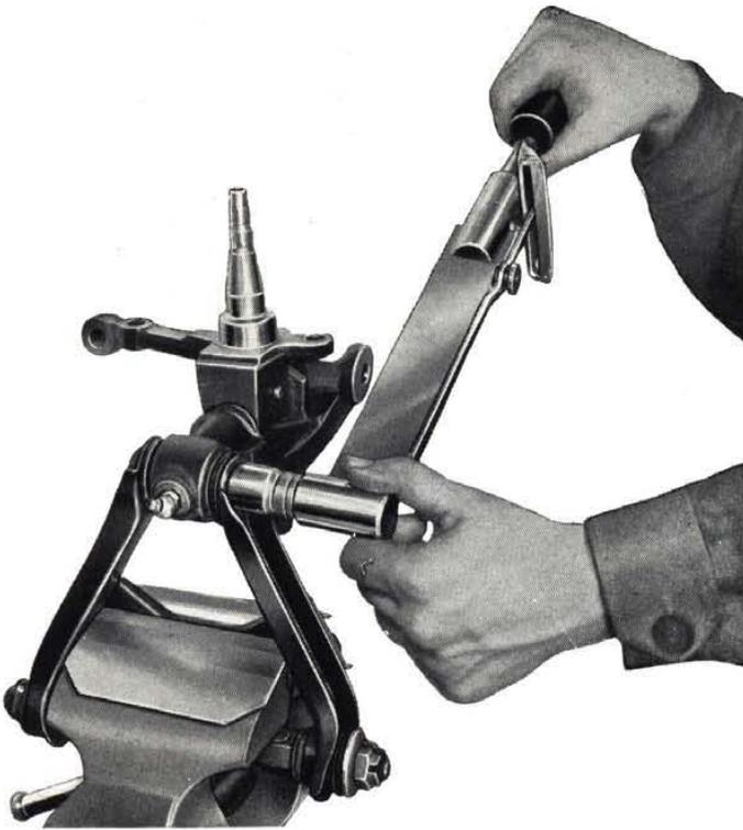
Fig. 228 - Using torque wrench to secure upper control arm to kingpin housing.
