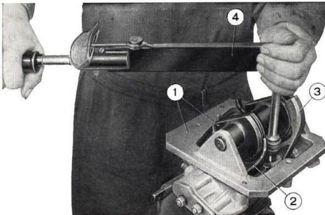
**Fig. 184 - Tightening shifter forks.**
