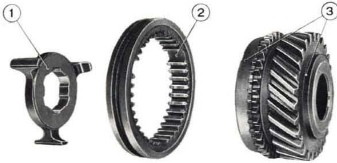
Fig. 165 - Transmission synchronesh gears.
