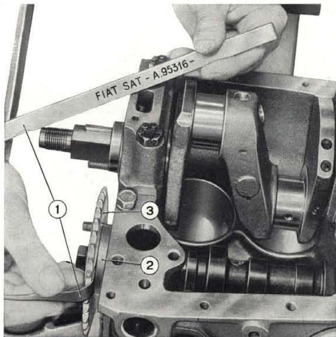
Fig. 18 - Checking driven sprocket-to-camshaft spacer clearance.
