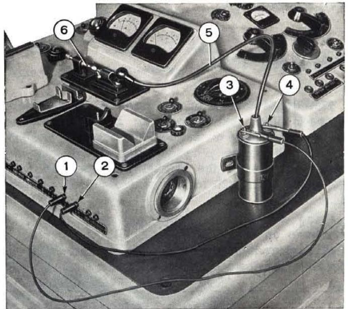
Fig. 354 - Checking ignition coil on test bench.
