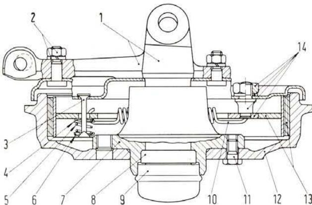
Fig. 290 - Sectional view of left side front wheel. (Up to car with No. for spare 802091).
