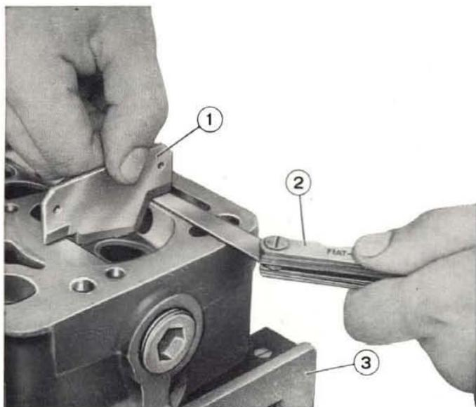
Fig. 89 - Checking depth of combustion chambers.
