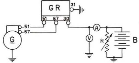
Fig. 331 - Wiring diagram for checking the current and voltage regulators.
