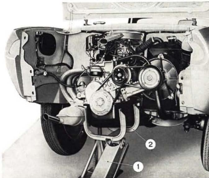
Fig. 484 - Engine removal.
