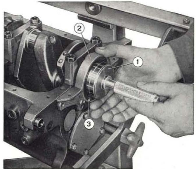
Fig. 81 - Installing crankshaft front seal cover.
