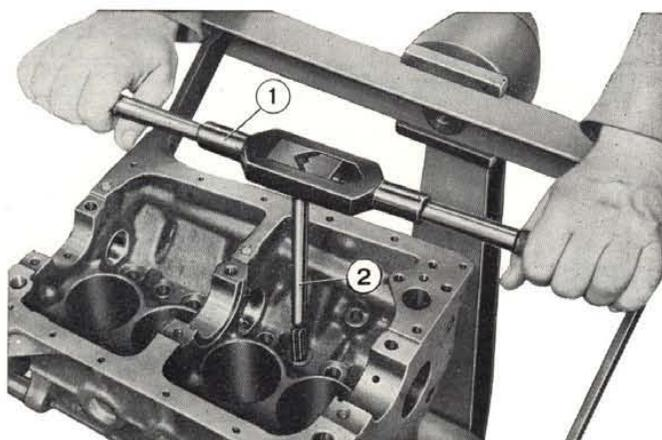
Fig. 116 - Reaming tappet seats in crankcase.
