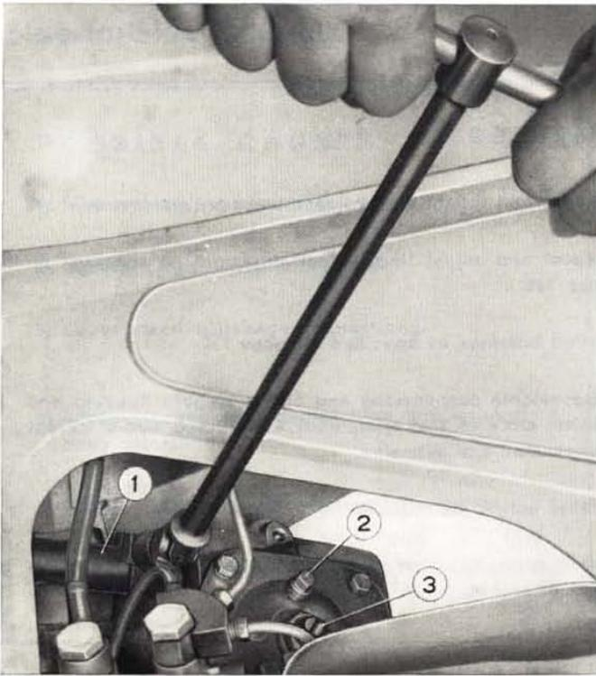
**Fig. 273 - Removing steering gear.**
