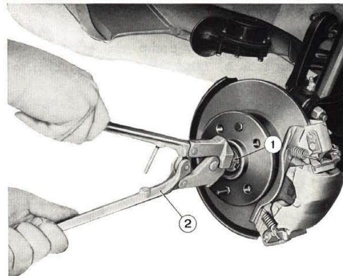
Fig. 458 - Staking wheel hub nut.
