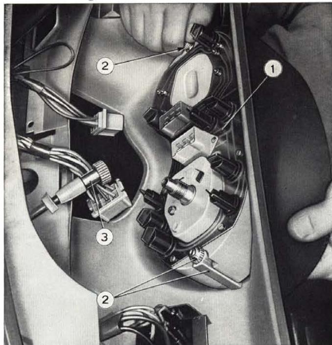
Fig. 469 - Removing instrument cluster.
