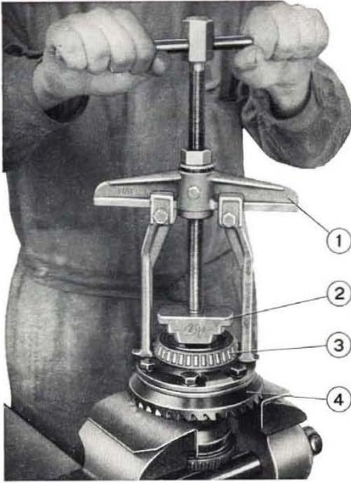
Fig. 187 - Pulling differential cage roller bearing cones.
