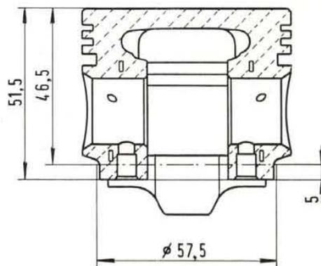
Fig. 46 - Milling diagram of piston to equalize the set weight.
