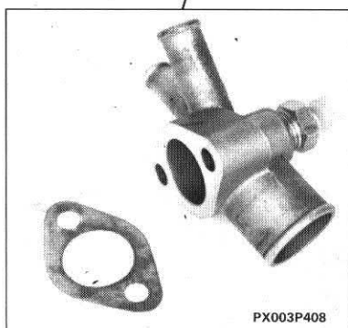
Cylinder head fitting for coolant line attachment complete with temperature transmitter
