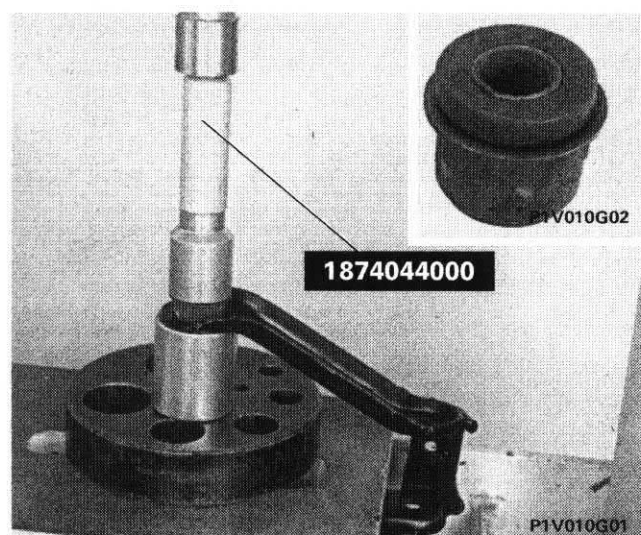
Fitting flexible bushes and pin for track control arm
